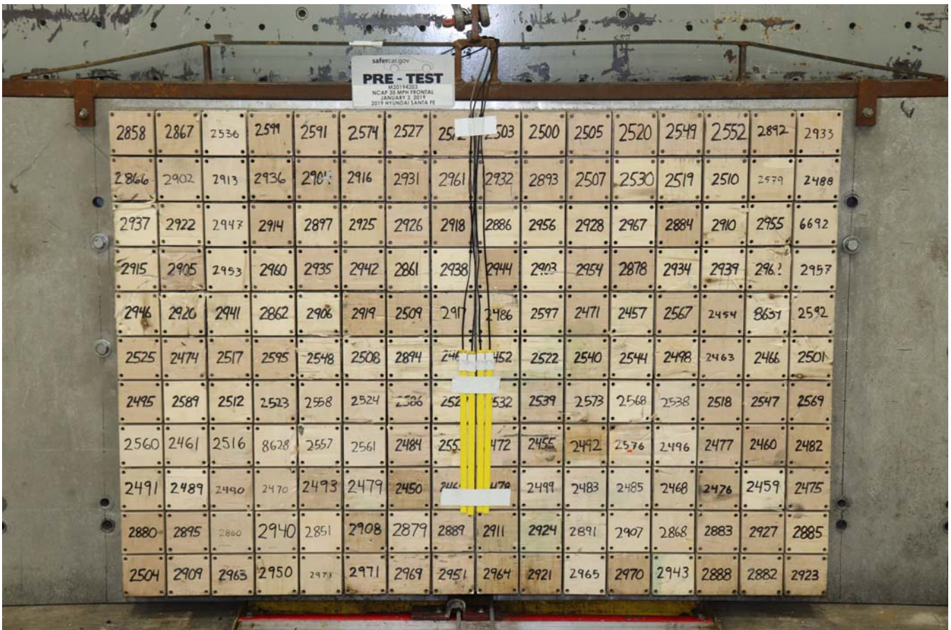
Photo No. 002 - Pre-Test Load Cell Wall
