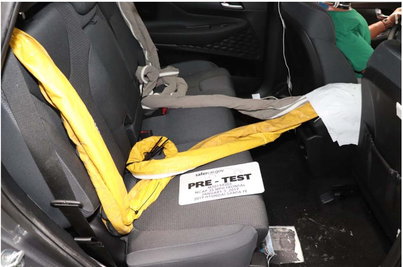
Photo No. 028 - Pre-Test Dummy Cable Routing
