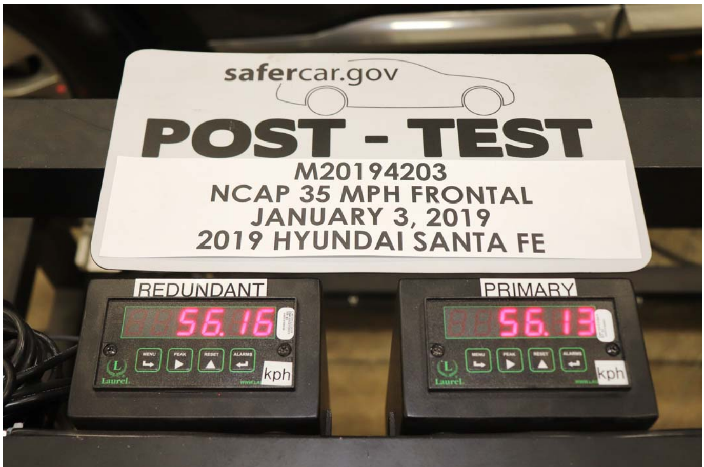
Photo No. 072 - Post-Test Speed Trap Read-Out
