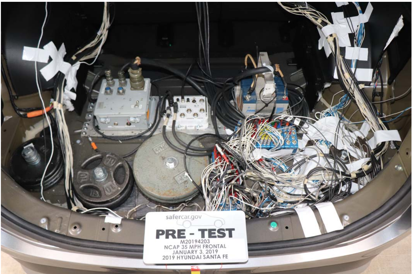
Photo No. 070 - Ballast Installed in Vehicle
