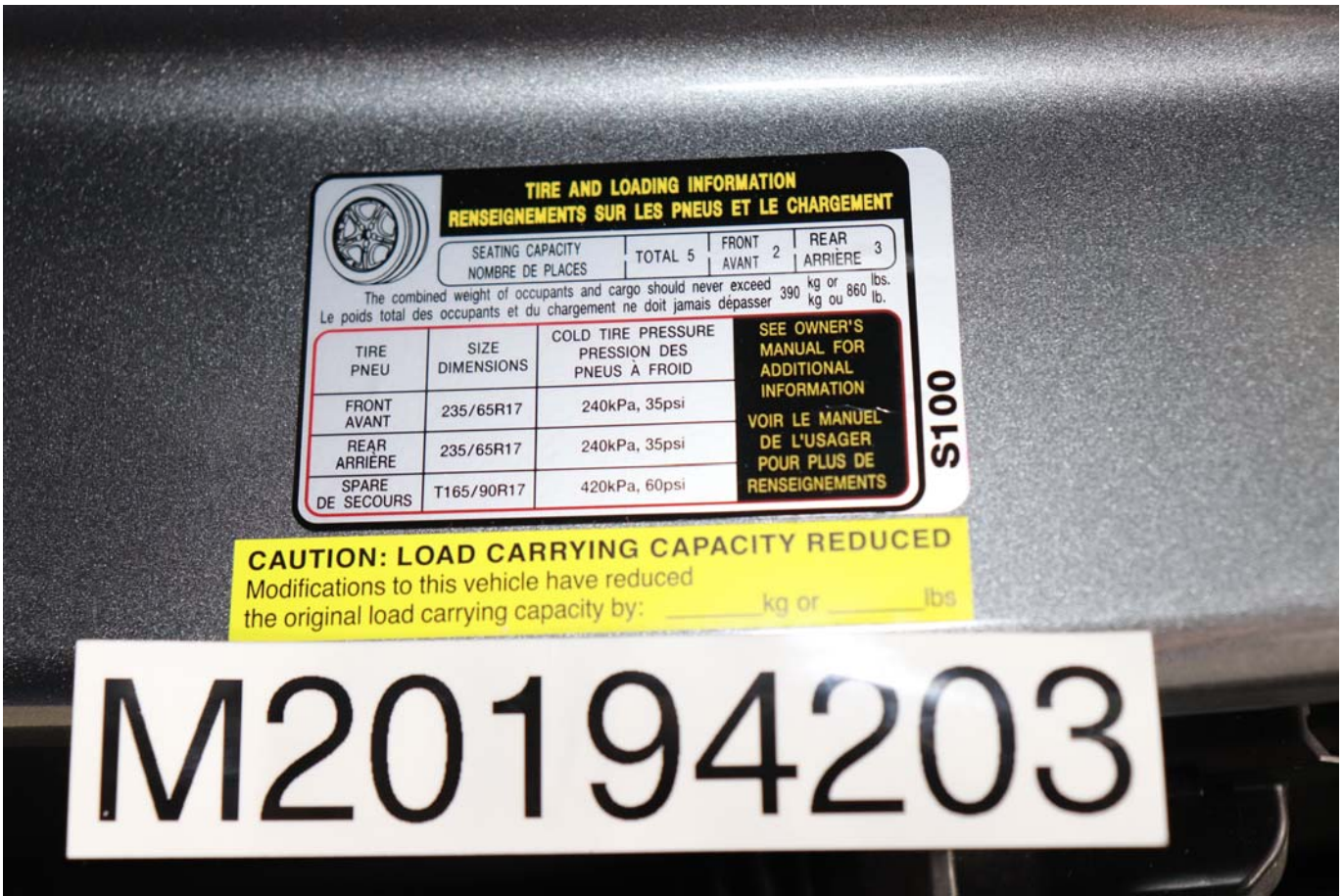
Photo No. 005 - Tire Placard Vehicle Capacity Weight updated by manufacturer from 390 kg to 480 kg.
