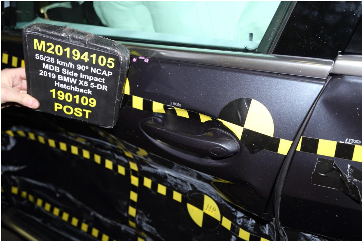
022 Post-Test Left Front Door Latch Close-Up
