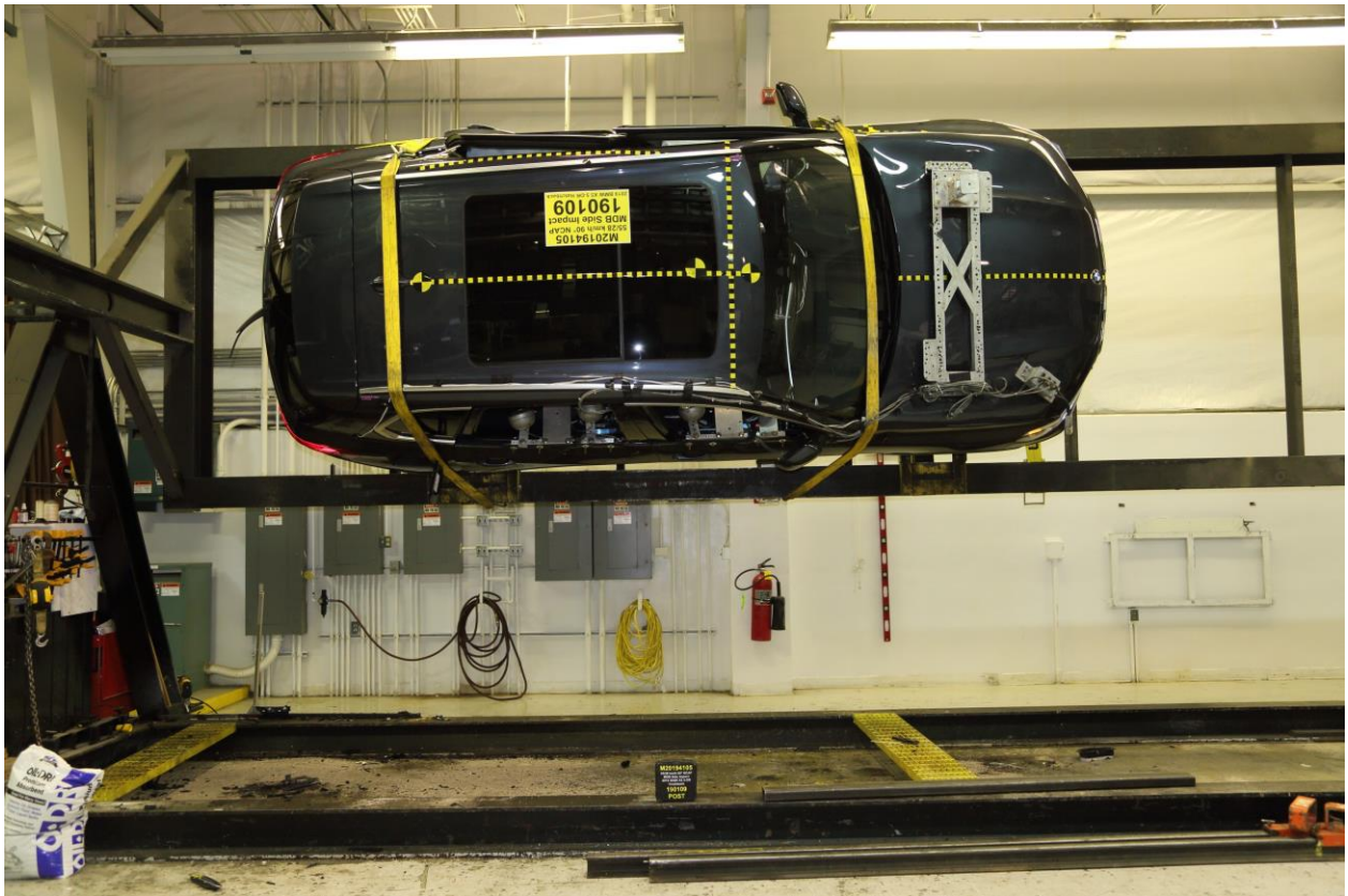
097 FMVSS No. 301 Static Rollover 90 Degrees
