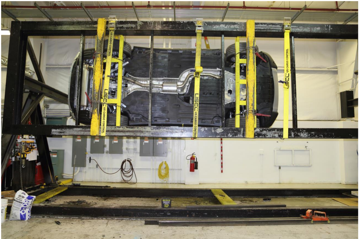
099 FMVSS No. 301 Static Rollover 270 Degrees
