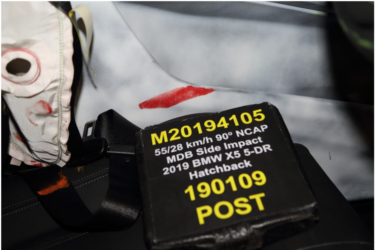
052 Post-Test Driver Dummy Close-Up Pelvis Contact View
