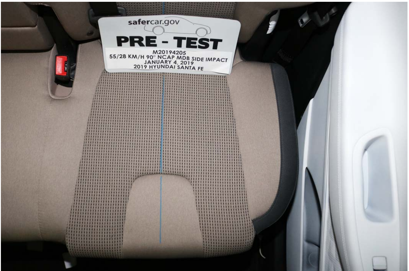
Photo No. 060 - Pre-Test Overhead View of Rear Passenger Seat Pan Prior to Dummy Positioning
