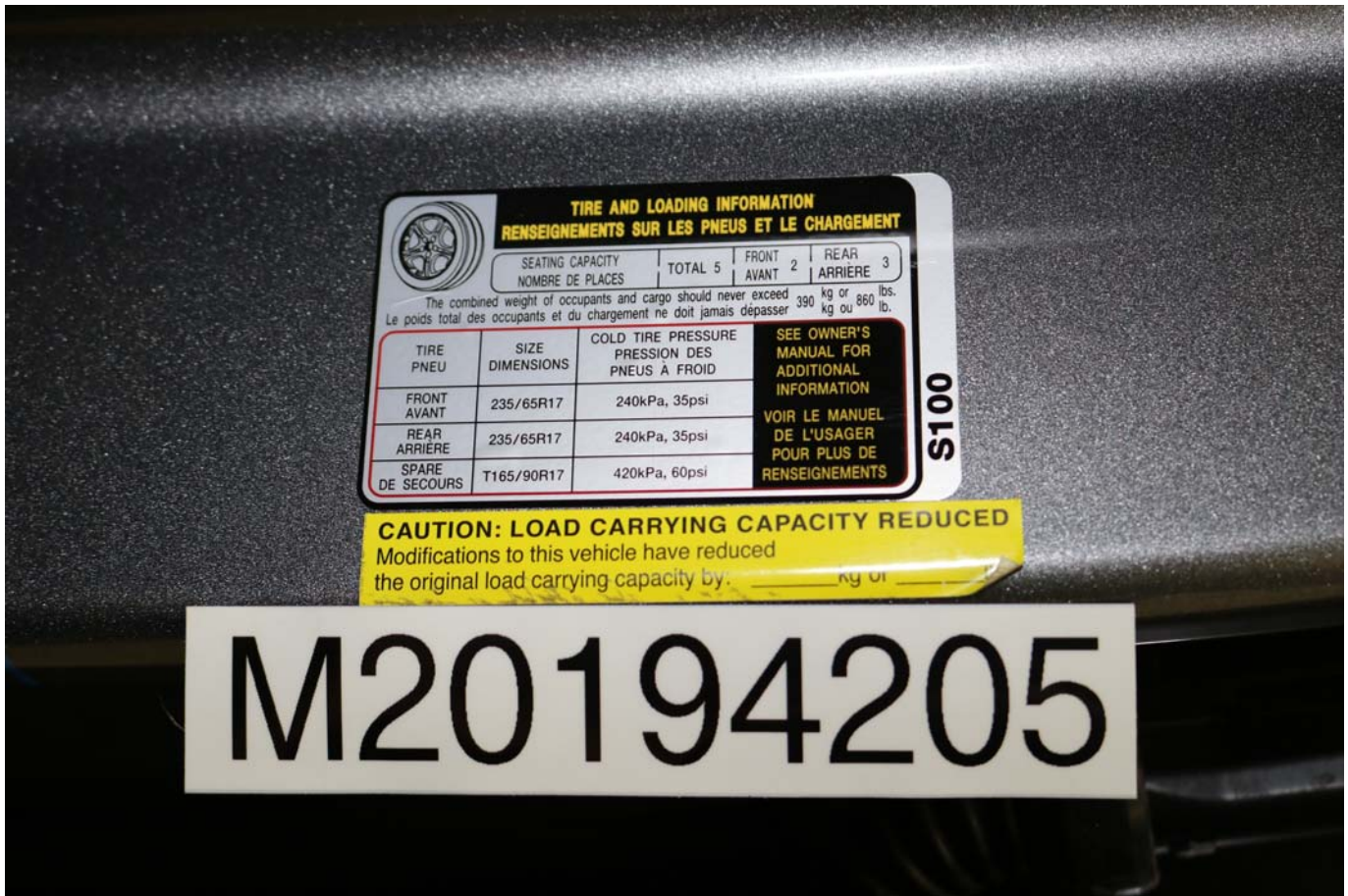
Photo No. 093 - Close-Up View of Vehicle Tire Information Placard or Label * Vehicle Capacity Weight updated by manufacturer from 390kg to 480kg.
