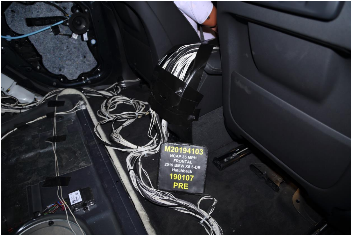
028 Pre-Test Dummy Cable Routing
