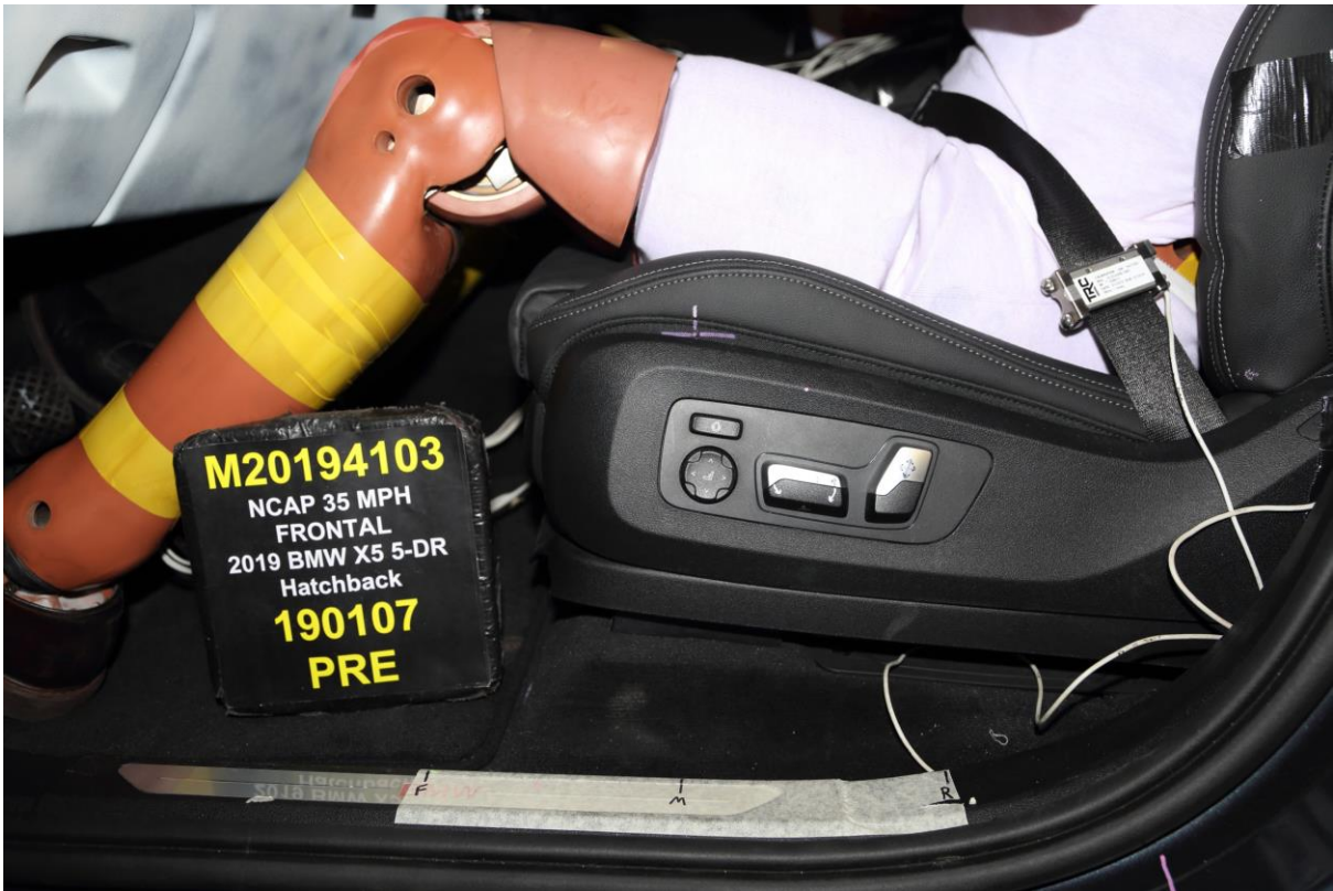
036 Pre-Test Driver's Seat Fore-Aft Markings
