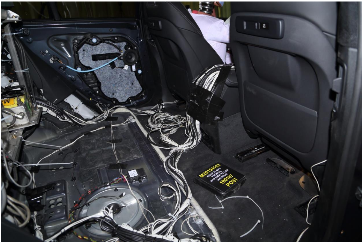
029 Post-Test Dummy Cable Routing
