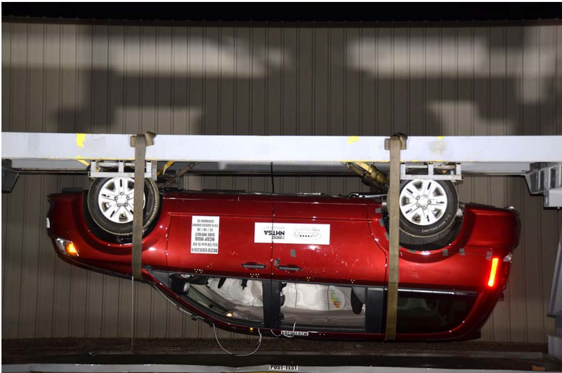
FIGURE 98. FMVSS No. 301 Static Rollover 180 Degrees
