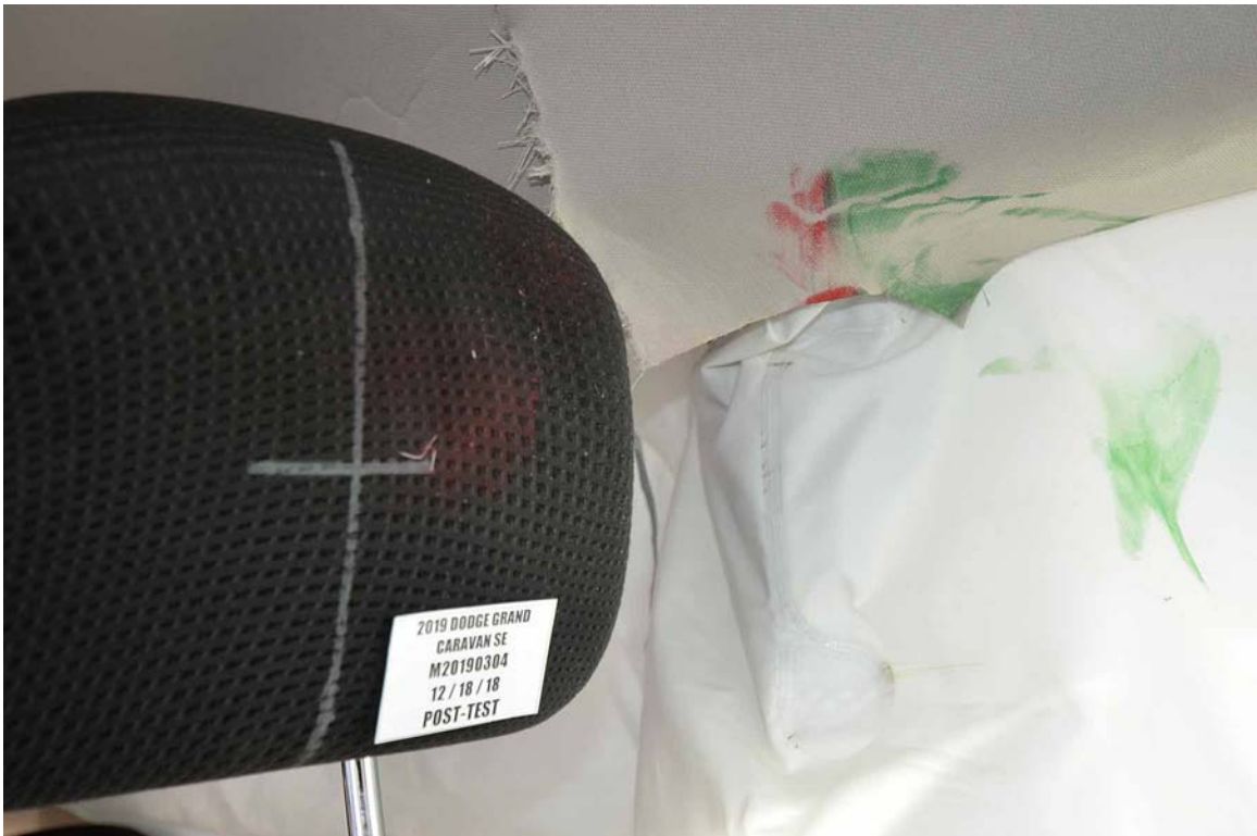
FIGURE 48. Post-Test Driver Dummy Close-Up Head Contact with Vehicle Interior View
