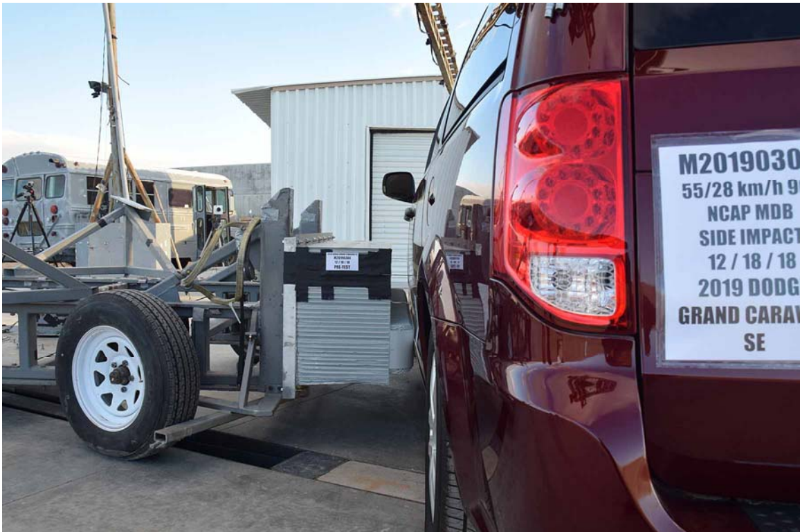
FIGURE 18. Pre-Test Right Side View of MDB Positioned Against Side of Test Vehicle
