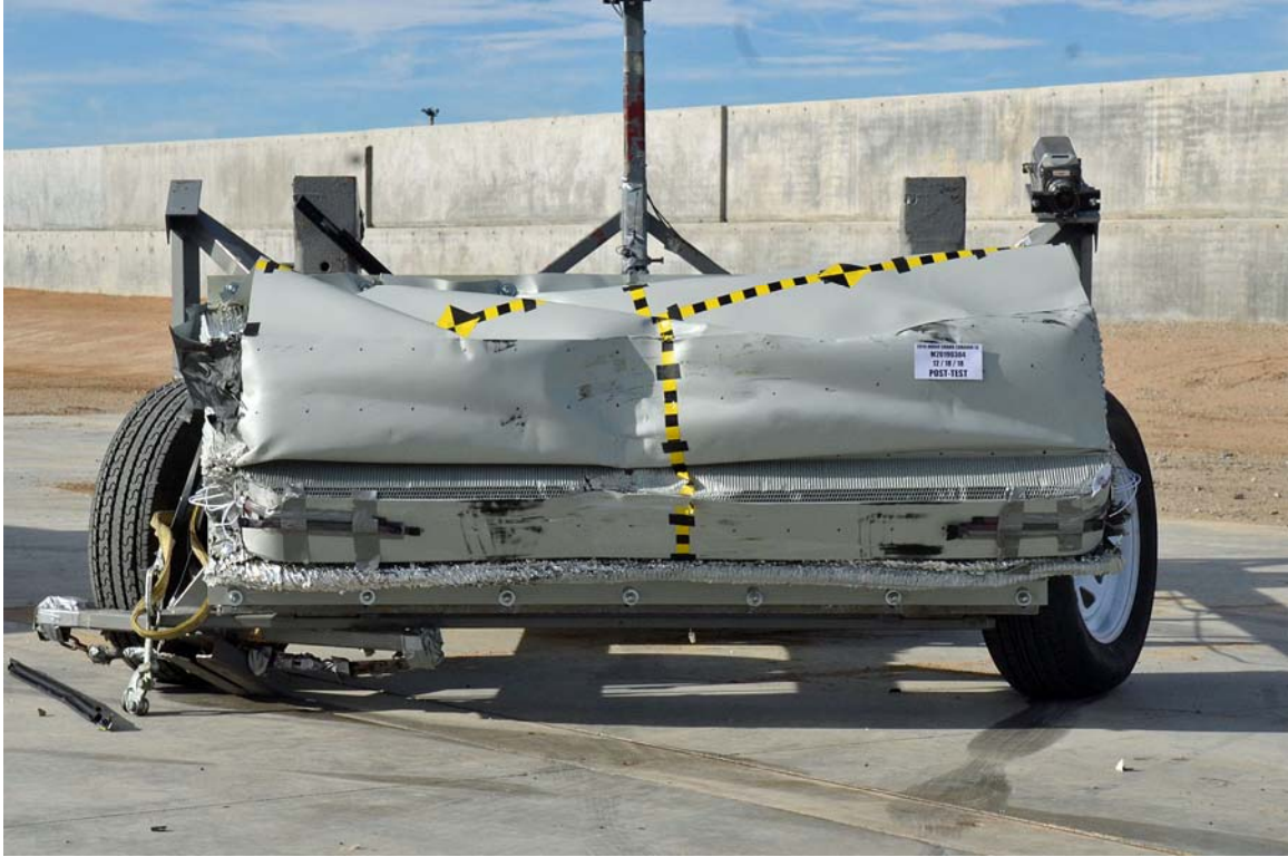
FIGURE 85. Post-Test Front View of MDB Impactor Face
