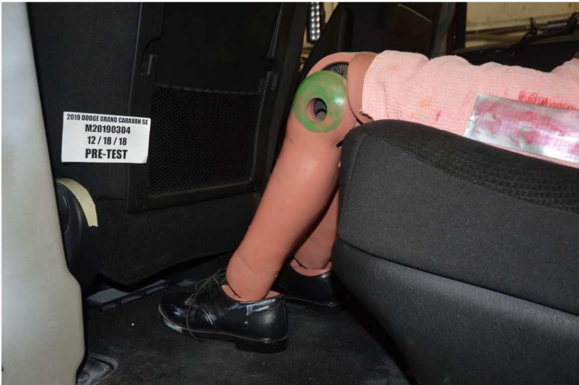
FIGURE 64. Pre-Test Placement of Rear Passenger Dummy's Feet
