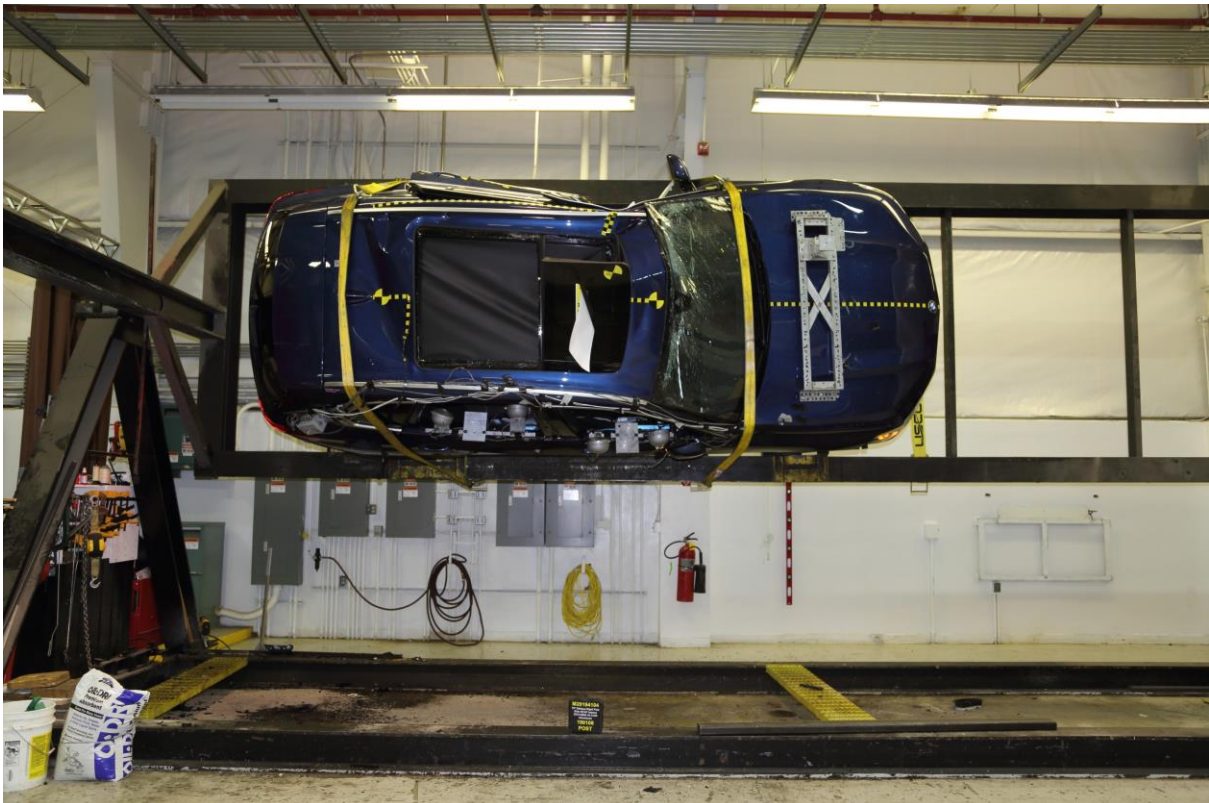
No. 064 FMVSS No. 301 Static Rollover 90 Degrees
