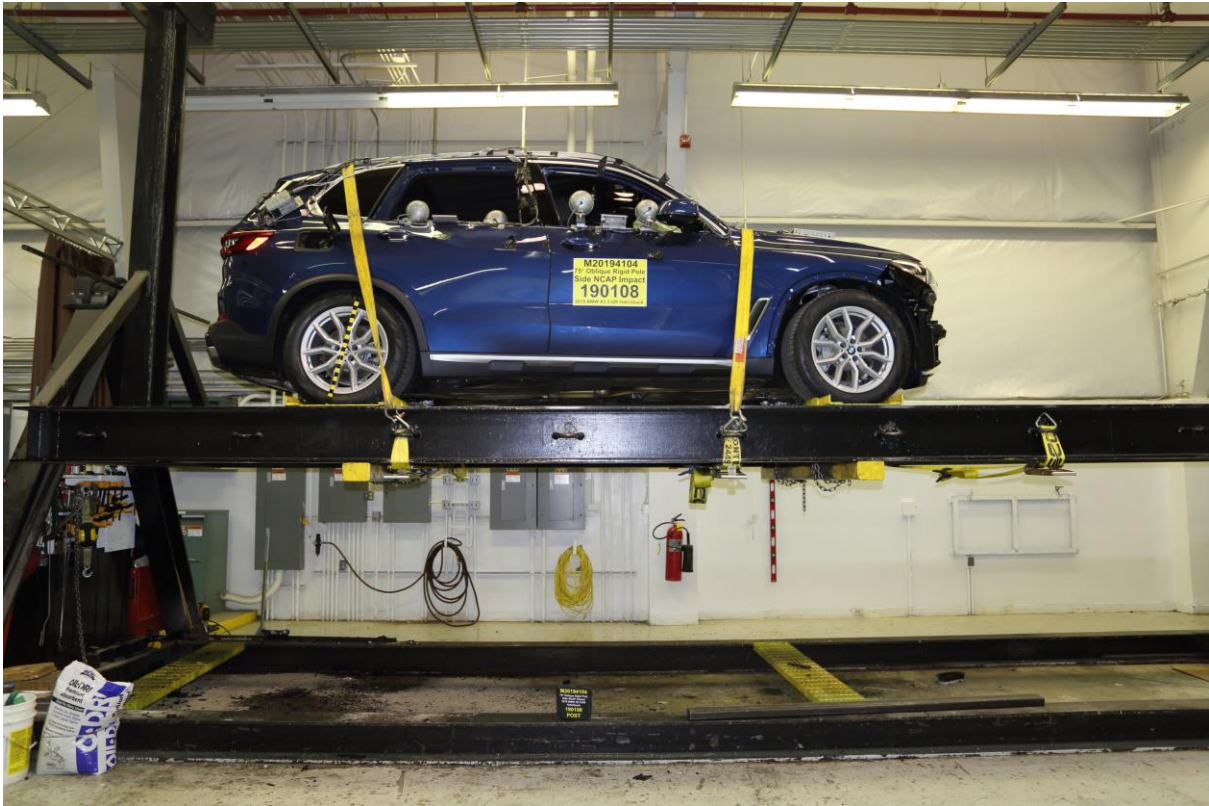
No. 067 FMVSS No. 301 Static Rollover 360 Degrees
