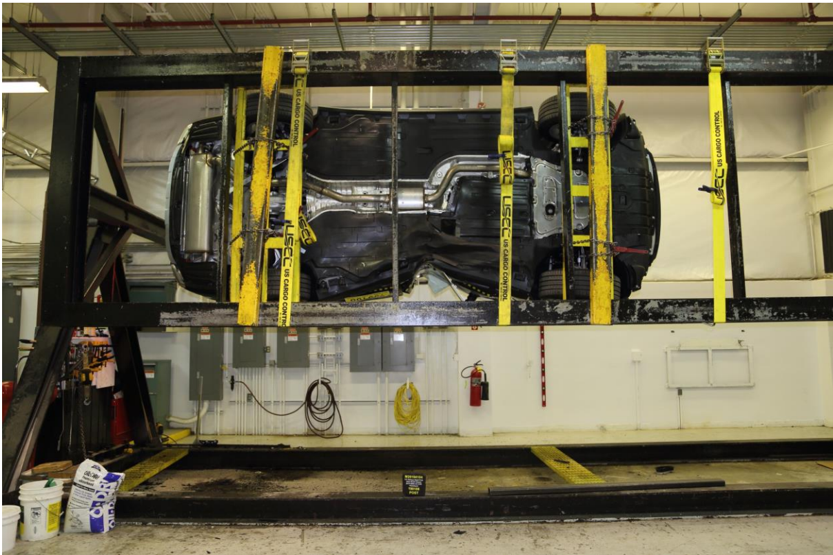
No. 066 FMVSS No. 301 Static Rollover 270 Degrees
