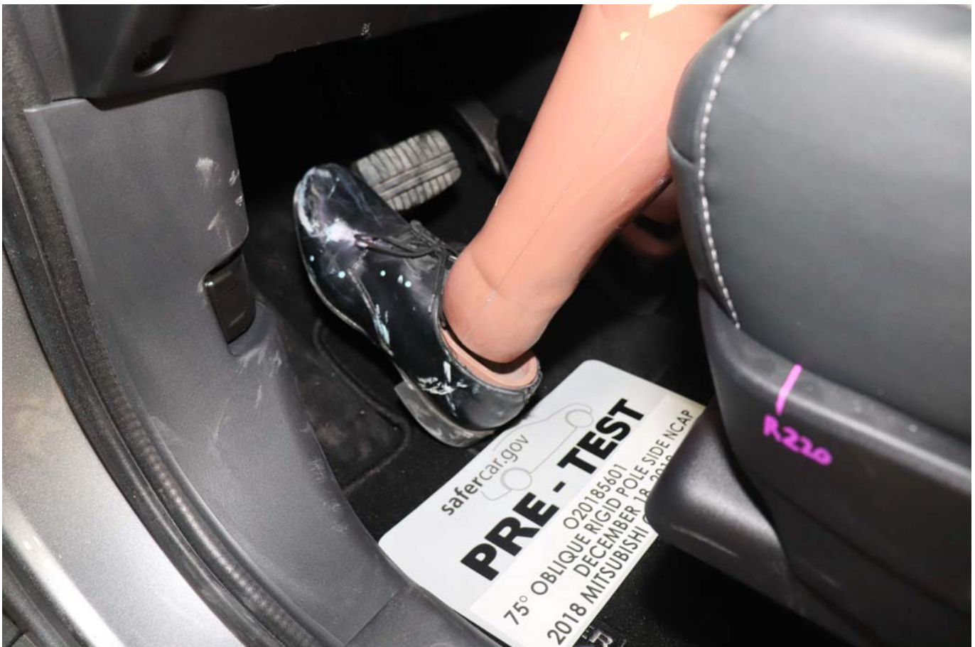
Photo No. 032 - Pre-Test Placement of Dummy Feet
