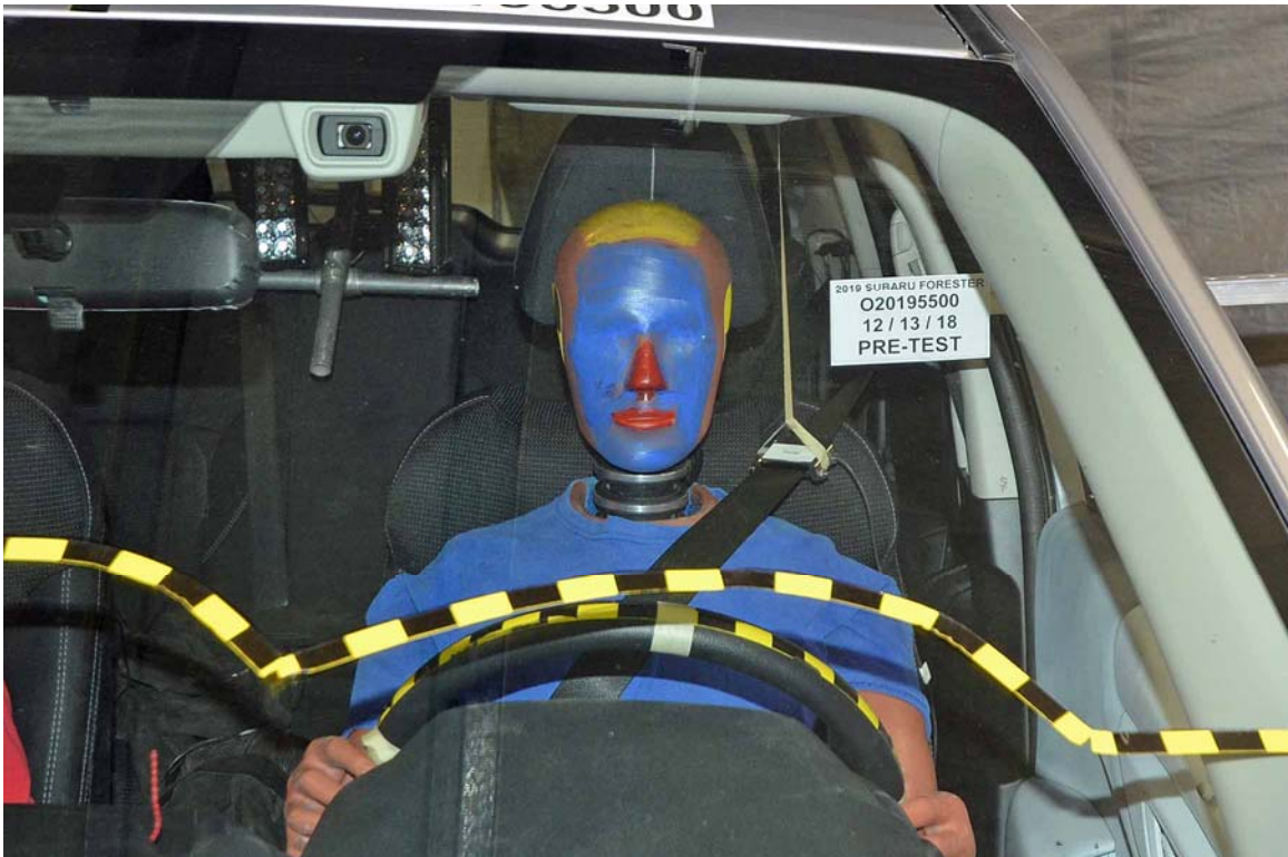
FIGURE 30. Pre-Test Driver Dummy Front View
