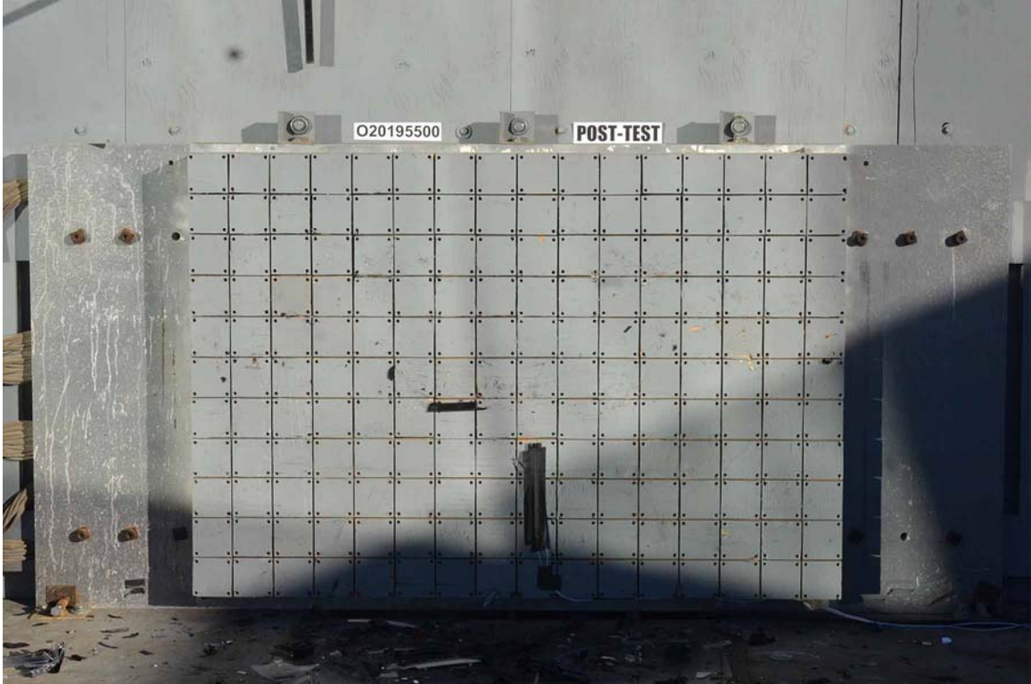
FIGURE 3. Post-Test Load Cell Wall
