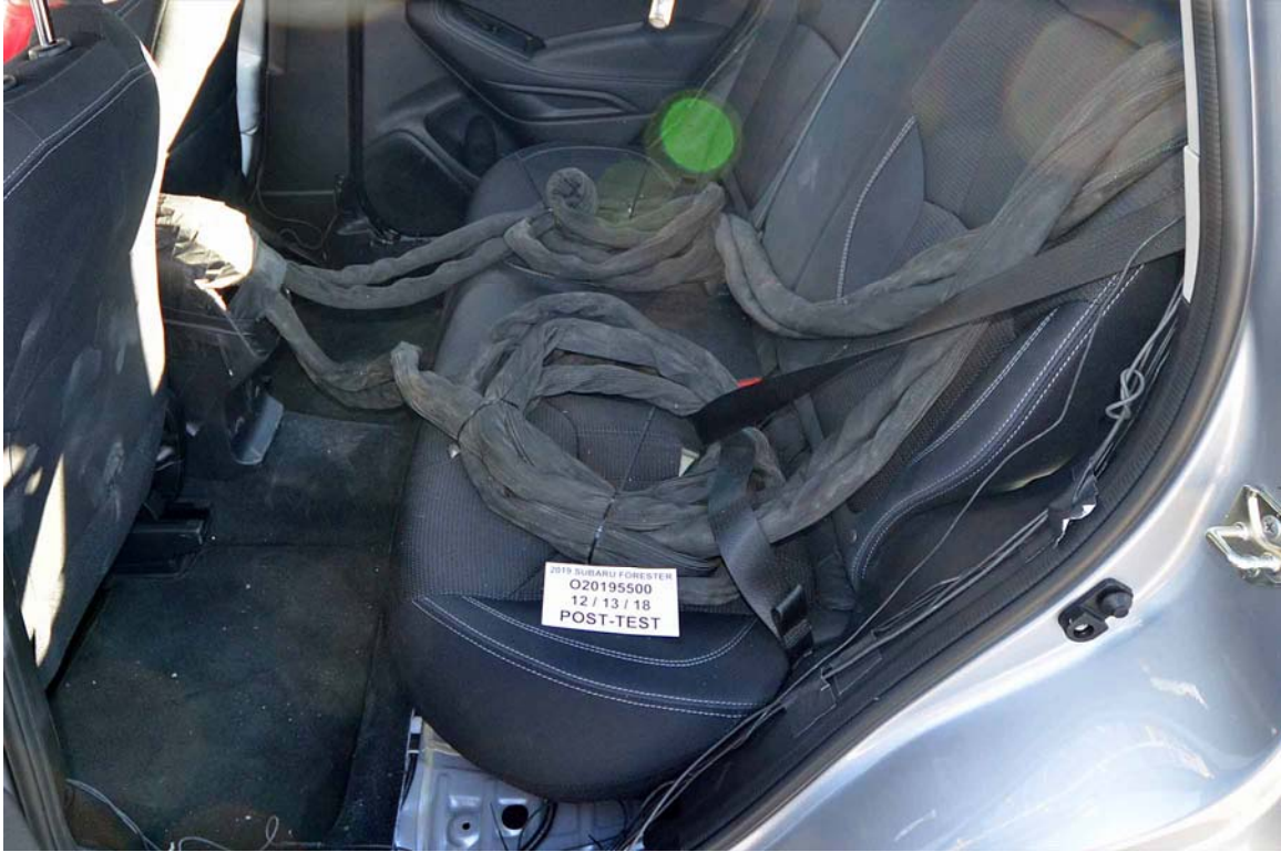
FIGURE 29. Post-Test Dummy Cable Routing
