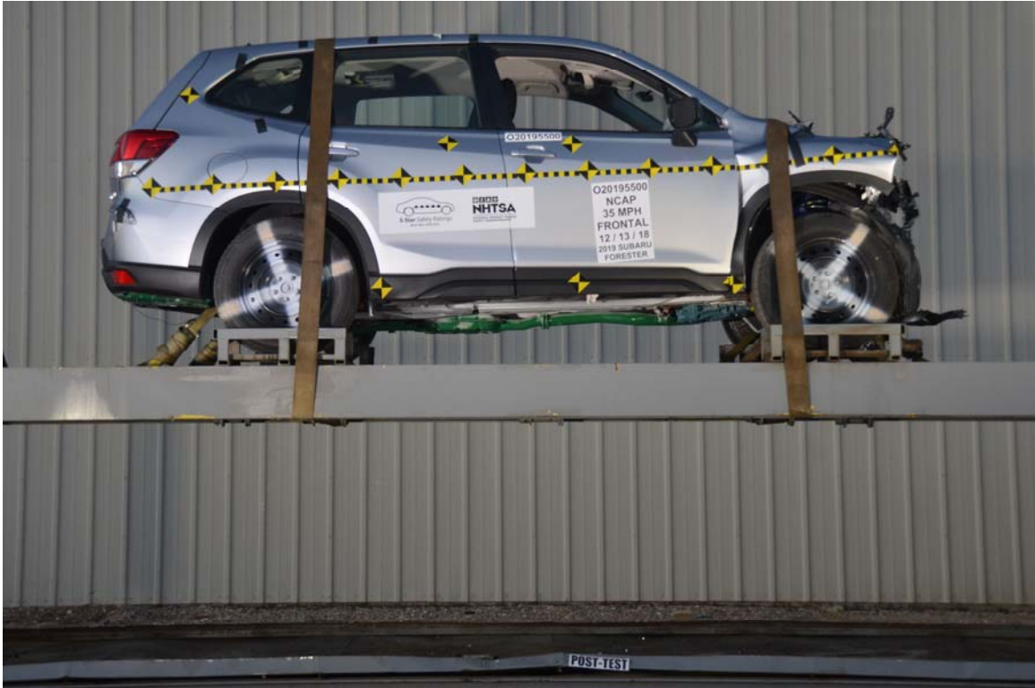
FIGURE 73. Vehicle at 0° on Static Rollover Device
