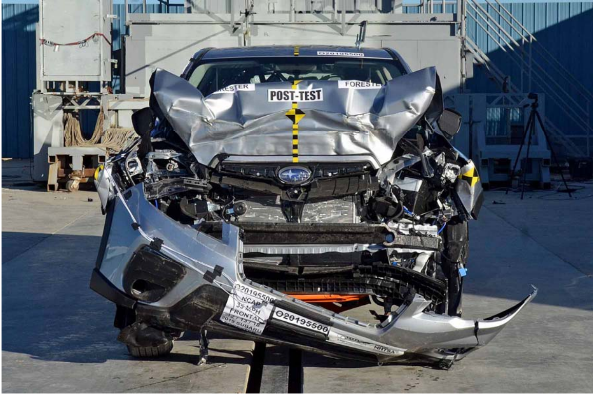
FIGURE 9. Post-Test Front View of Test Vehicle
