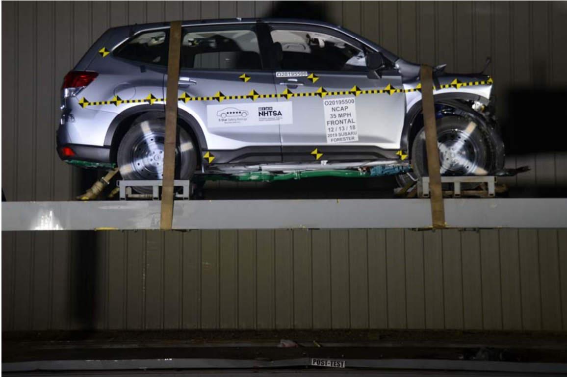
FIGURE 77. Vehicle at 360° on Static Rollover Device
