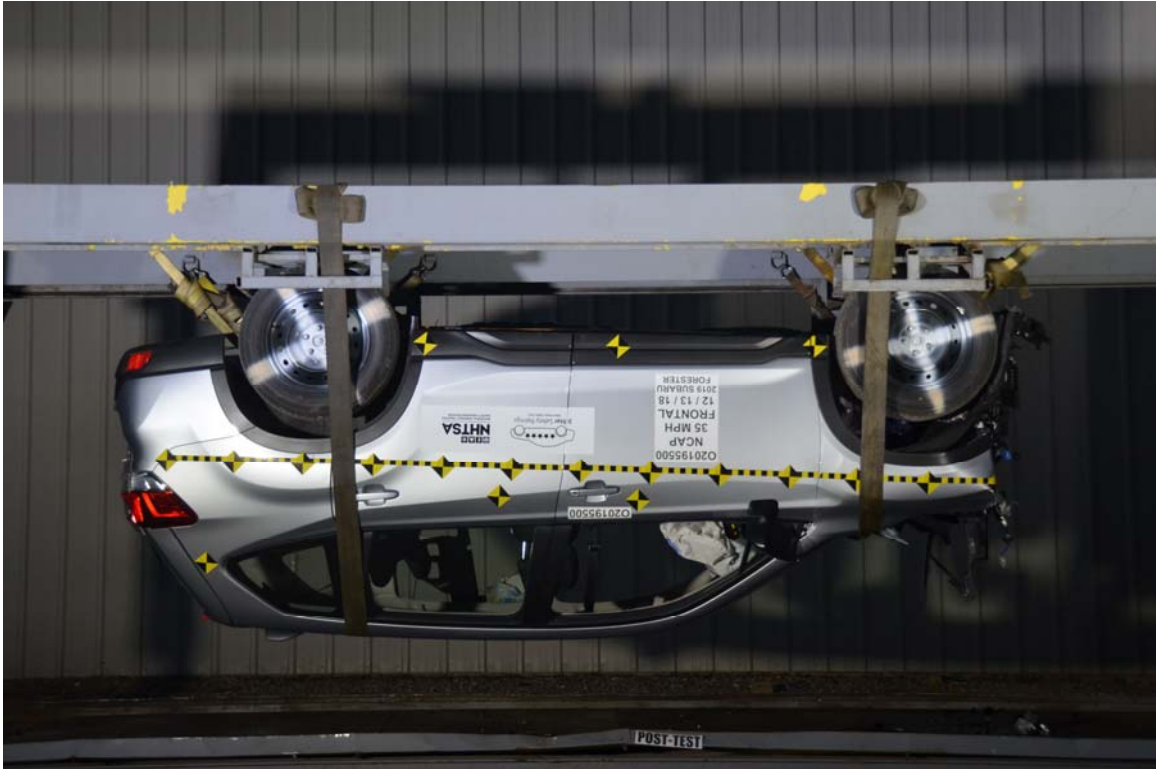
FIGURE 75. Vehicle at 180° on Static Rollover Device
