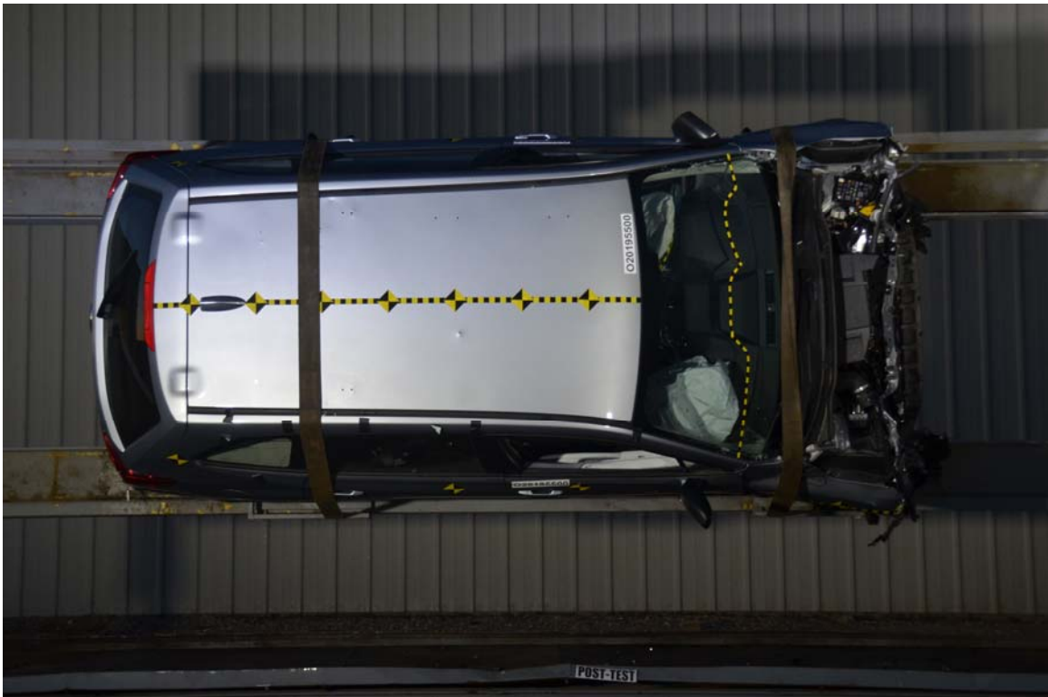
FIGURE 74. Vehicle at 90° on Static Rollover Device
