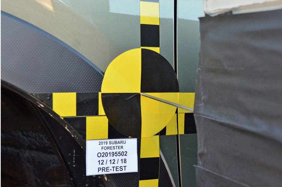
FIGURE 19. Pre-Test Close-Up View of Impact Point Target
