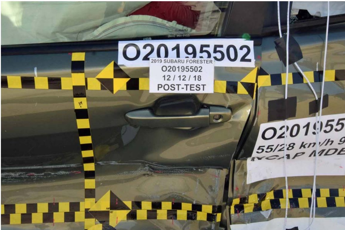
FIGURE 22. Post-Test Left Front Door Latch Close-Up
