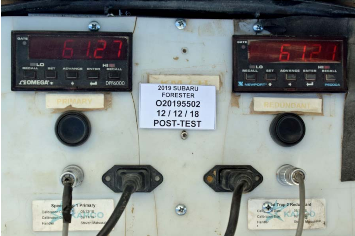
FIGURE 95. Post-Test Primary and Redundant Speed Trap Read-Out
