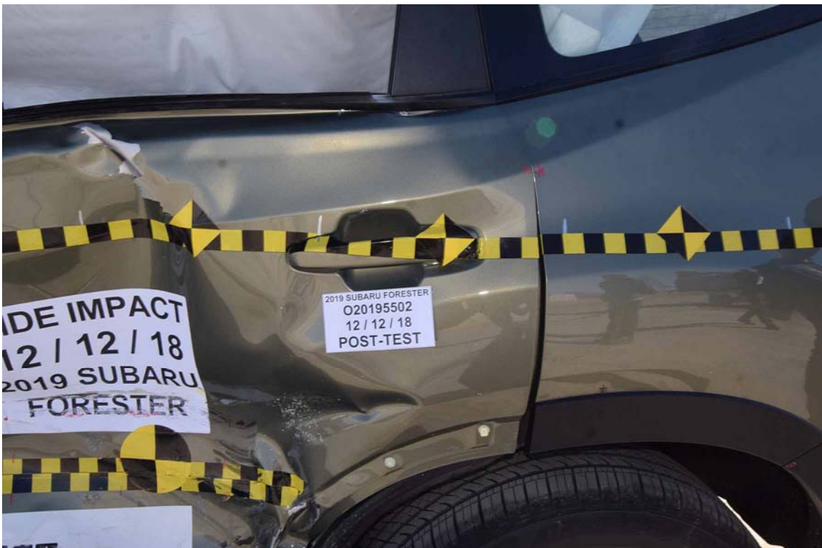
FIGURE 24. Post-Test Left Rear Door Latch Close-Up
