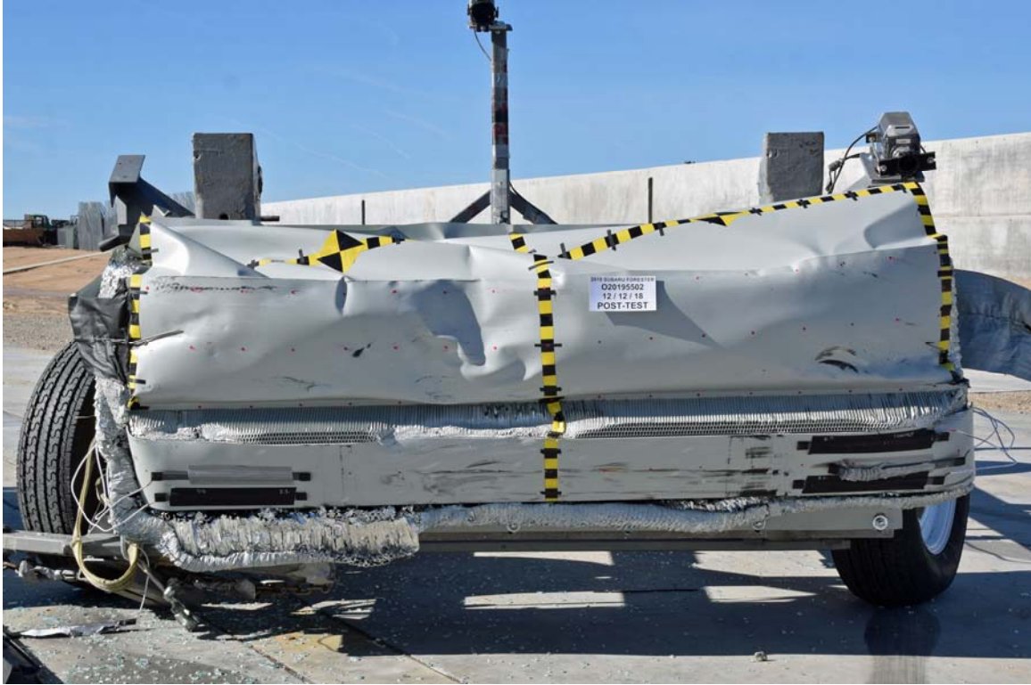
FIGURE 85. Post-Test Front View of MDB Impactor Face
