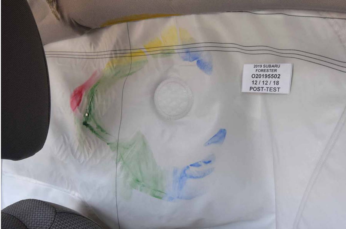
FIGURE 49. Post-Test Driver Dummy Close-Up Head Contact with Side Airbag View
