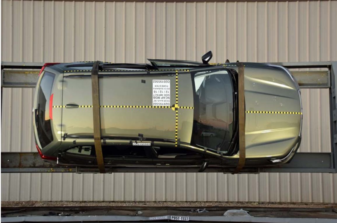
FIGURE 97. FMVSS No. 301 Static Rollover 90 Degrees
