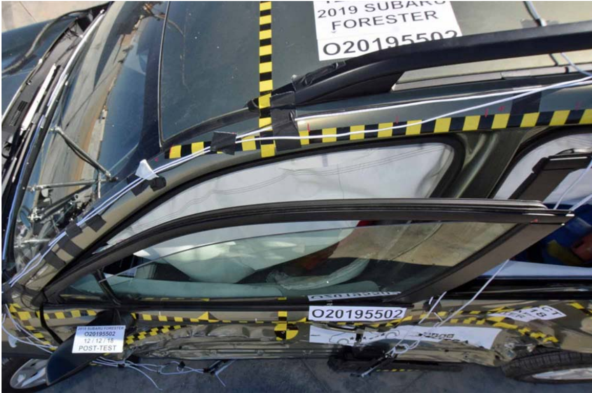
FIGURE 43. Post-Test Driver Dummy and Door Clearance View
