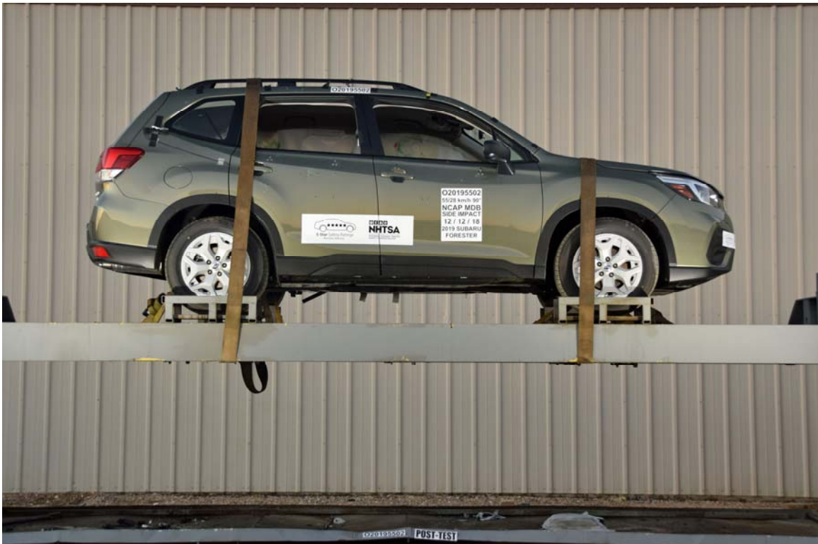
FIGURE 96. FMVSS No. 301 Static Rollover 0 Degrees
