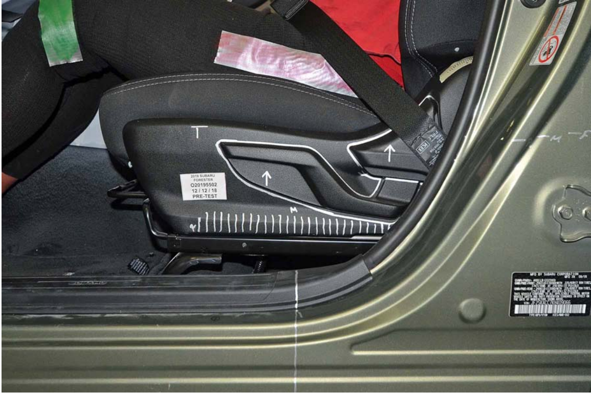
FIGURE 39. Pre-Test Close-Up Left Side View of Driver Seat Track
