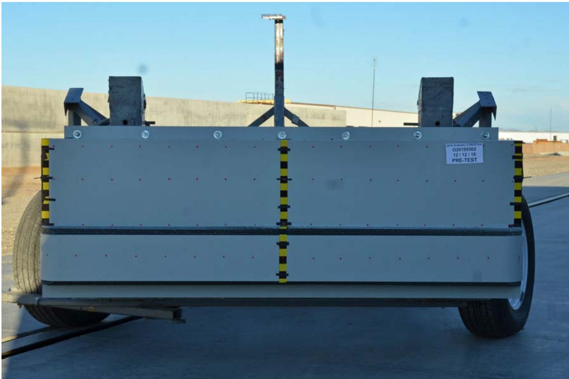
FIGURE 84. Pre-Test Front View of MDB Impactor Face
