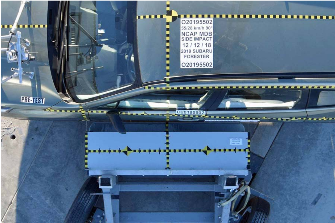
FIGURE 15. Pre-Test Overhead View of Test Area
