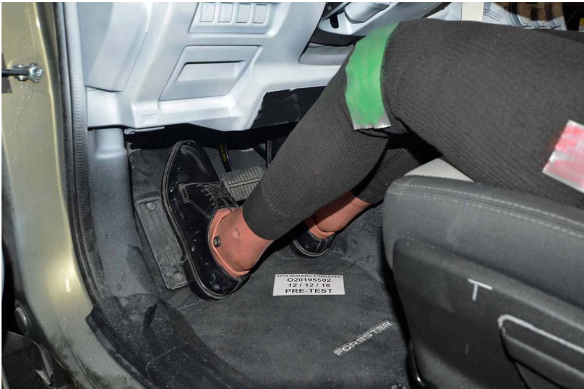
FIGURE 34. Pre-Test Placement of Driver Dummy's Feet
