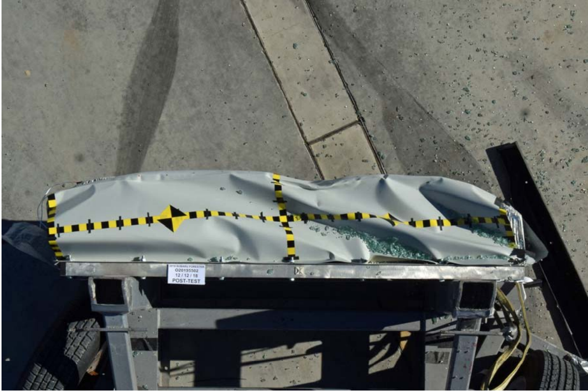
FIGURE 87. Post-Test Top View of MDB Impactor Face
