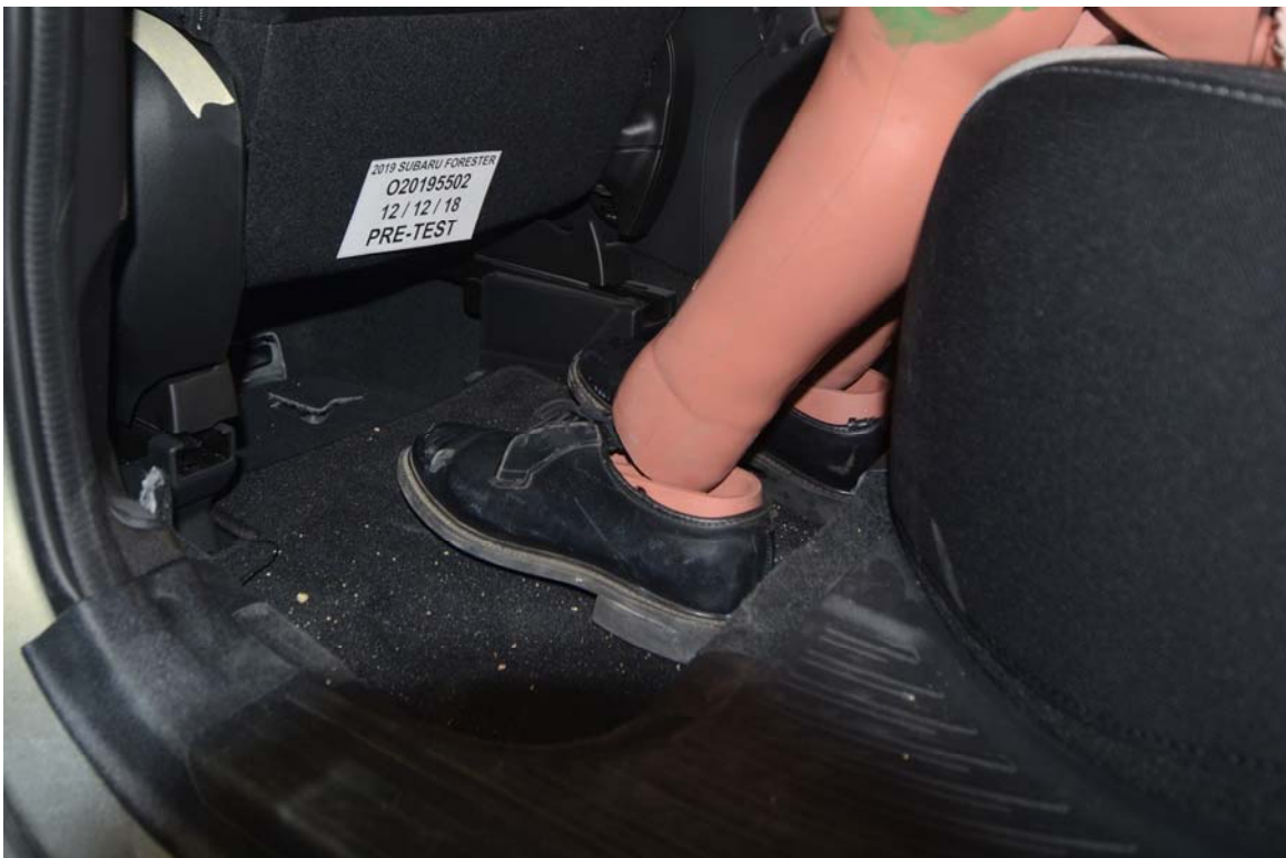
FIGURE 64. Pre-Test Placement of Rear Passenger Dummy's Feet
