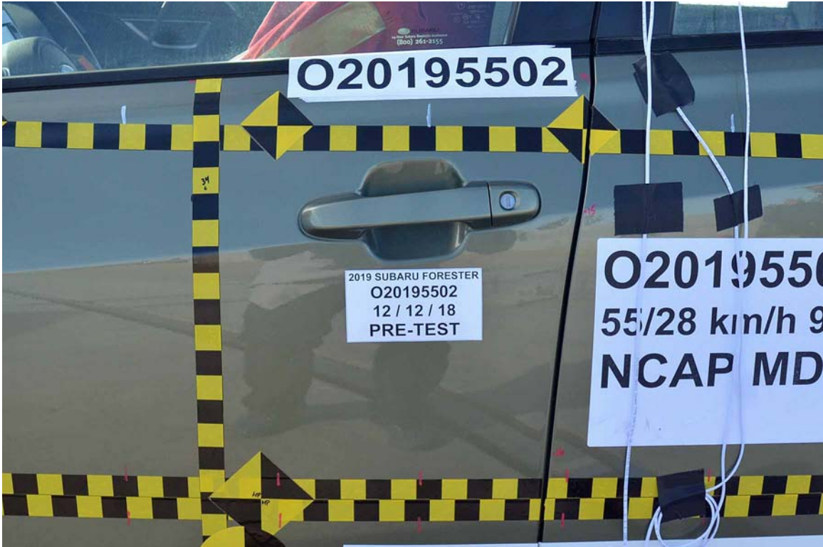
FIGURE 21. Pre-Test Left Front Door Latch Close-Up
