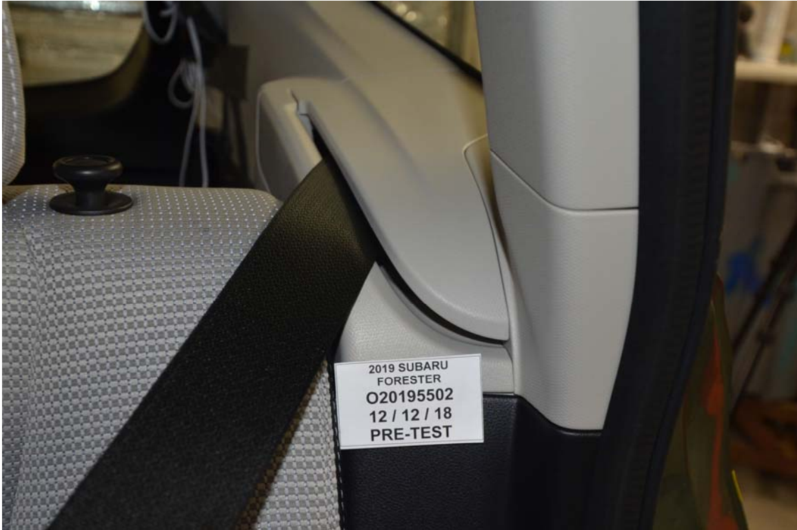
FIGURE 65. Pre-Test View of Belt Anchorage for Rear Passenger Dummy
