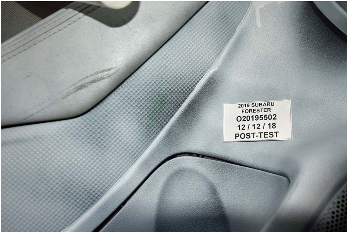
FIGURE 54. Post-Test Driver Dummy Close-Up Knee Contact View
