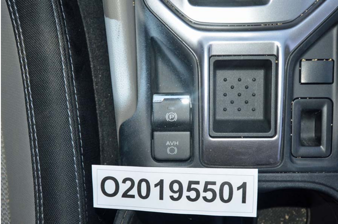
FIGURE 35. View of Disengaged Parking Brake
