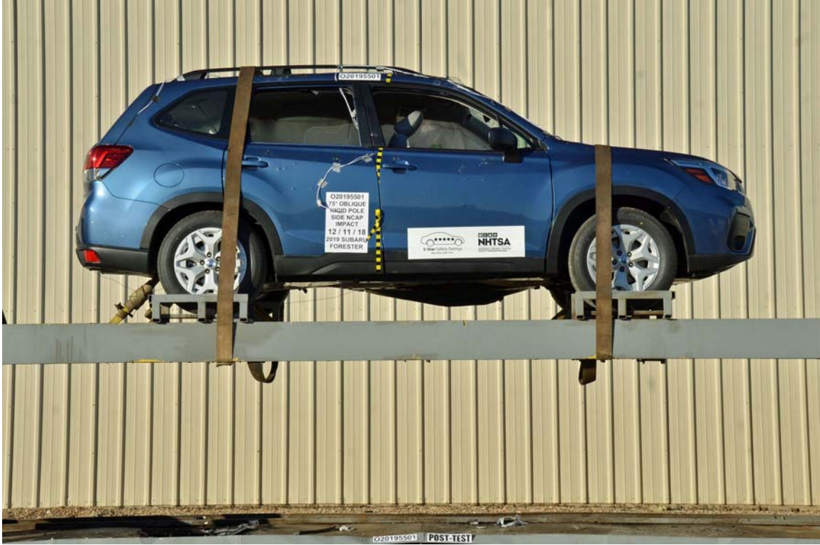
FIGURE 67. FMVSS No. 301 Static Rollover 360 Degrees
