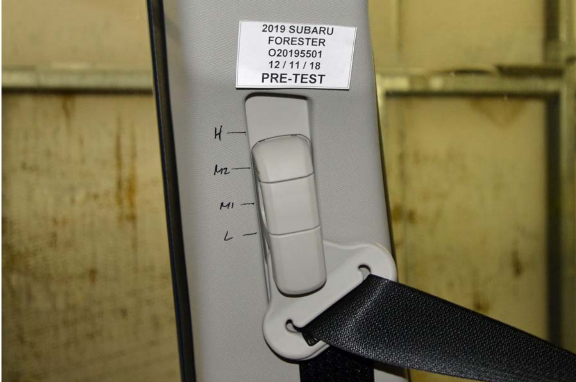
FIGURE 33. Pre-Test View of Belt Anchorage for Dummy
