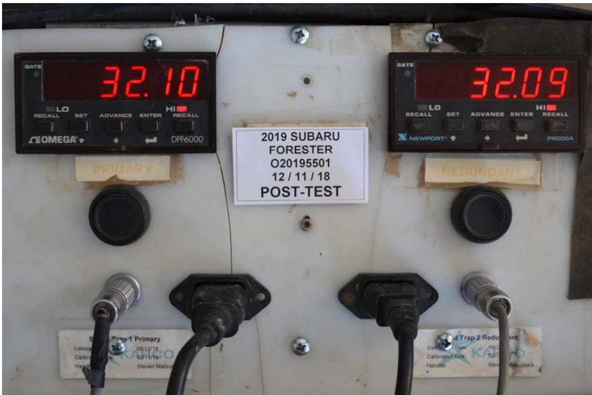
FIGURE 62. Post-Test Primary and Redundant Speed Trap Read-Out
