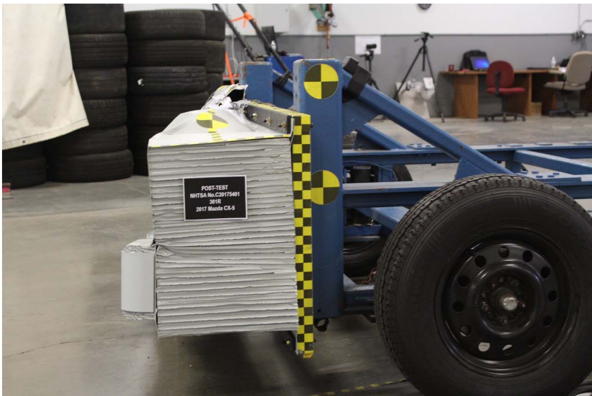
Figure A-22: Post-Test MDB Left Side View
