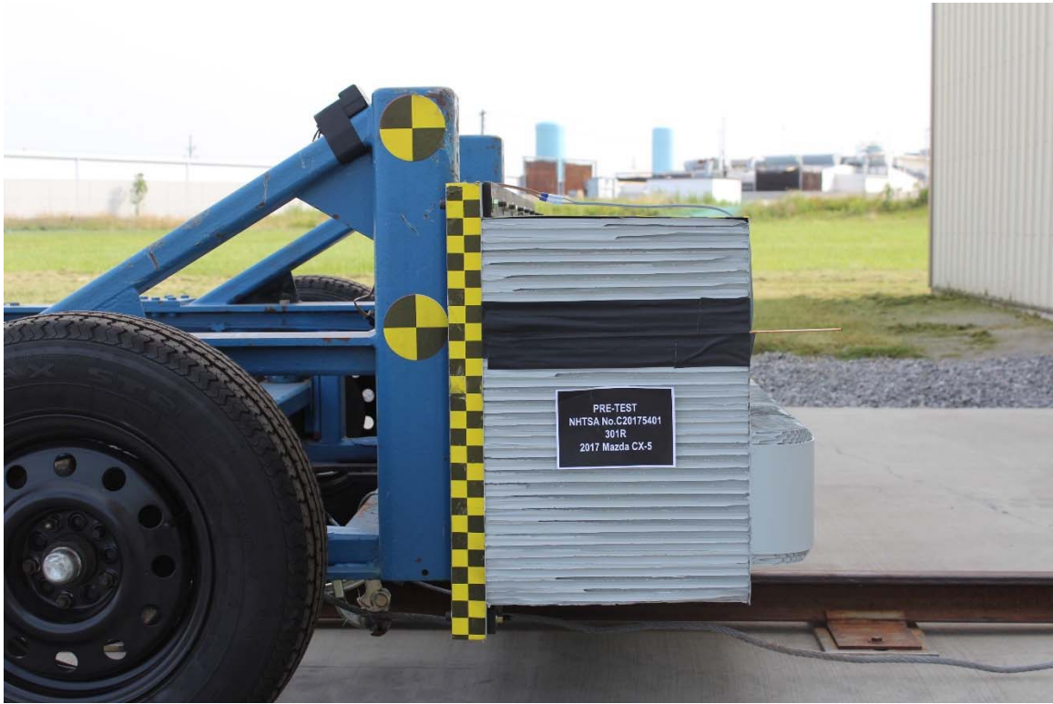
Figure A-23: Pre-Test MDB Right Side View
