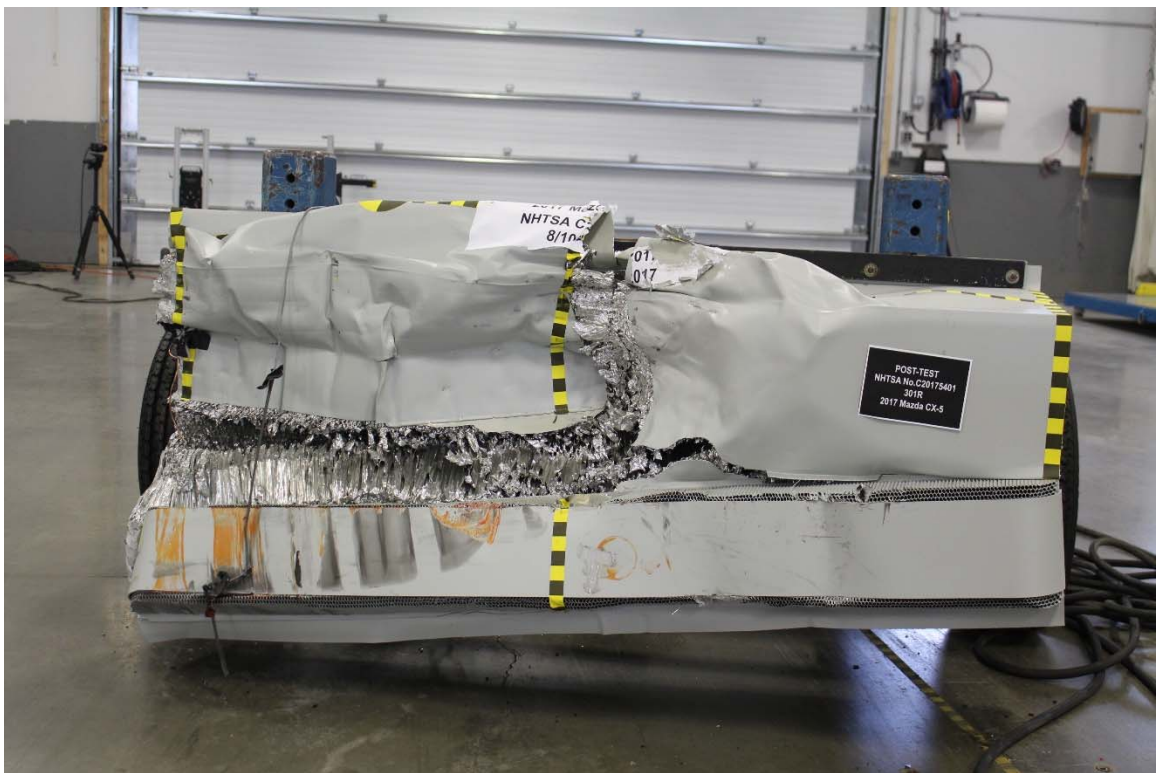
Figure A-20: Post-Test MDB Front View
