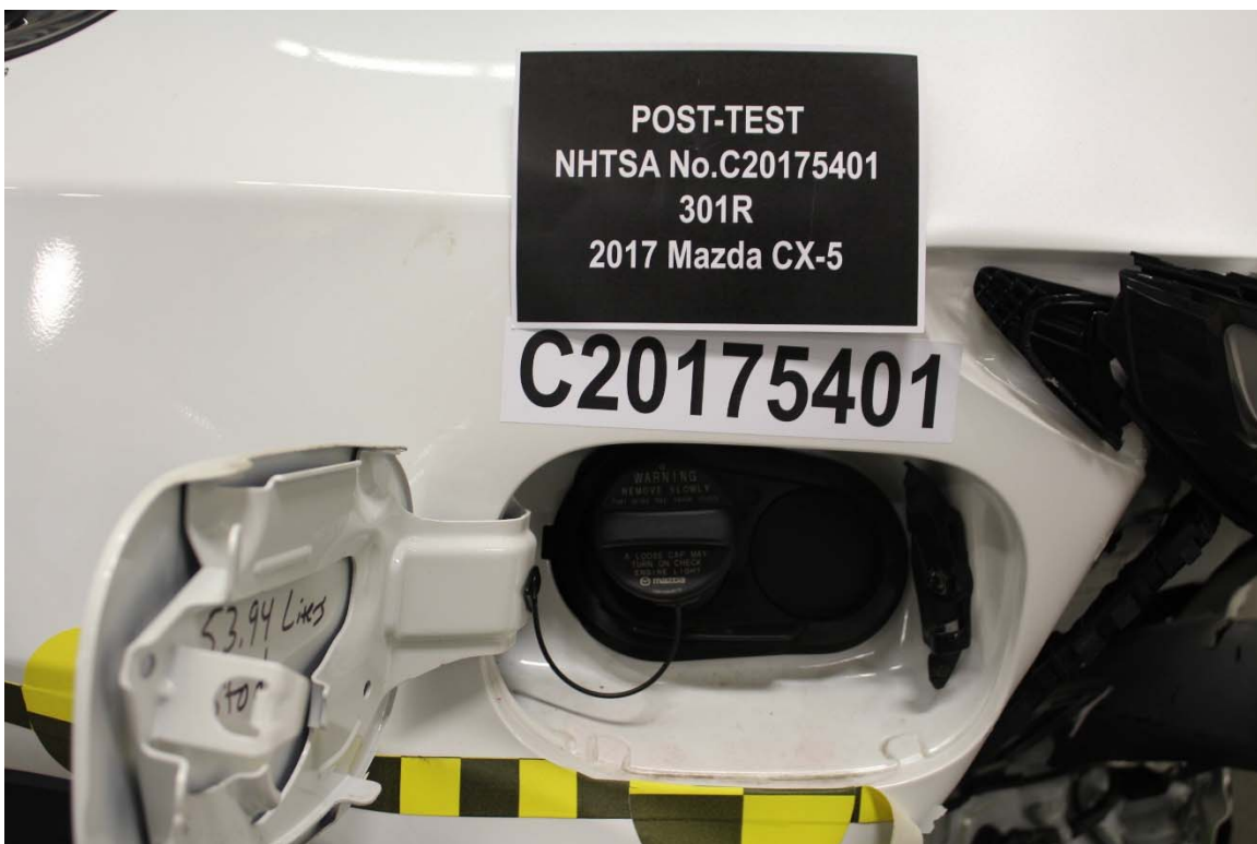
Figure A-36: Post-Test Fuel Filler Cap View
