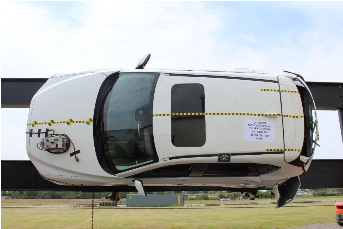
Figure A-39: Rollover 90° View
