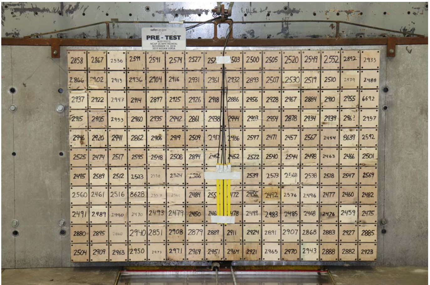
Photo No. 002 - Pre-Test Load Cell Wall
