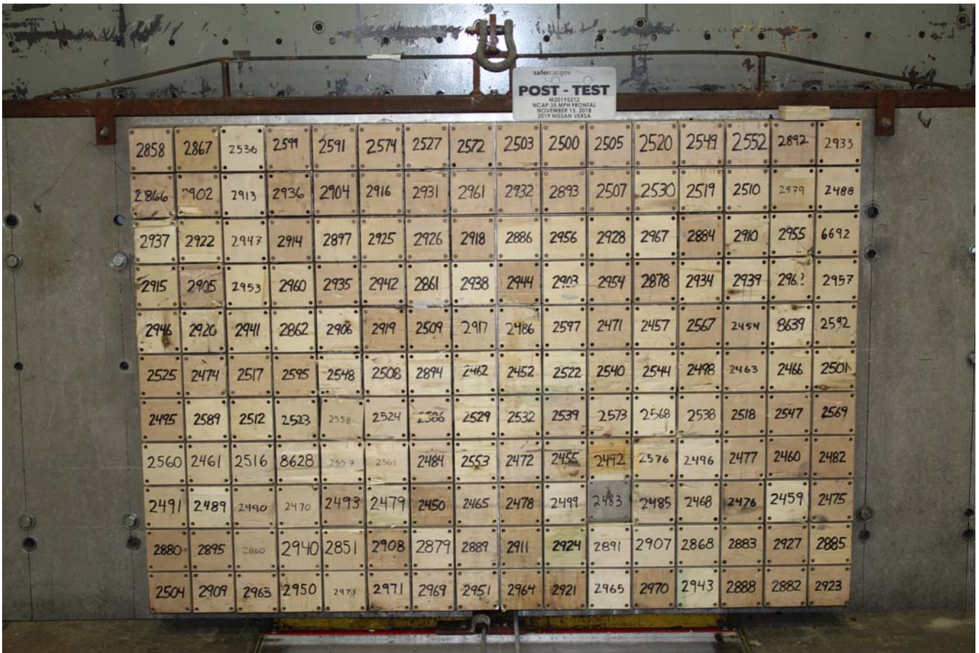
Photo No. 003 - Post-Test Load Cell Wall
