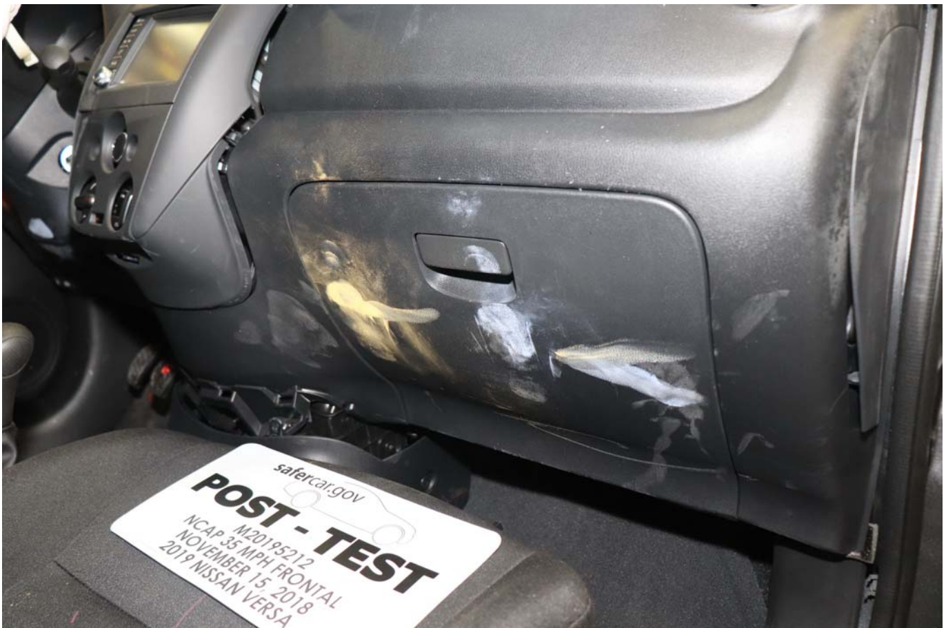
Photo No. 064 - Post-Test Passenger Side Knee Bolster
