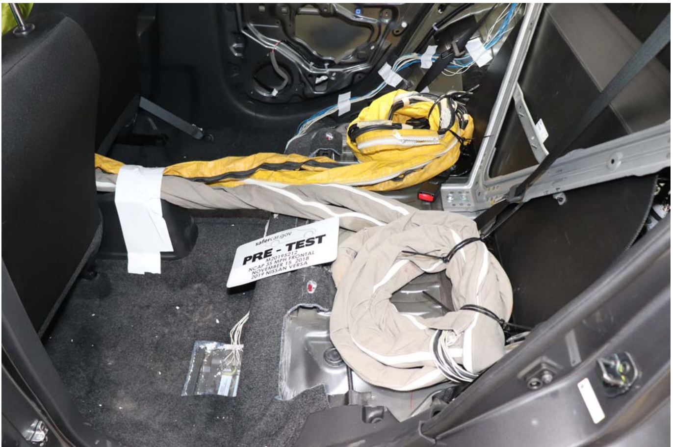
Photo No. 028 - Pre-Test Dummy Cable Routing
