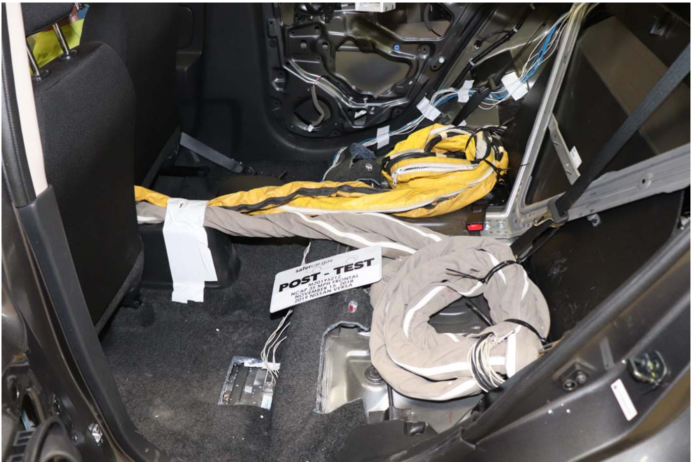
Photo No. 029 - Post-Test Dummy Cable Routing
