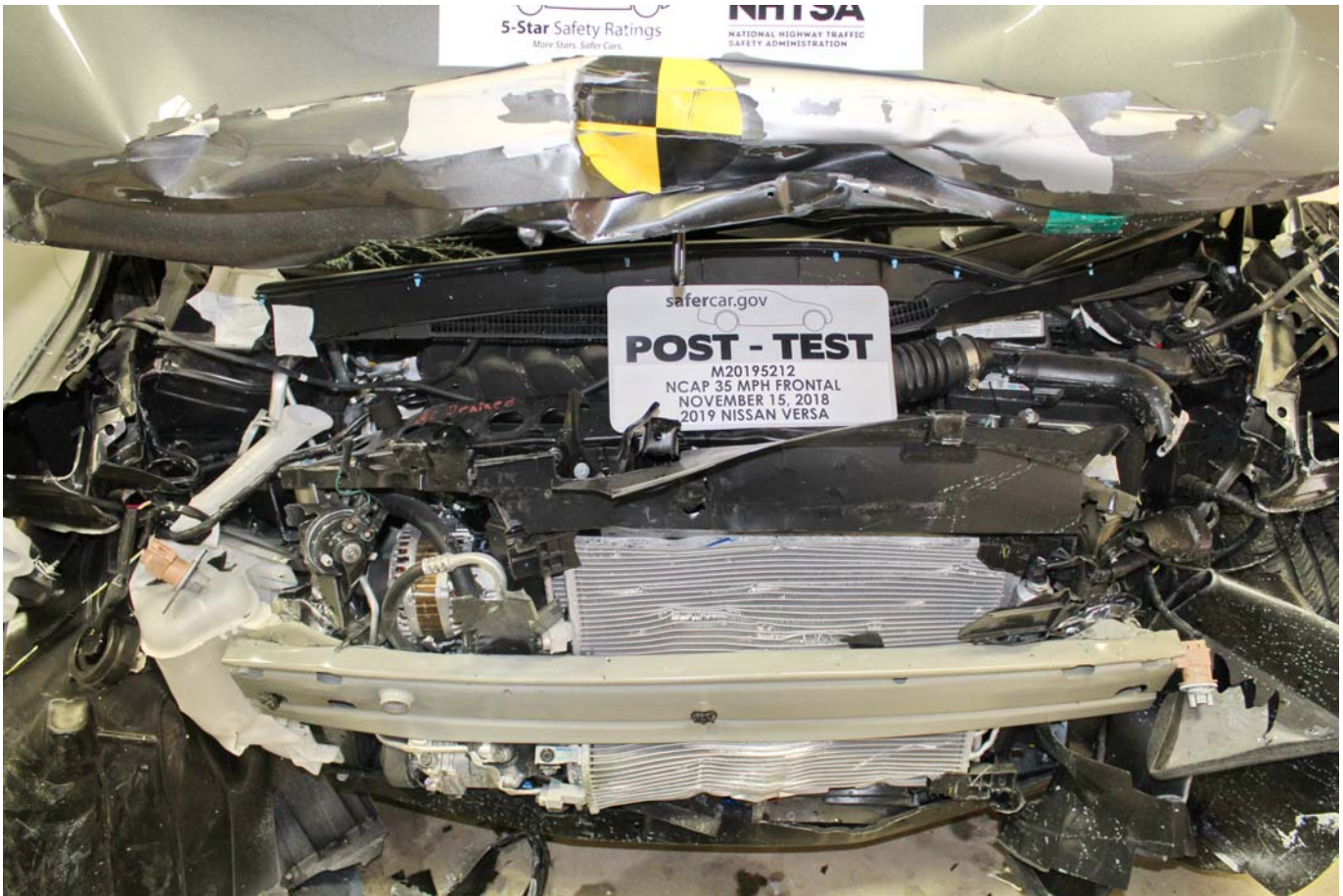
Photo No. 021 - Post-Test Engine Compartment View
