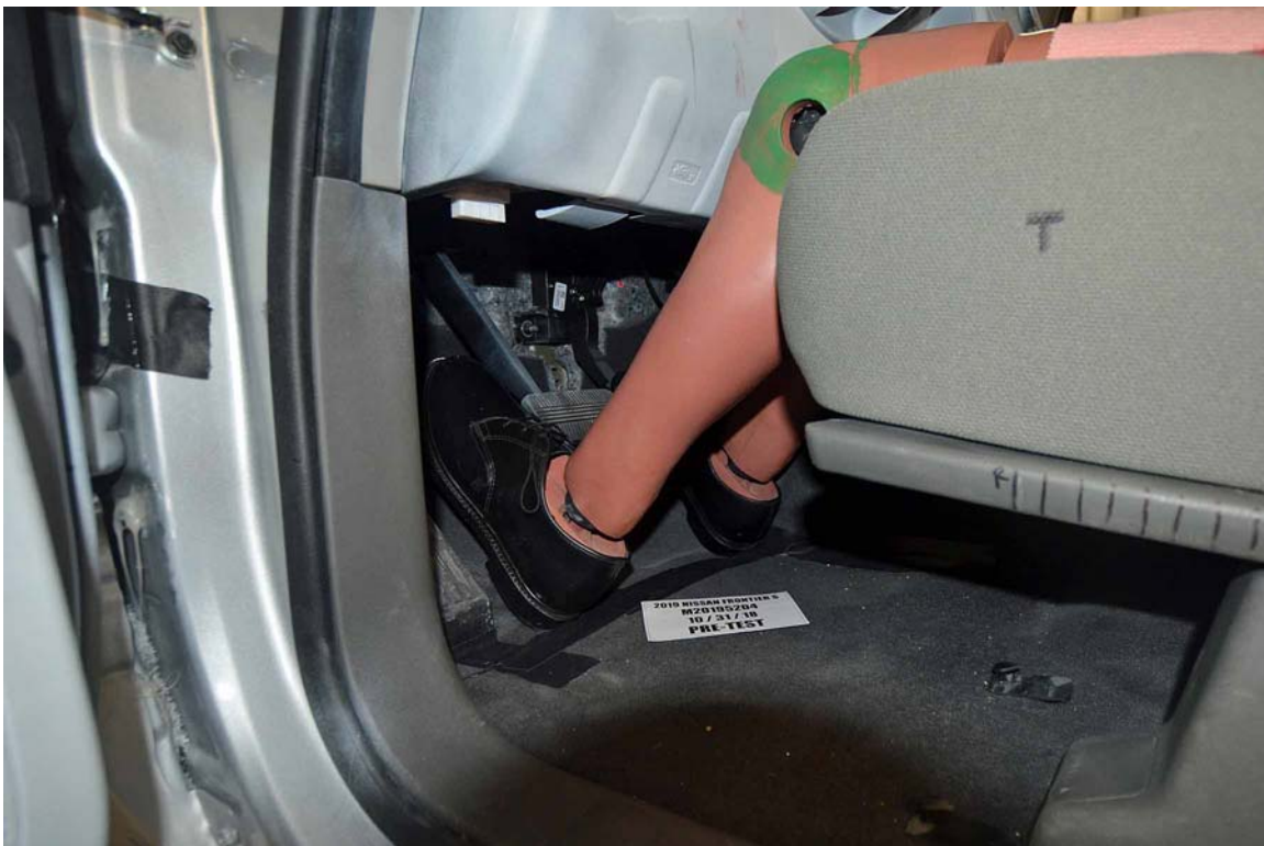
FIGURE 32. Pre-Test Placement of Dummy's Feet
