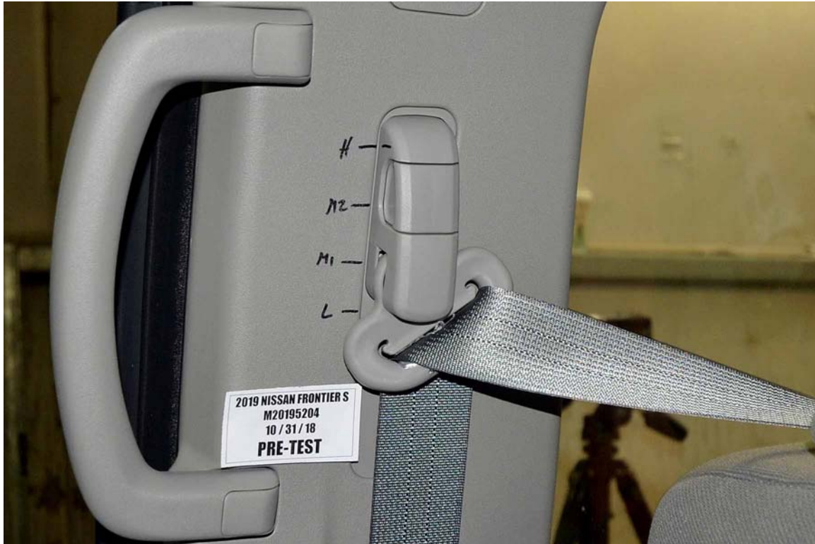
FIGURE 33. Pre-Test View of Belt Anchorage for Dummy
