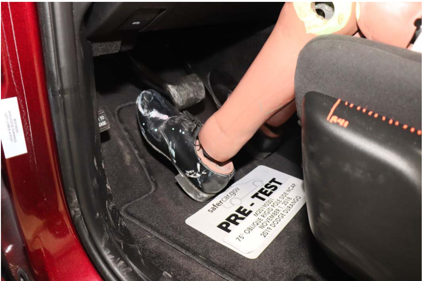
Photo No. 032 - Pre-Test Placement of Dummy Feet
