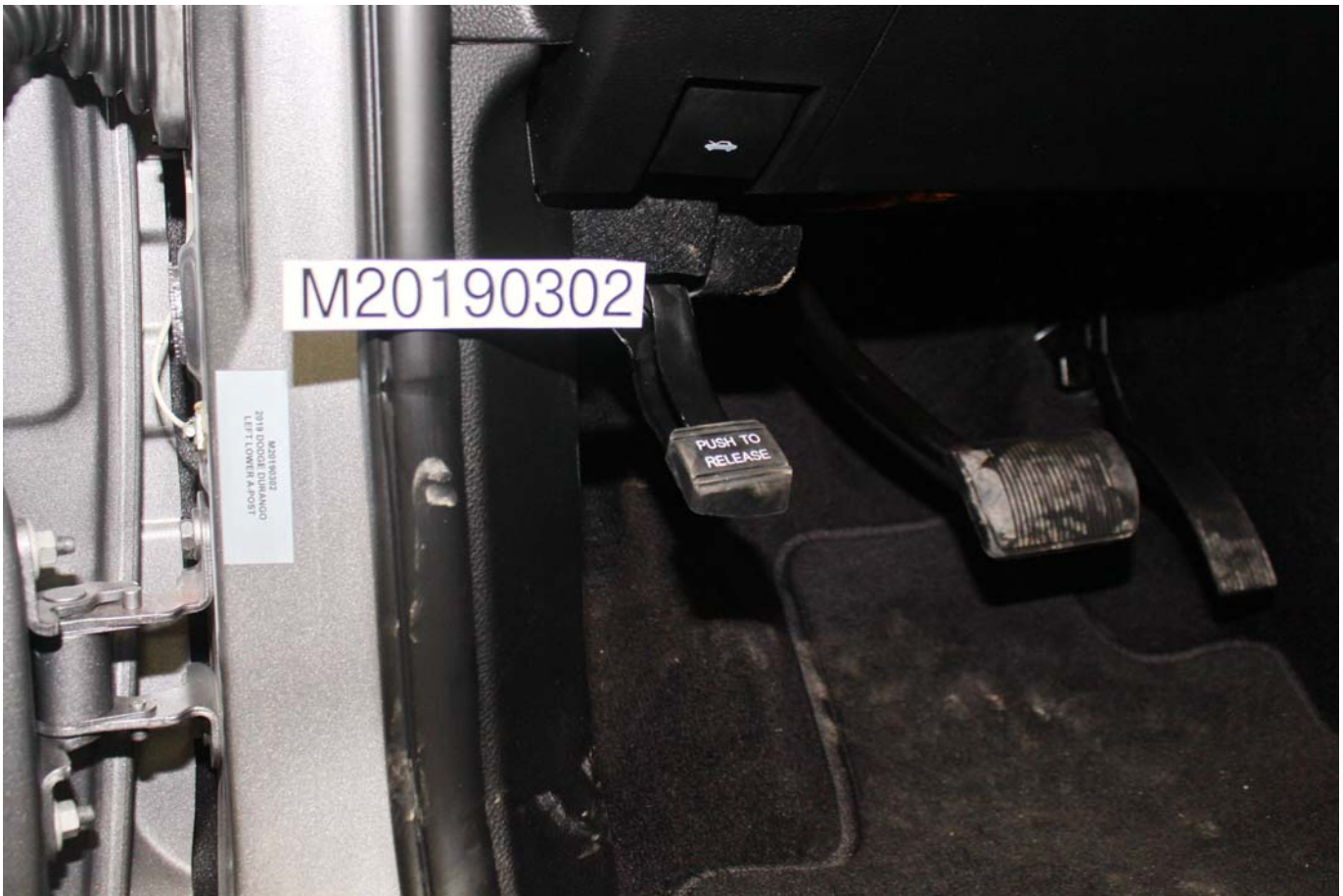
Photo No. 037 - Pre-Test View of Disengaged Parking Brake
