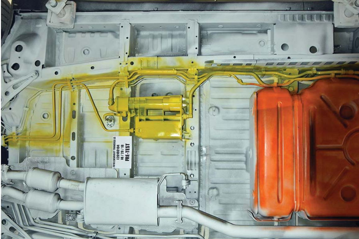
FIGURE 29. Pre-Test Underbody View of Fuel Lines
