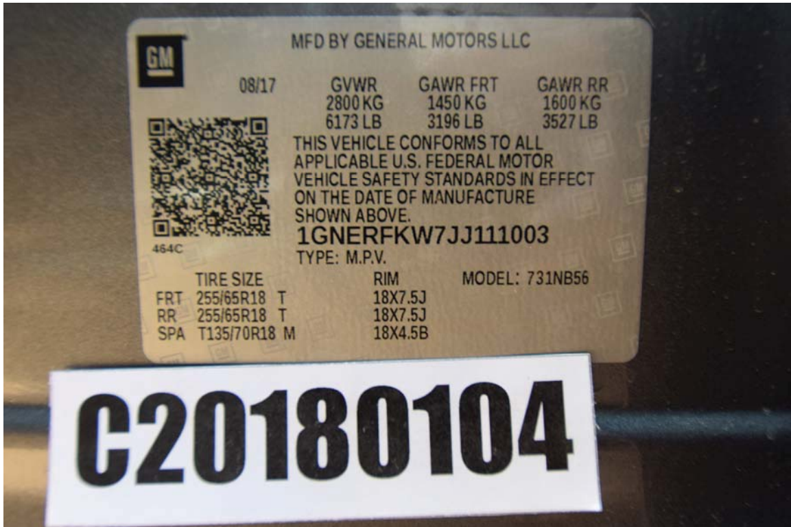
FIGURE 3. Test Vehicle Manufacturer's Label
