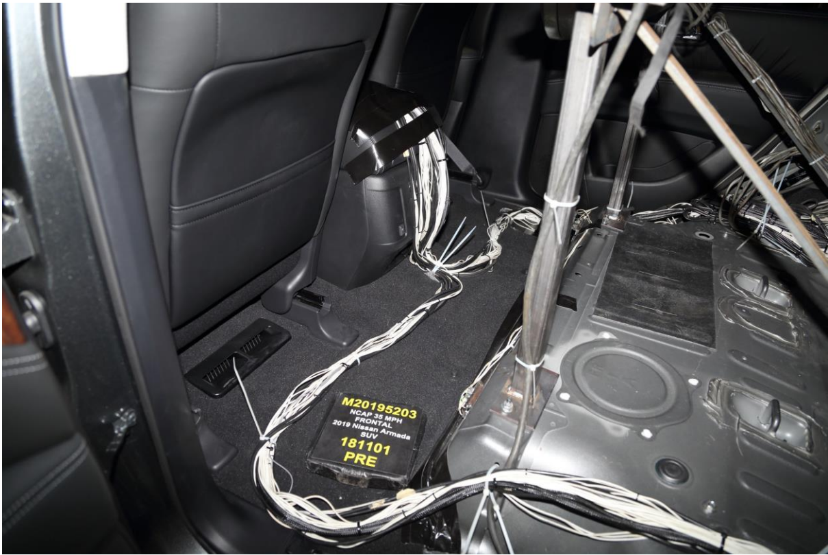
028 Pre-Test Dummy Cable Routing
