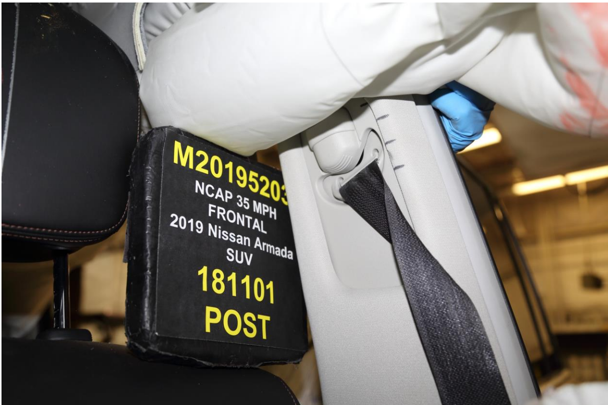
039 Post-Test View of Belt Anchorage for Driver Dummy
