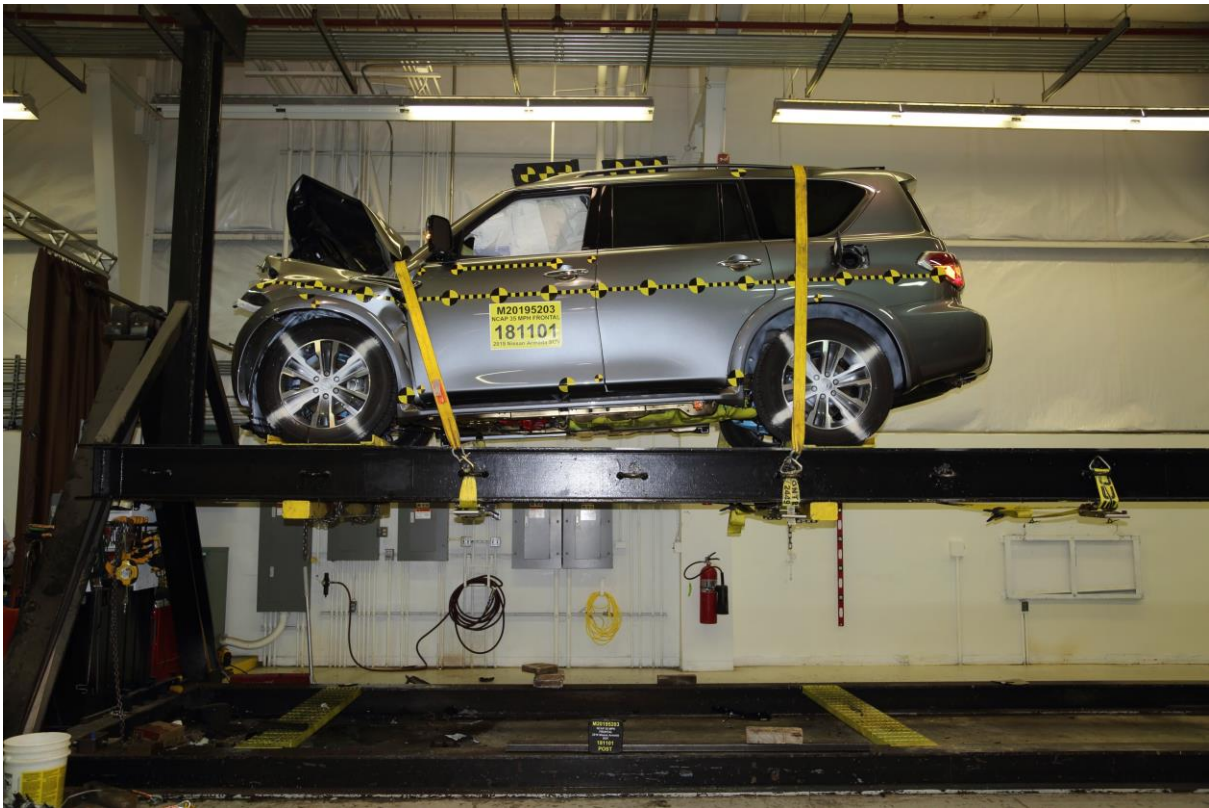
081 Vehicle at 360° on Static Rollover Device
