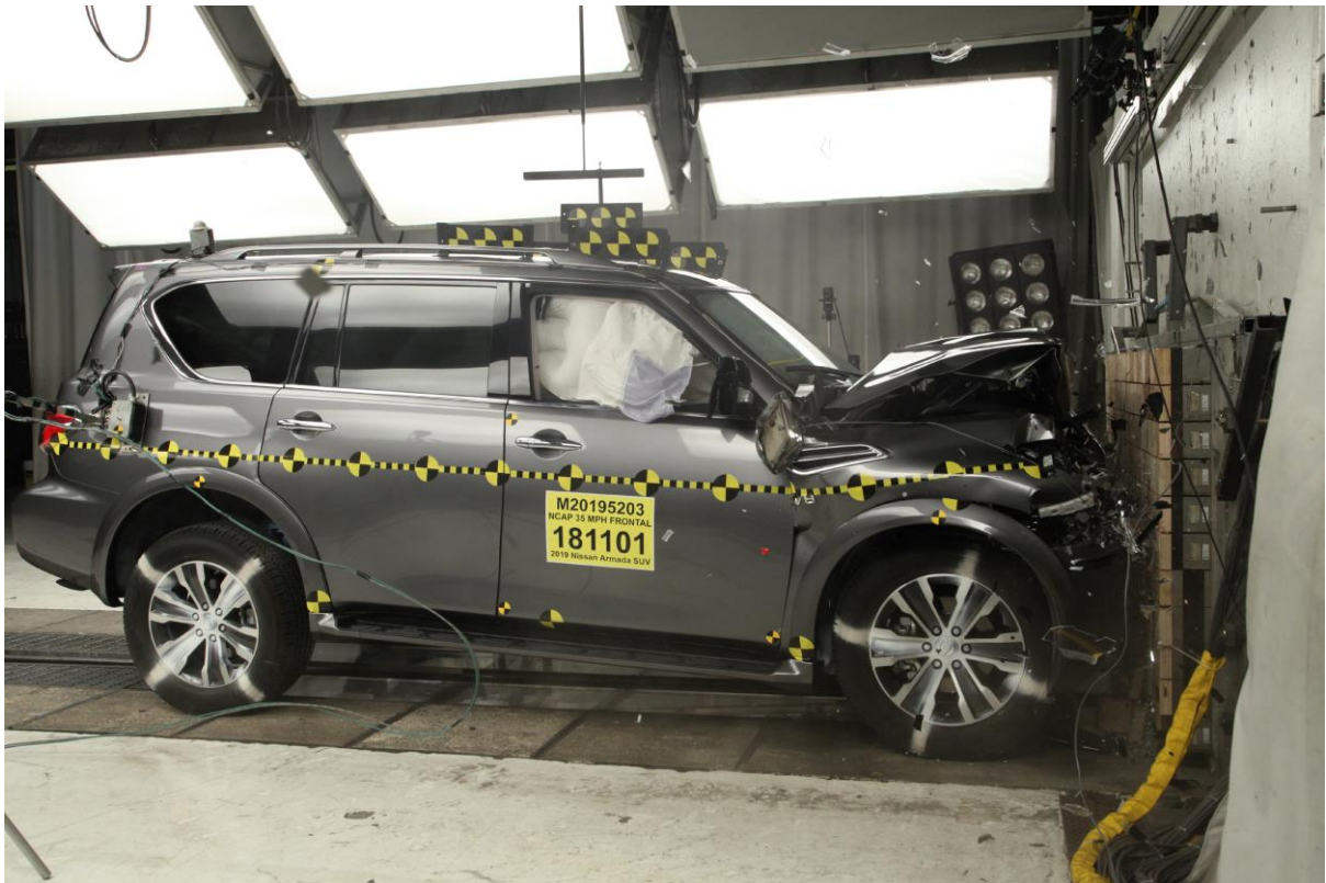
082 2019 Nissan Armada SUV Frontal Impact Event
