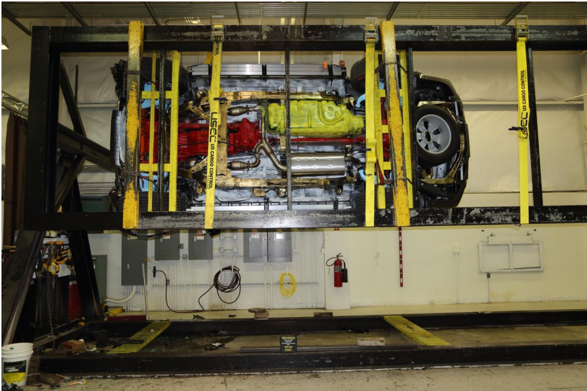
080 Vehicle at 270° on Static Rollover Device
