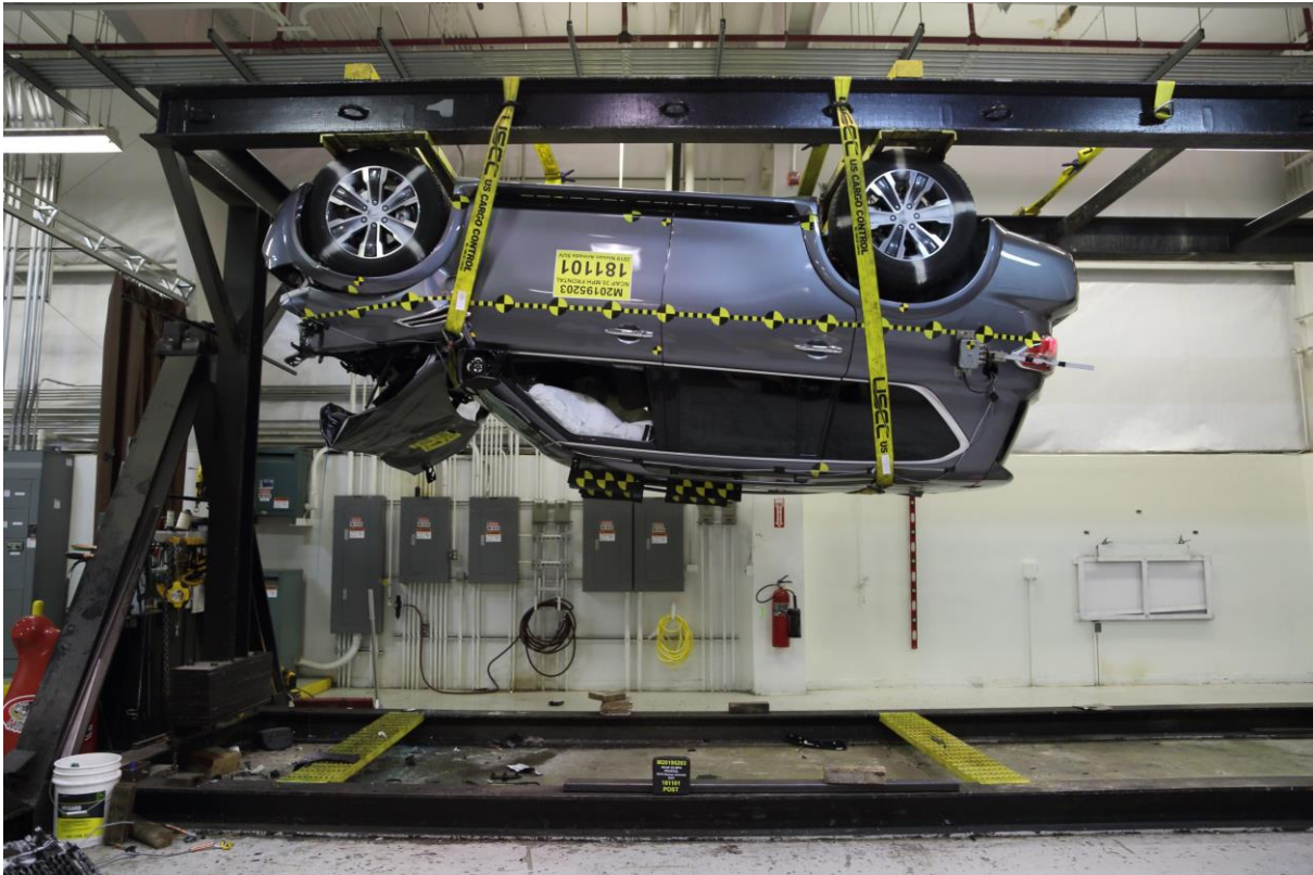
079 Vehicle at 180° on Static Rollover Device
