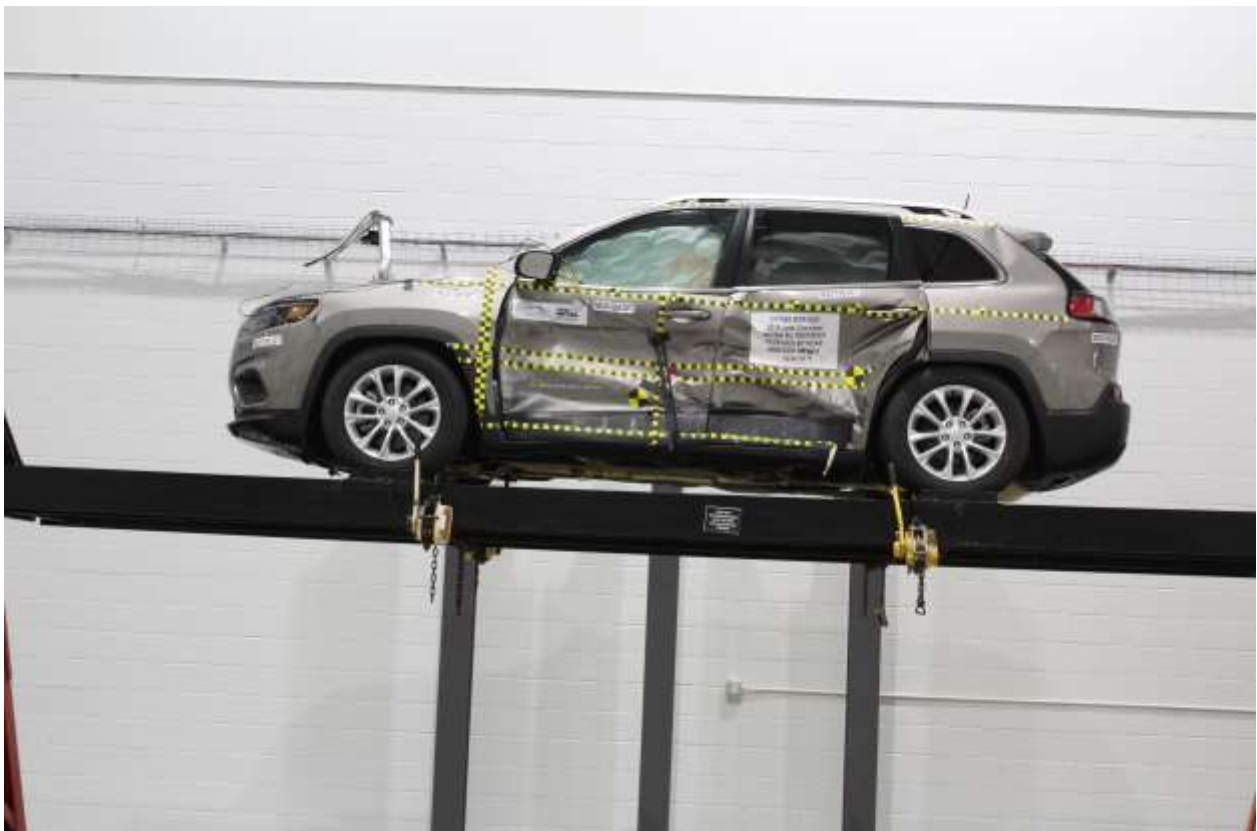
Figure A-100: FMVSS No. 301 Static Rollover 360 Degrees
