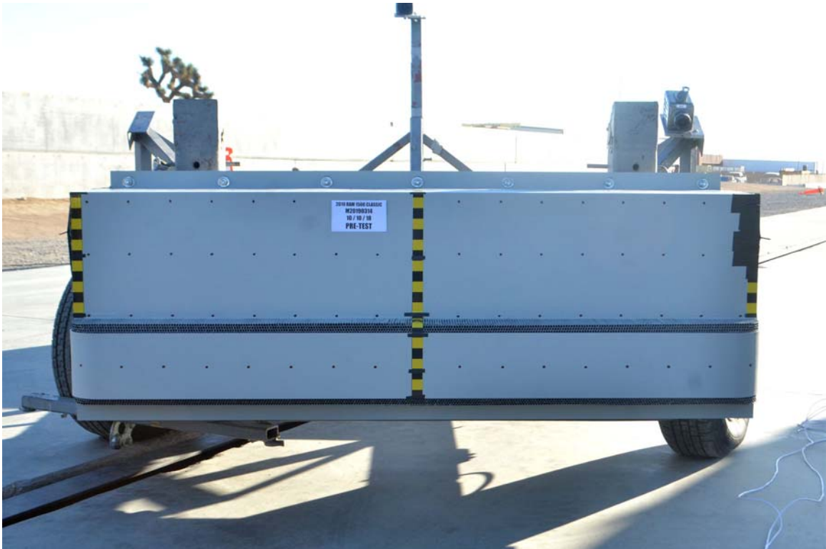
FIGURE 84. Pre-Test Front View of MDB Impactor Face
