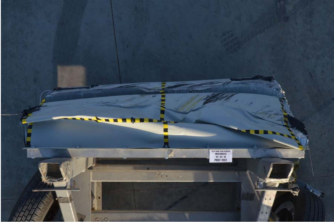
FIGURE 87. Post-Test Top View of MDB Impactor Face
