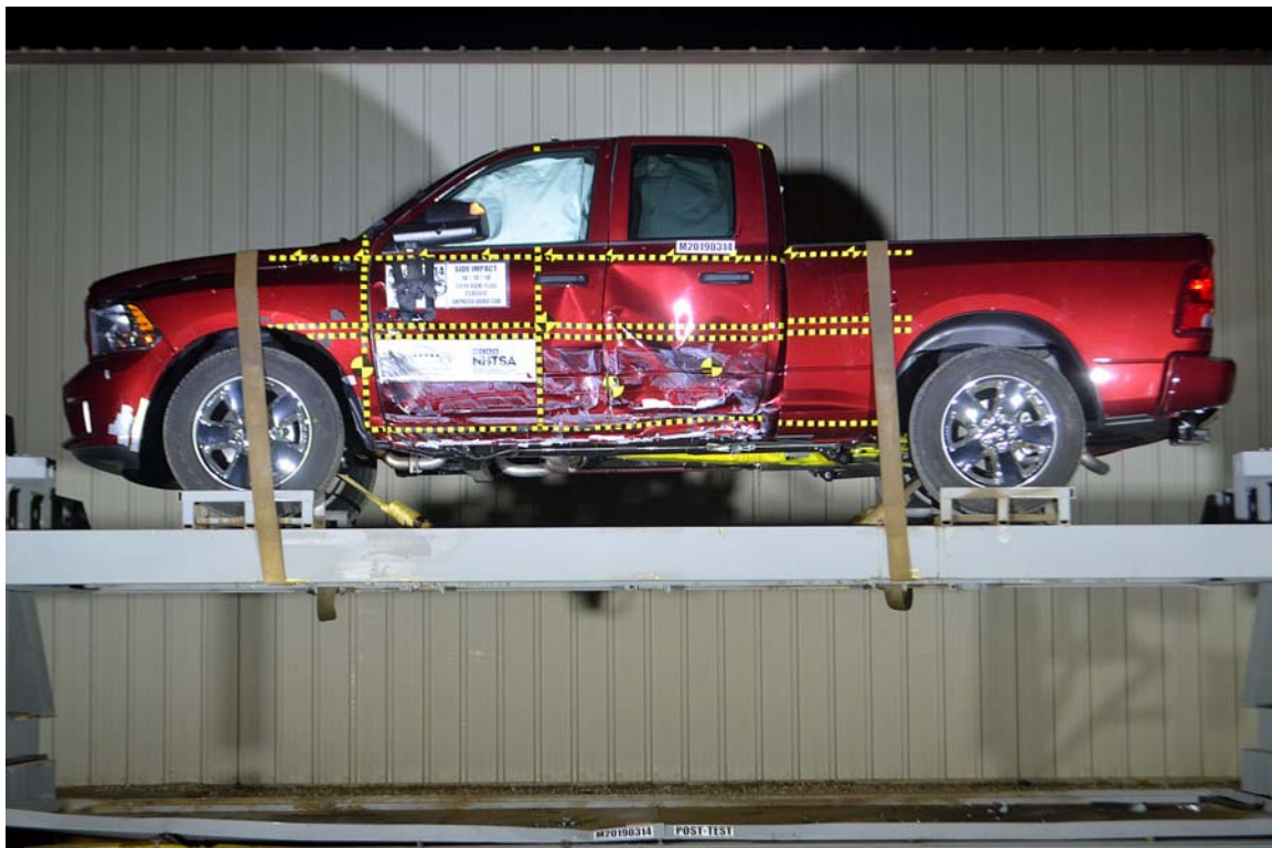
FIGURE 96. FMVSS No. 301 Static Rollover 0 Degrees
