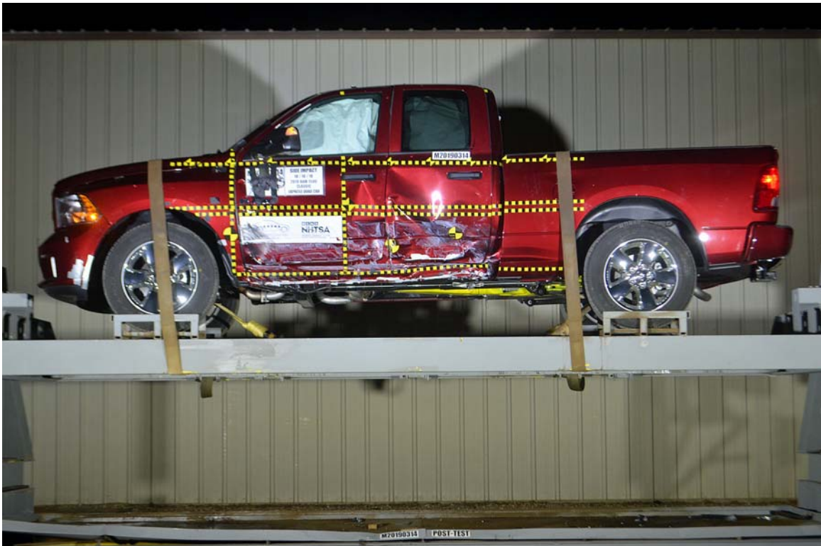
FIGURE 100. FMVSS No. 301 Static Rollover 360 Degrees
