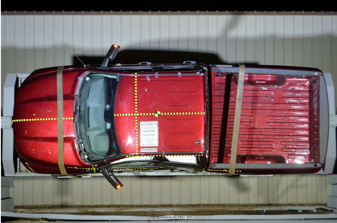
FIGURE 97. FMVSS No. 301 Static Rollover 90 Degrees
