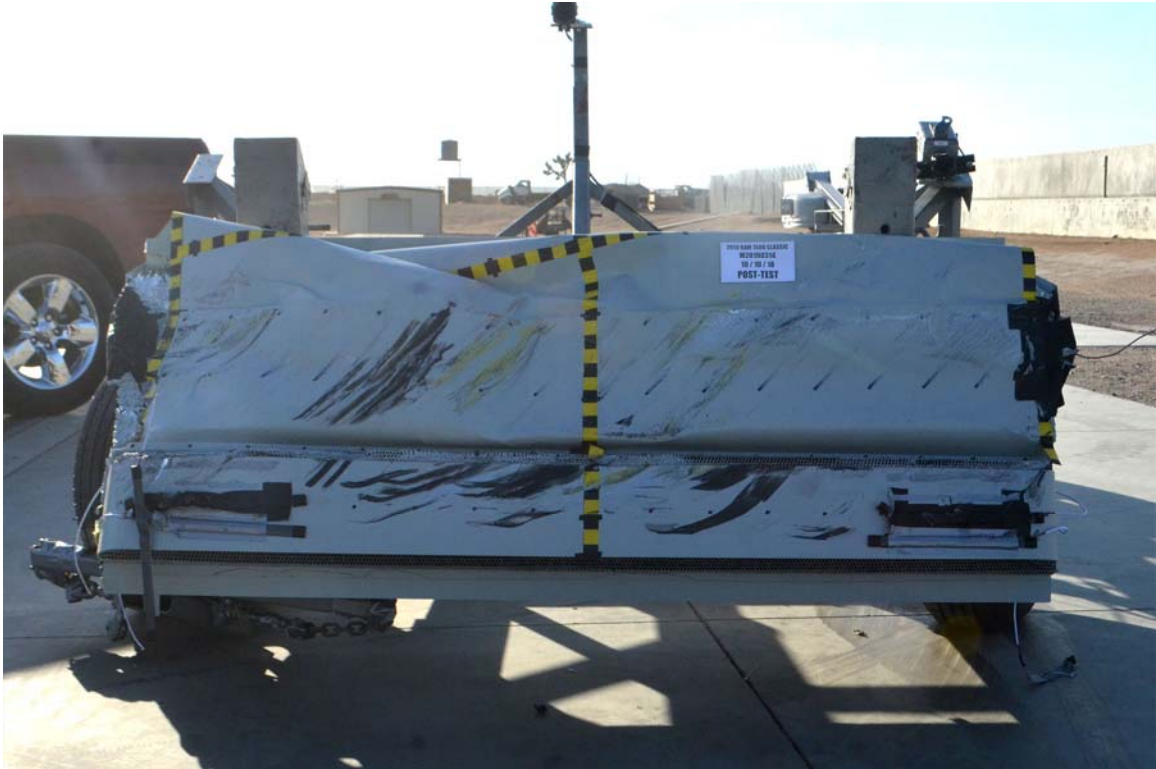
FIGURE 85. Post-Test Front View of MDB Impactor Face
