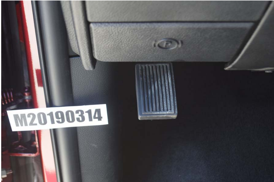
FIGURE 37. View of Disengaged Parking Brake
