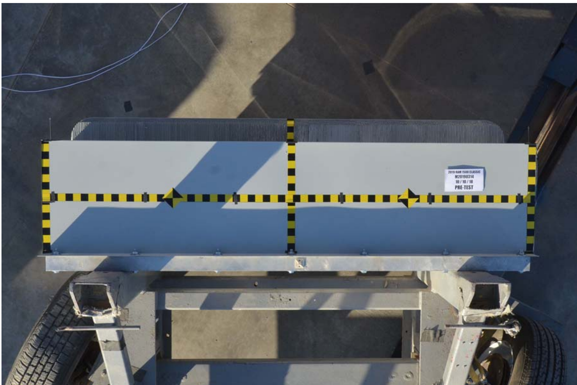
FIGURE 86. Pre-Test Top View of MDB Impactor Face
