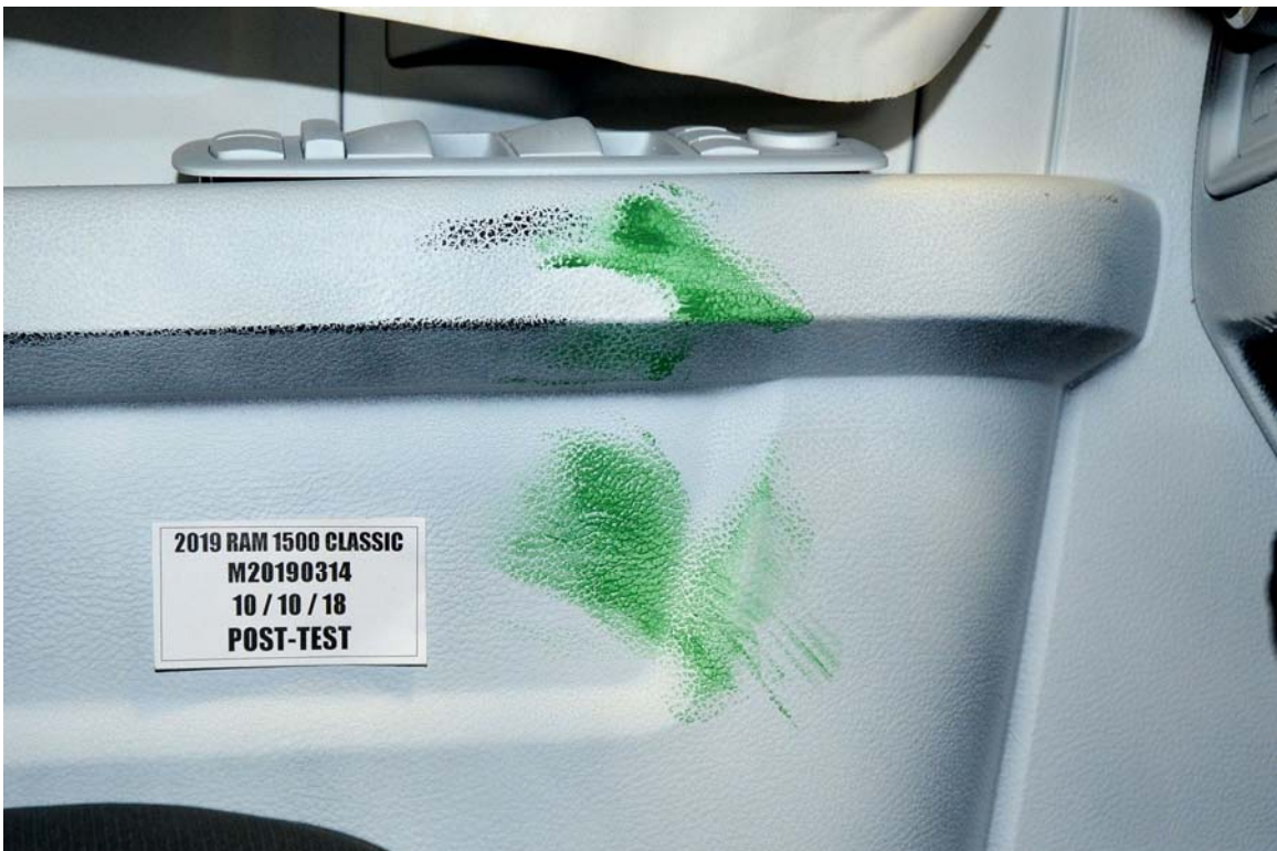
FIGURE 54. Post-Test Driver Dummy Close-Up Knee Contact View
