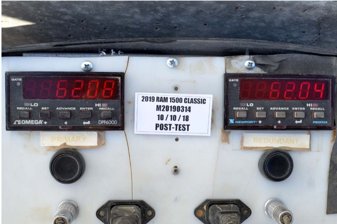
FIGURE 95. Post-Test Primary and Redundant Speed Trap Read-Out
