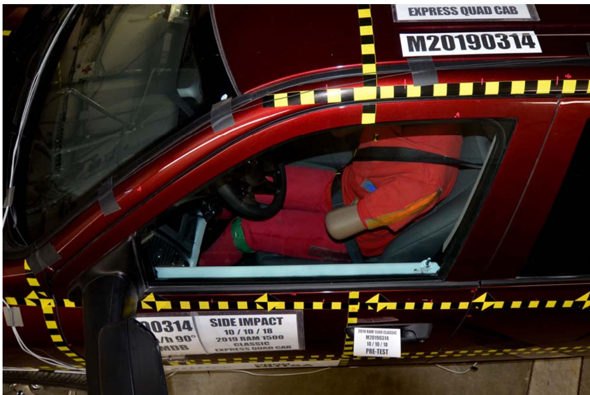
FIGURE 42. Pre-Test Driver Dummy and Door Clearance View
