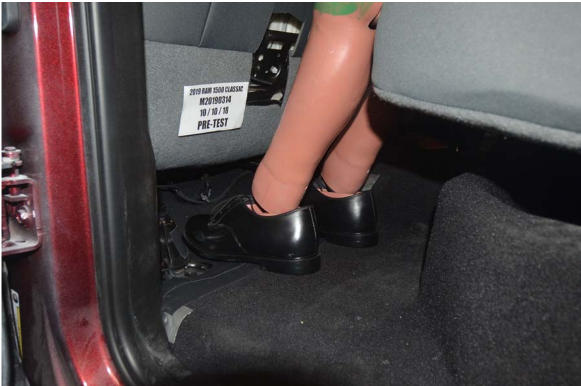
FIGURE 64. Pre-Test Placement of Rear Passenger Dummy's Feet
