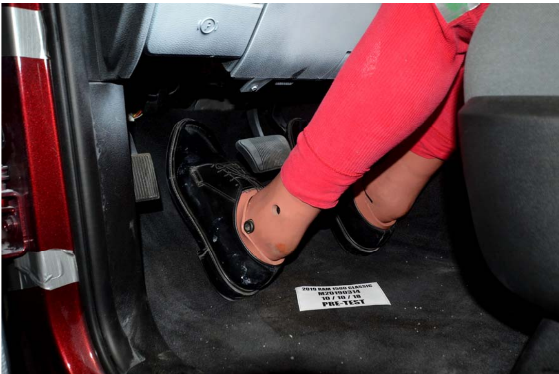
FIGURE 34. Pre-Test Placement of Driver Dummy's Feet
