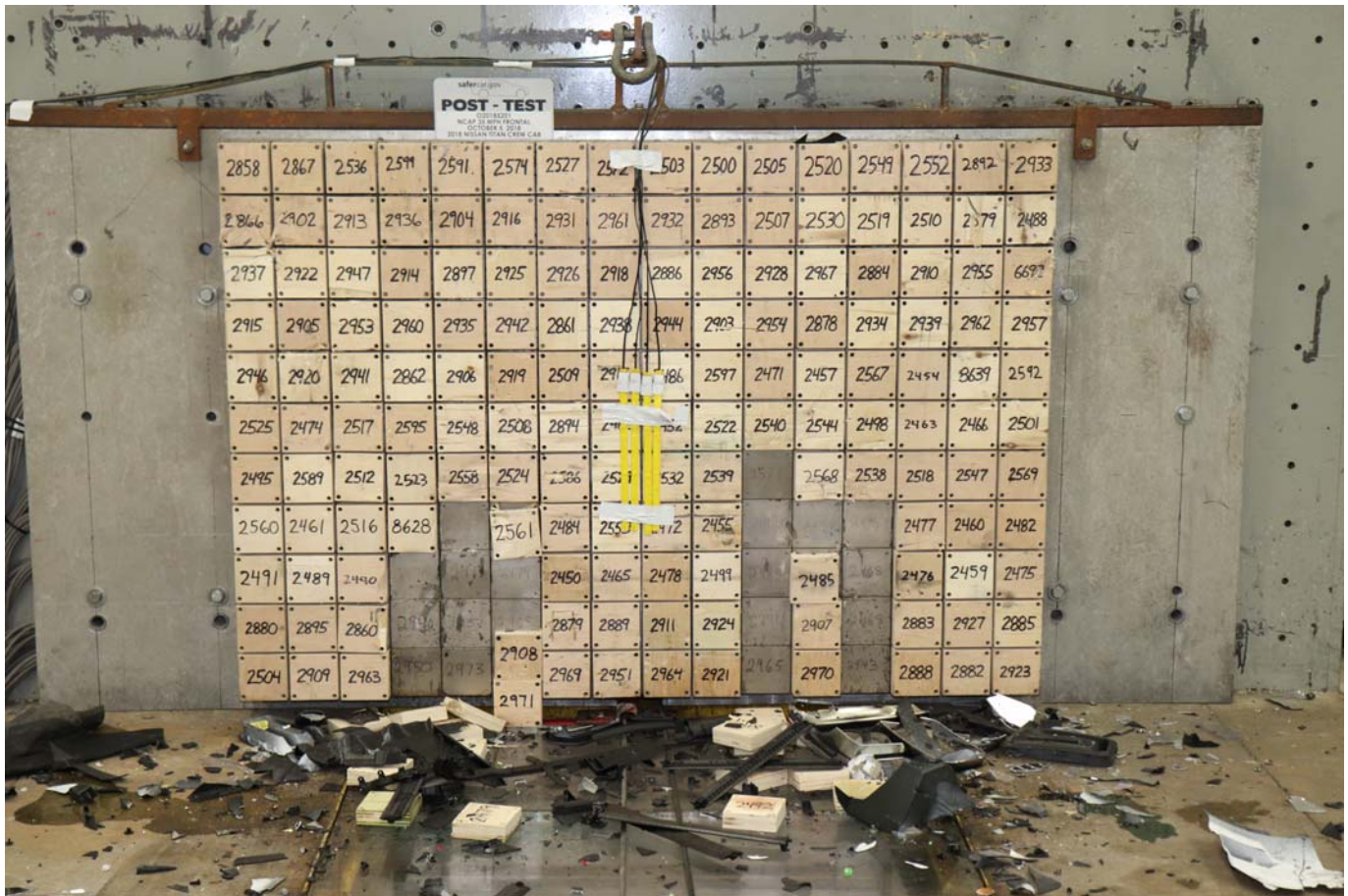
Photo No. 003 - Post-Test Load Cell Wall
