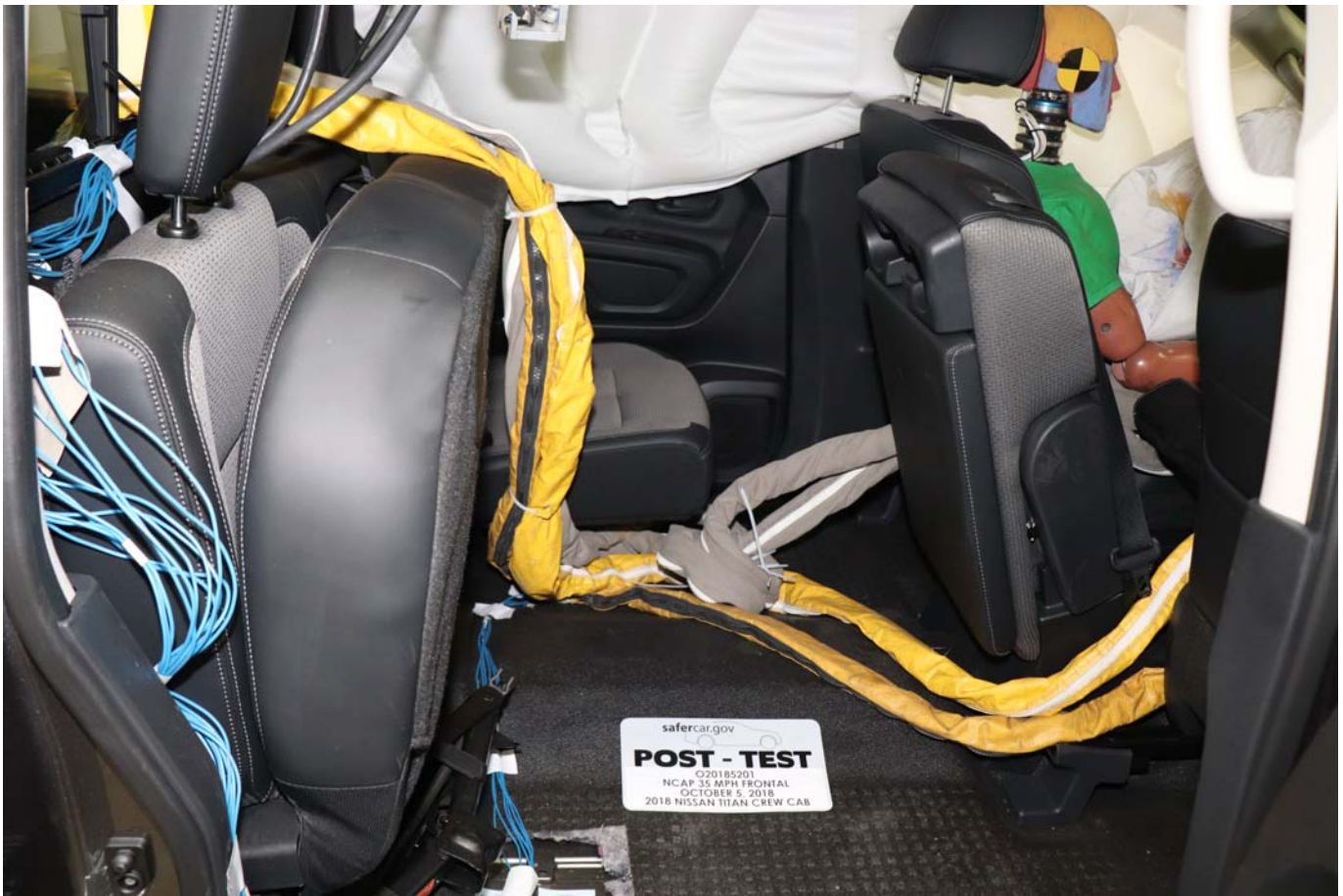
Photo No. 029 - Post-Test Dummy Cable Routing
