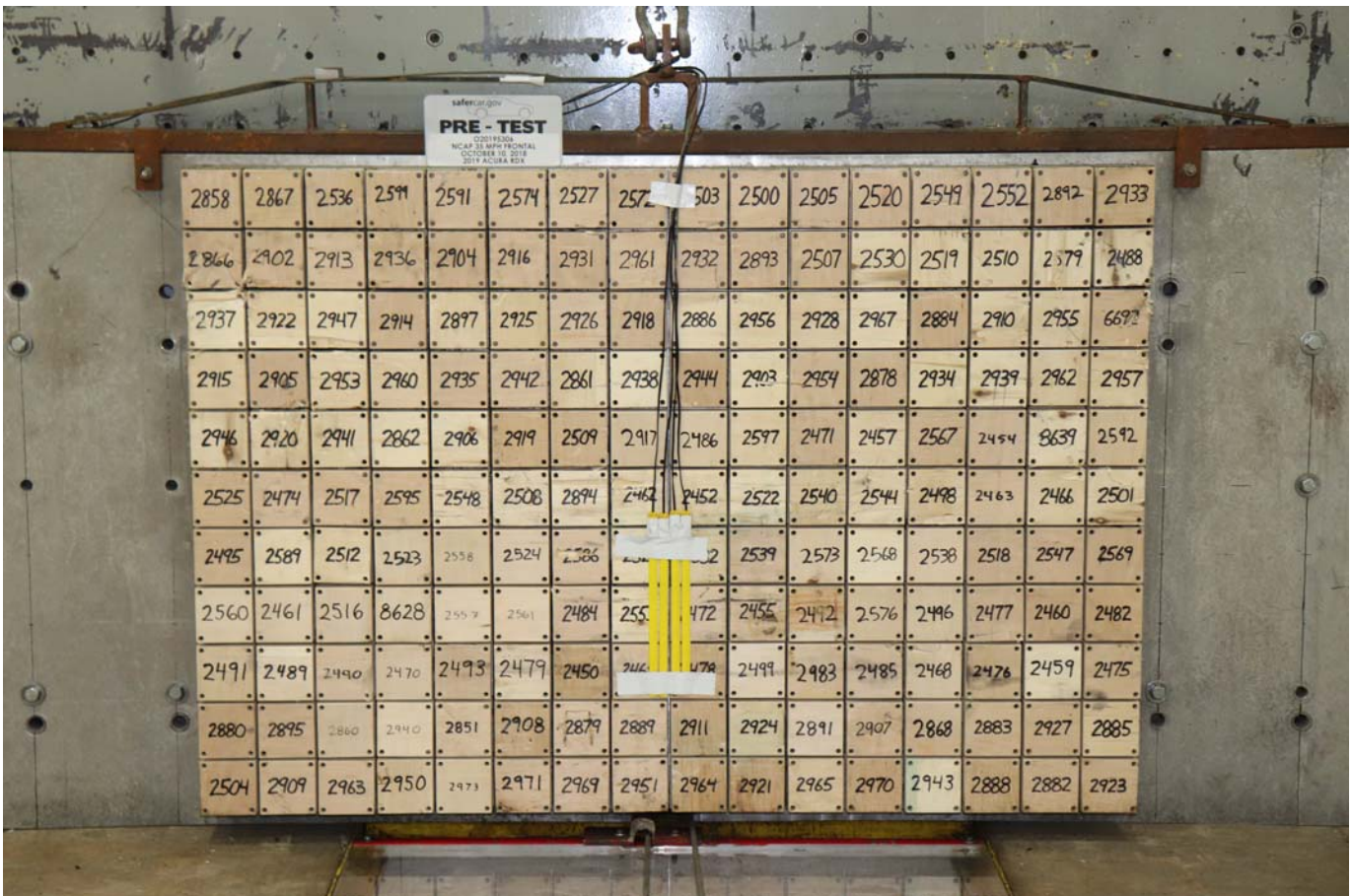
Photo No. 002 - Pre-Test Load Cell Wall
