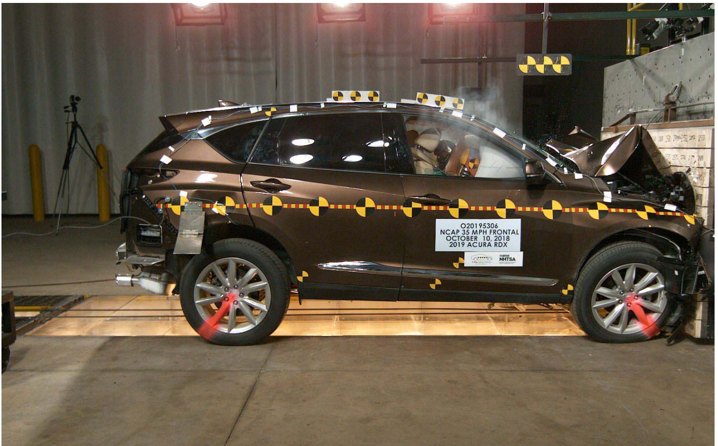
Photo No. 078 - 2019 Acura RDX AWD 5-Door SUV Frontal Impact Event
