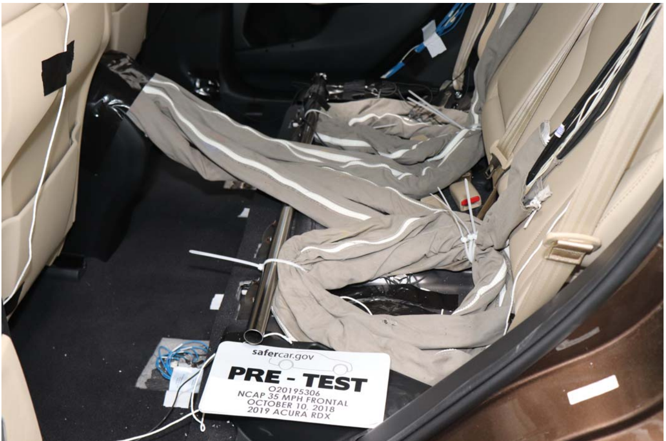
Photo No. 028 - Pre-Test Dummy Cable Routing
