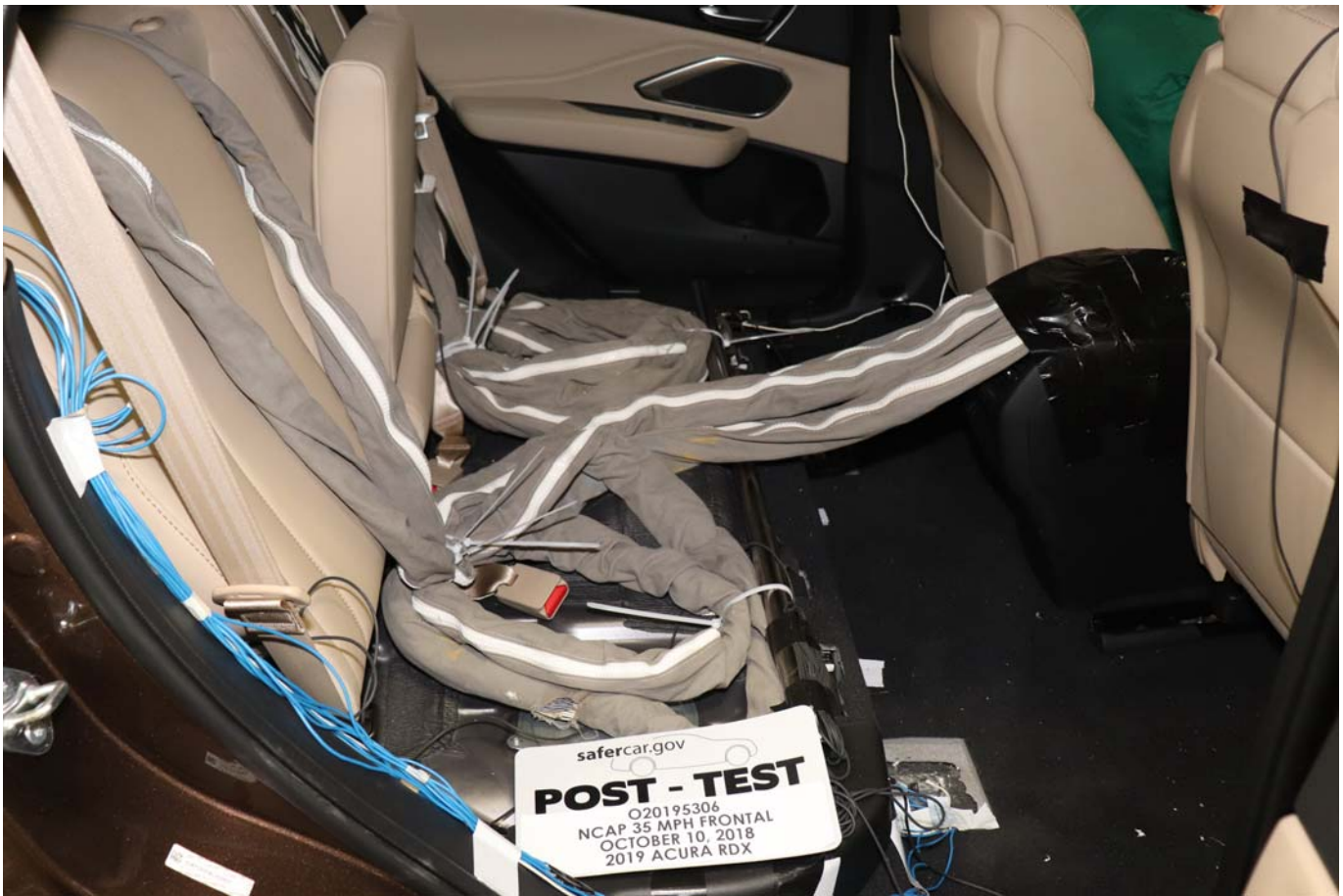
Photo No. 029 - Post-Test Dummy Cable Routing
