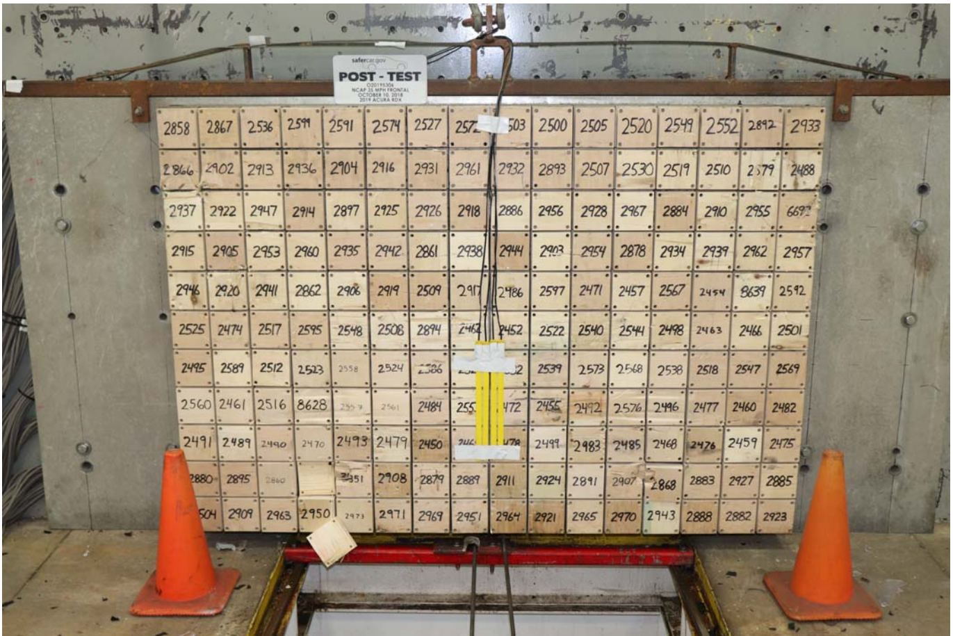
Photo No. 003 - Post-Test Load Cell Wall
