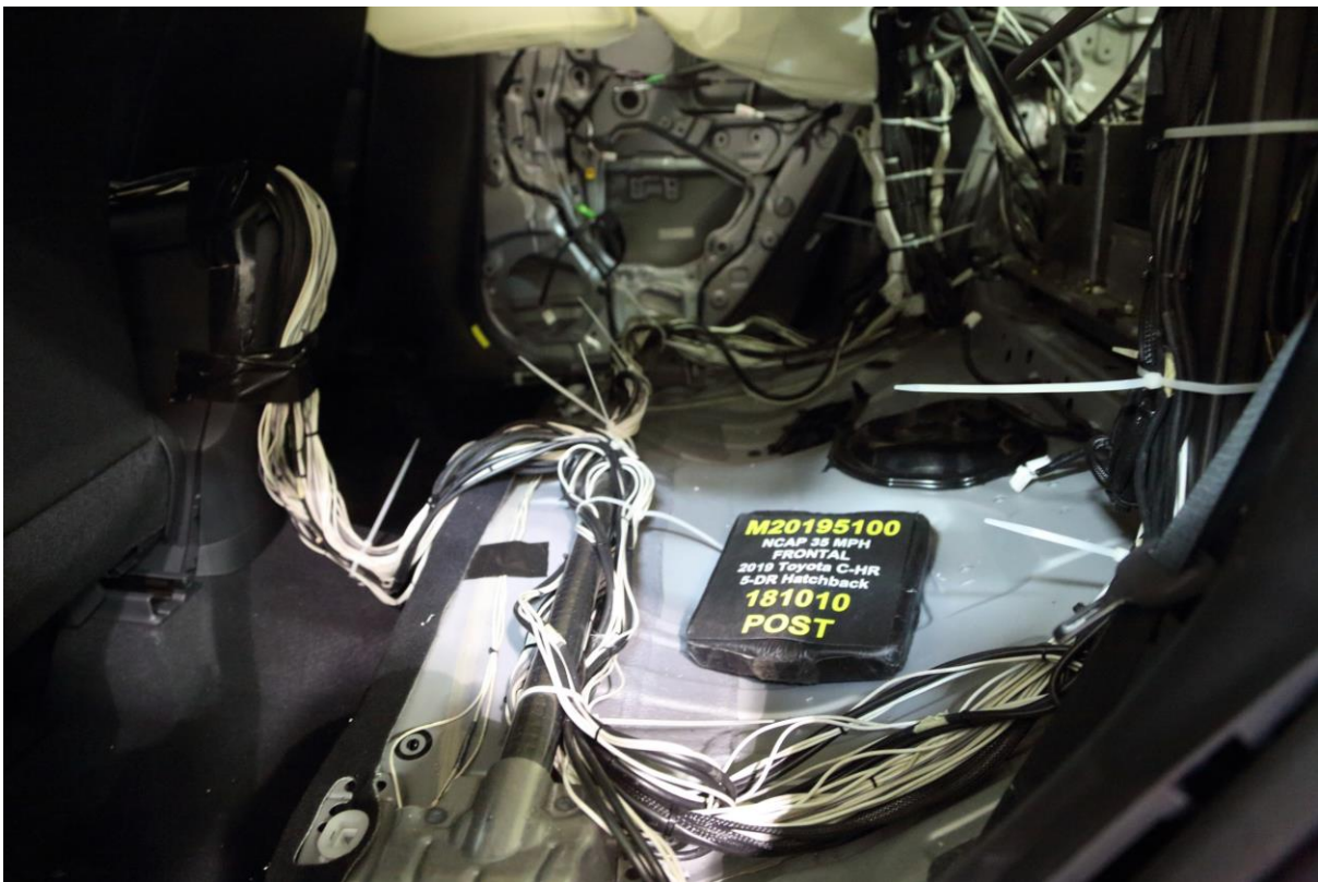
029 Post-Test Dummy Cable Routing
