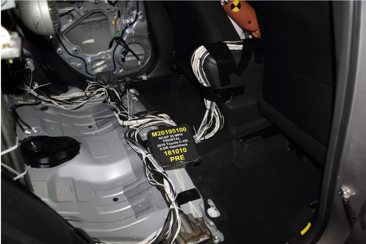
028 Pre-Test Dummy Cable Routing
