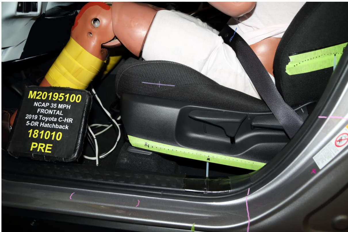
036 Pre-Test Driver's Seat Fore-Aft Markings
