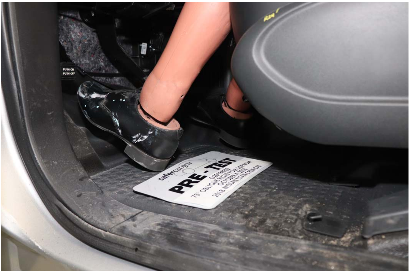
Photo No. 032 - Pre-Test Placement of Dummy Feet
