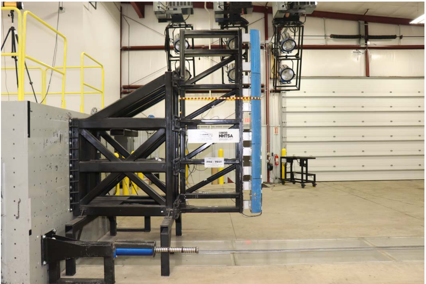
Photo No. 059 - Pre-Test Pole Barrier Side View
