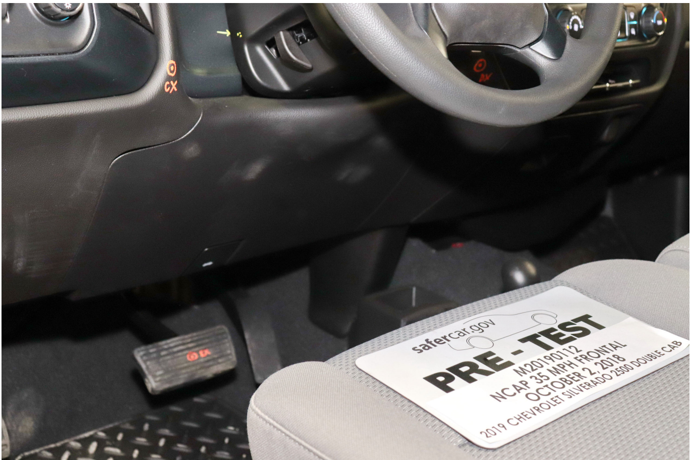
Photo No. 042 - Pre-Test Driver Side Knee Bolster
