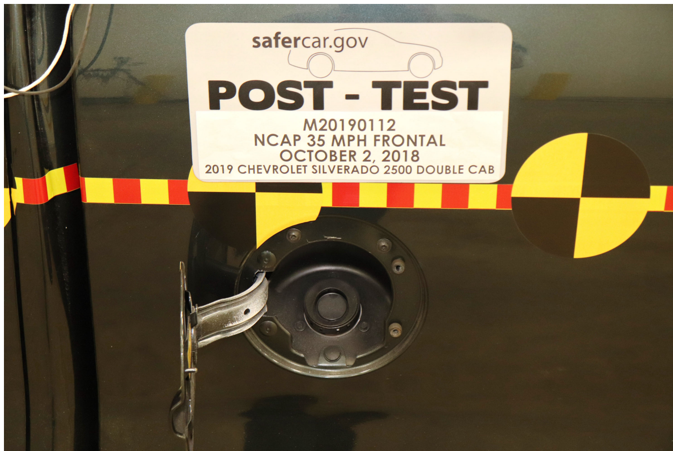
Photo No. 023 - Post-Test Fuel Filler Cap View
