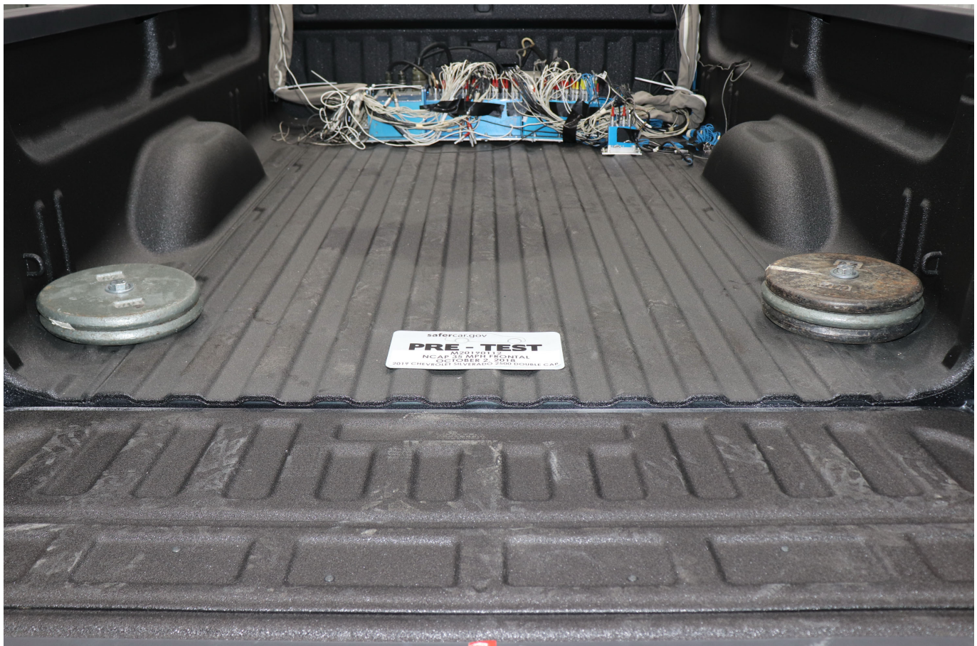
Photo No. 070 - Ballast Installed in Vehicle
