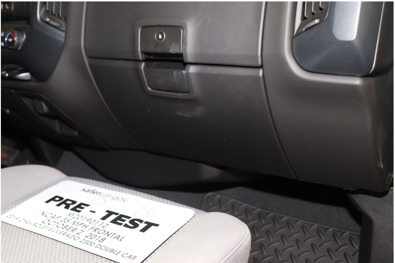
Photo No. 063 - Pre-Test Passenger Side Knee Bolster
