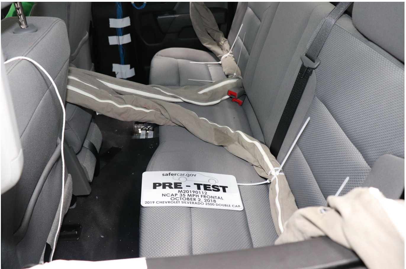
Photo No. 028 - Pre-Test Dummy Cable Routing
