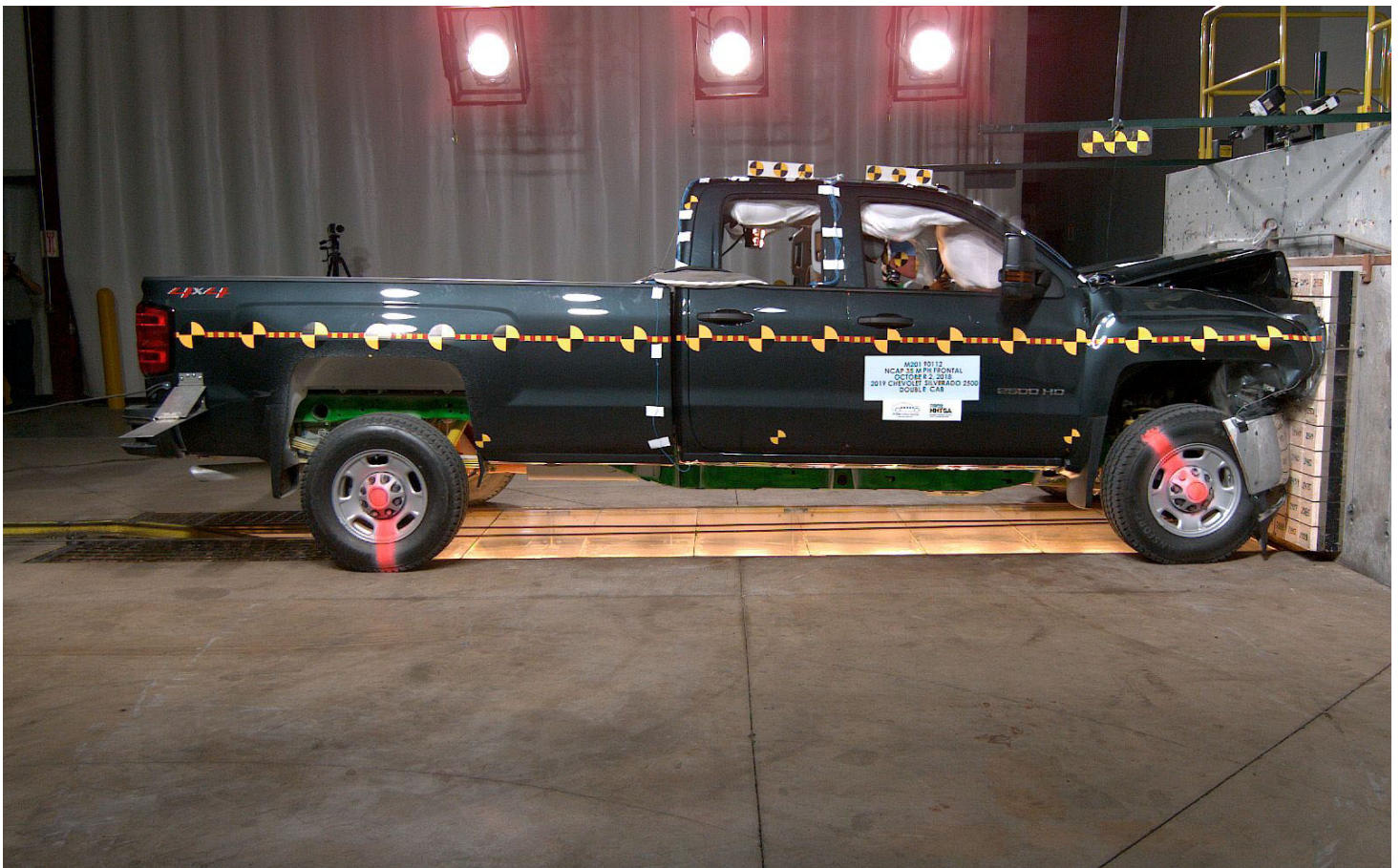
Photo No. 078 - 2019 Chevrolet Silverado 2500 Double Cab Frontal Impact Event
