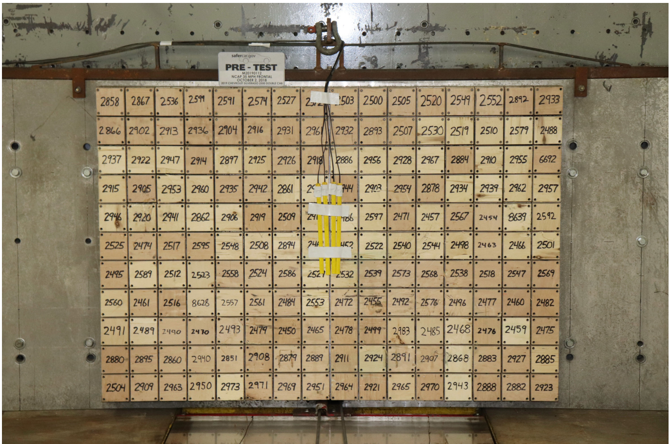
Photo No. 002 - Pre-Test Load Cell Wall
