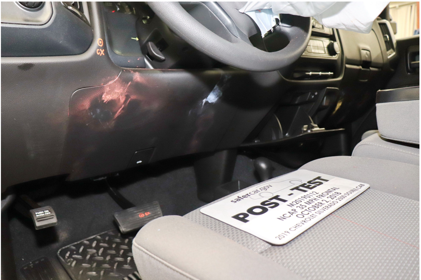
Photo No. 043 - Post-Test Driver Side Knee Bolster
