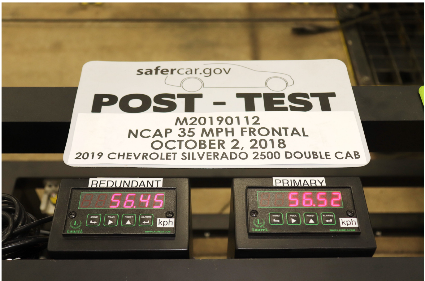
Photo No. 072 - Post-Test Speed Trap Read-Out
