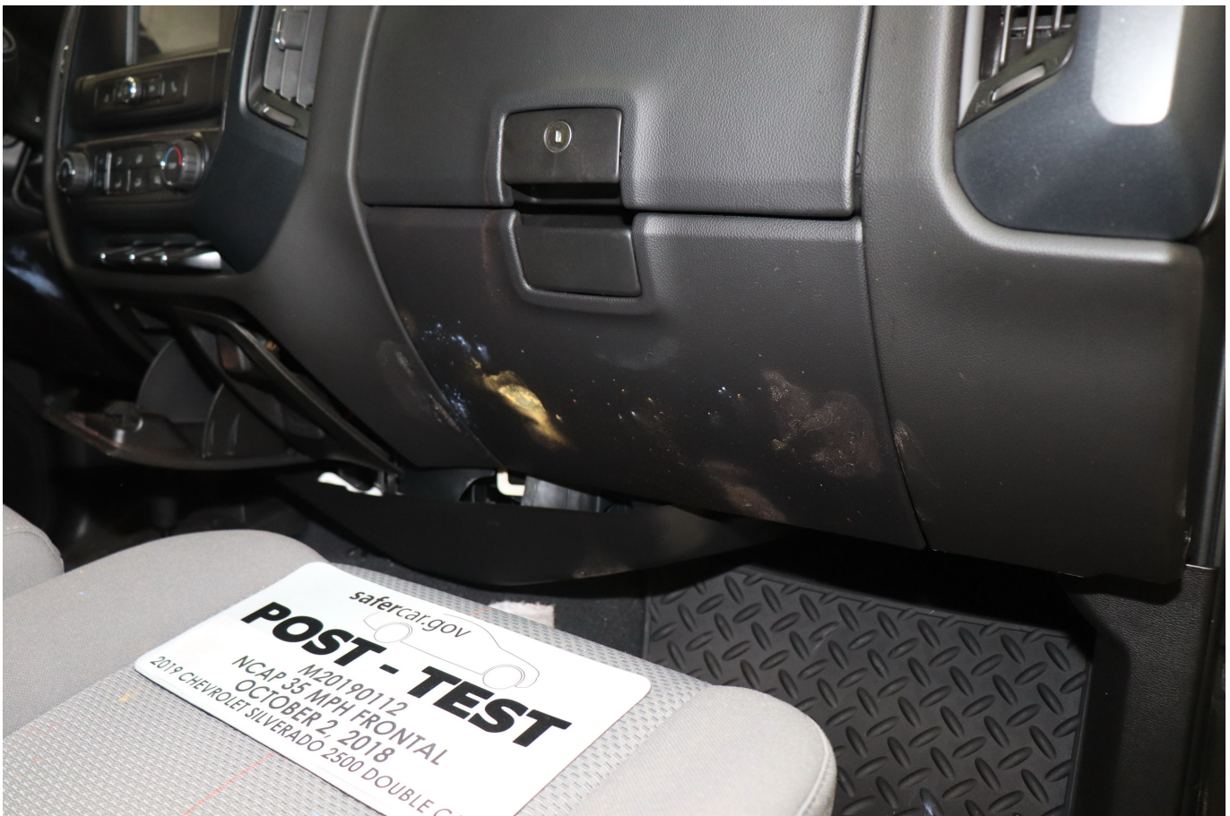
Photo No. 064 - Post-Test Passenger Side Knee Bolster
