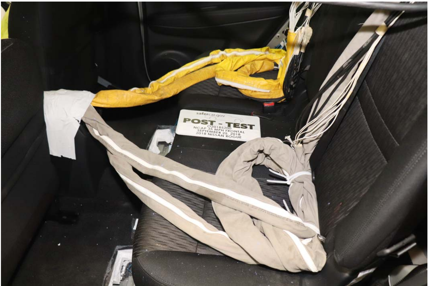
Photo No. 029 - Post-Test Dummy Cable Routing
