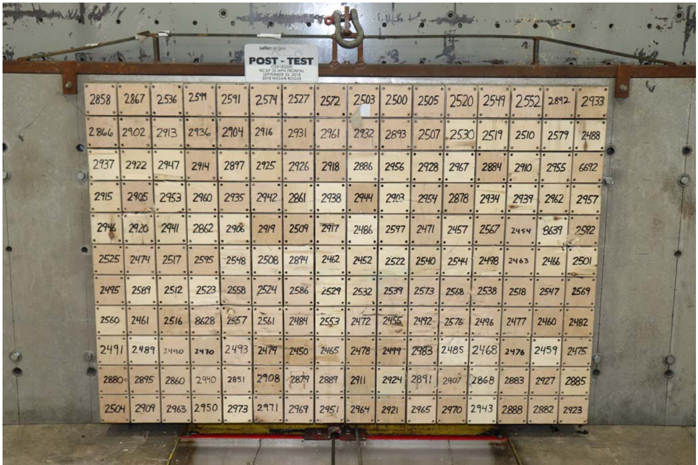
Photo No. 003 - Post-Test Load Cell Wall
