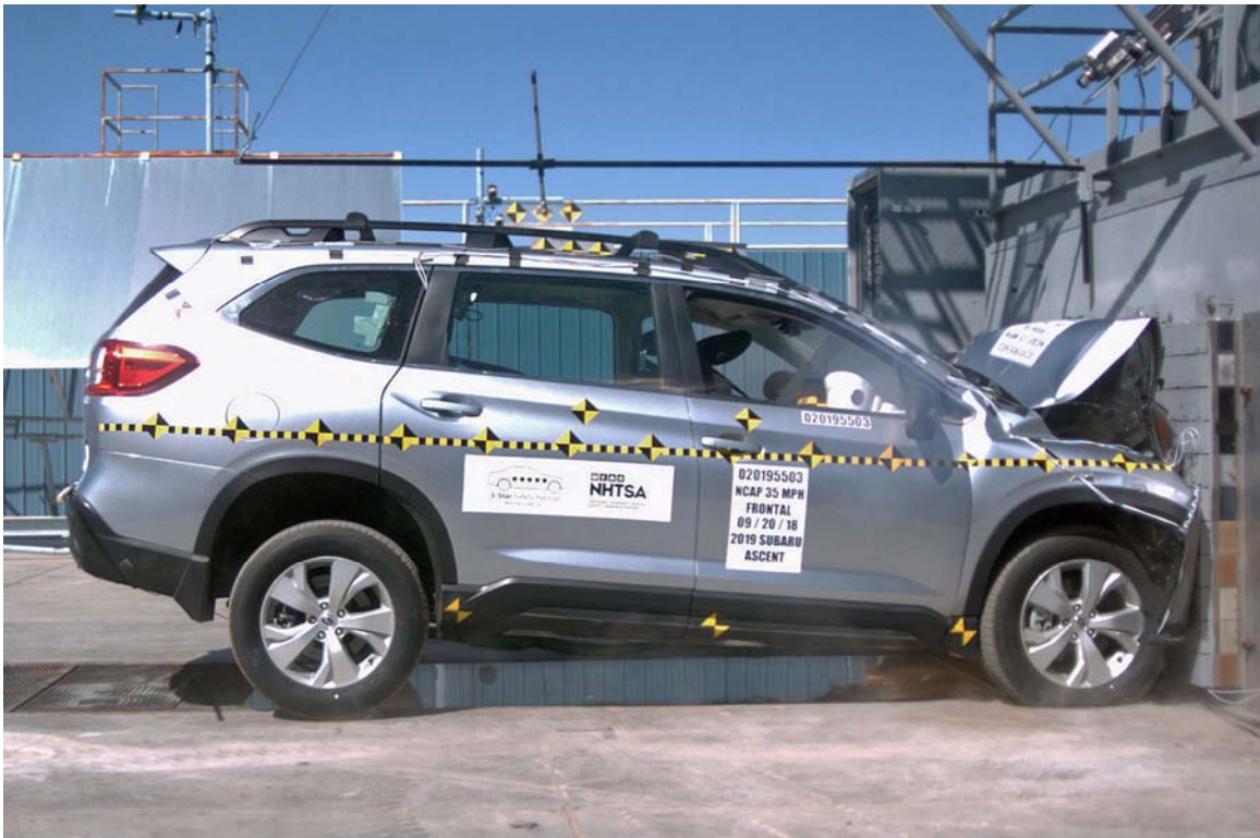
FIGURE 78. 2019 Subaru Ascent Frontal Impact Event
