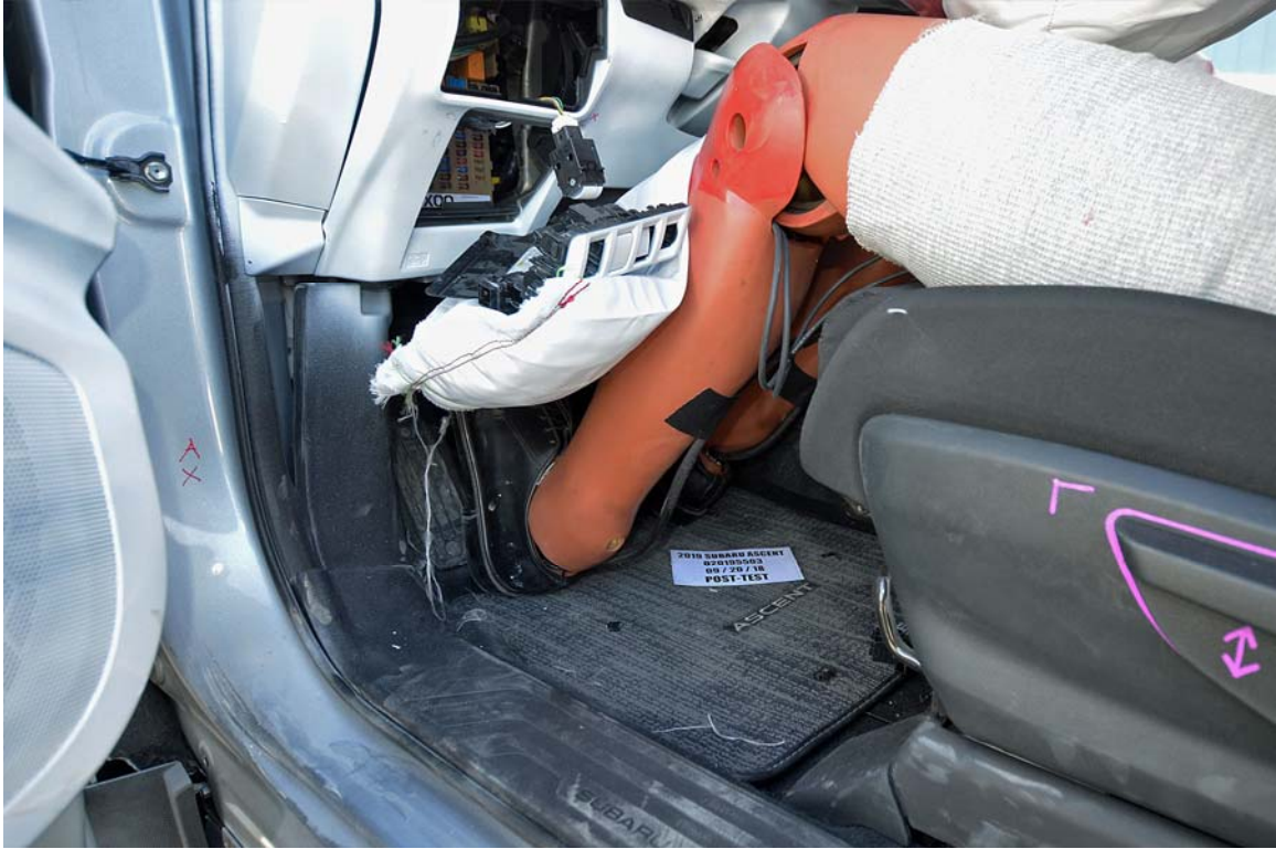
FIGURE 41. Post-Test Driver Dummy Feet
