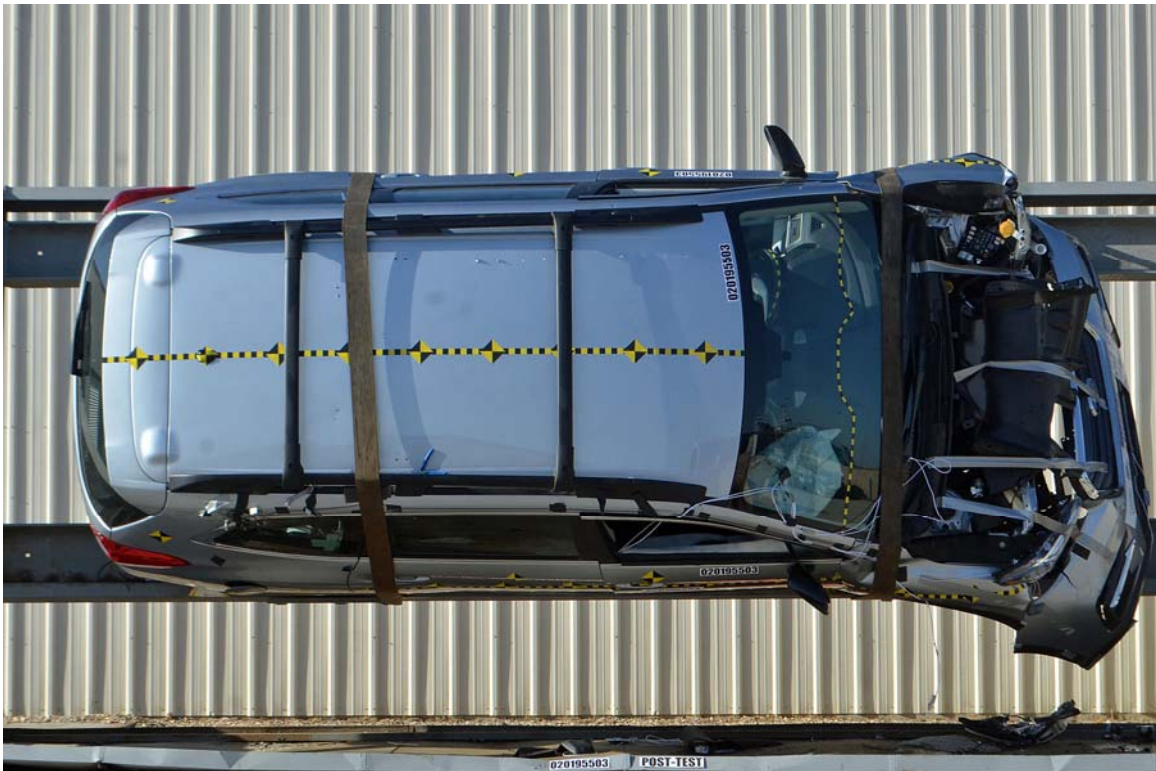
FIGURE 74. Vehicle at 90° on Static Rollover Device
