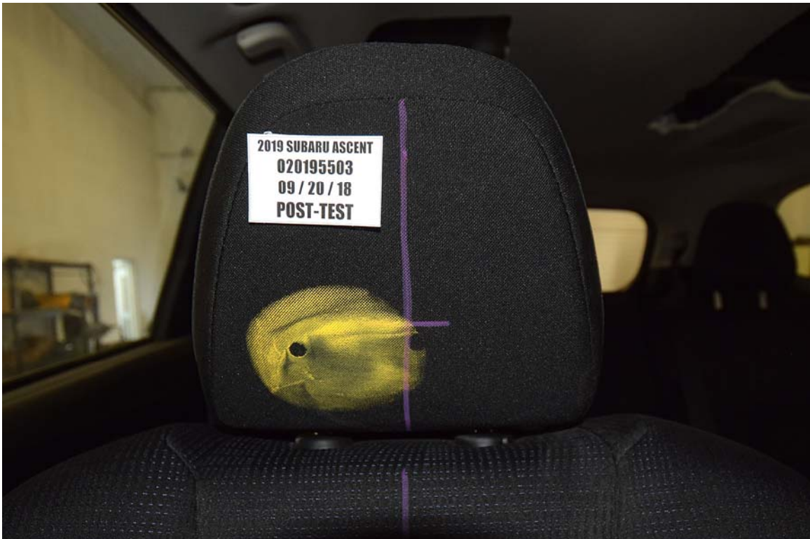
FIGURE 69. Post-Test Passenger Dummy Contact with Headrest
