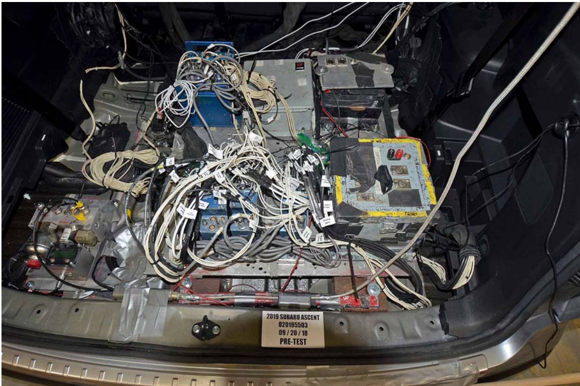
FIGURE 70. Photograph of Ballast Installed in Vehicle
