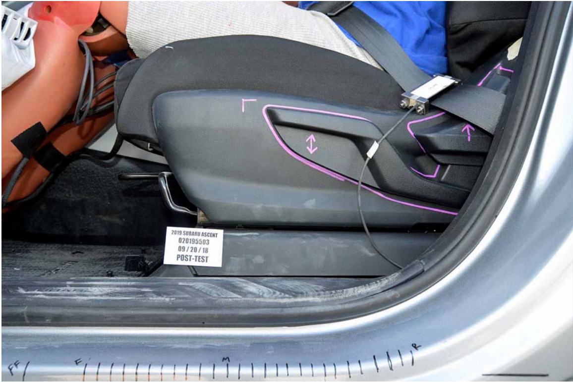
FIGURE 37. Post-Test Driver's Seat Fore-Aft Markings
