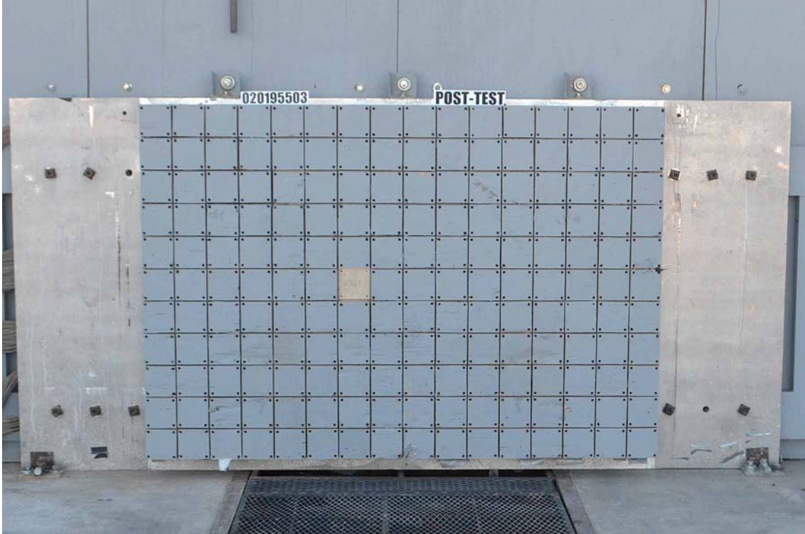
FIGURE 3. Post-Test Load Cell Wall
