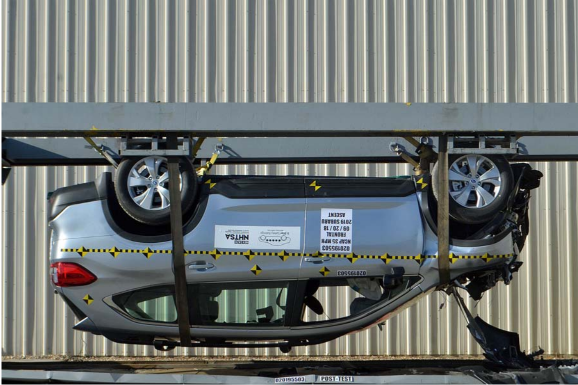
FIGURE 75. Vehicle at 180° on Static Rollover Device
