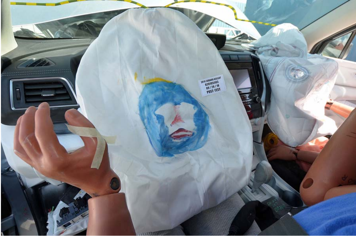
FIGURE 47. Post-Test Driver Dummy Contact with Airbag
