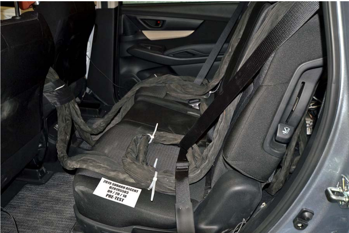
FIGURE 28. Pre-Test Dummy Cable Routing
