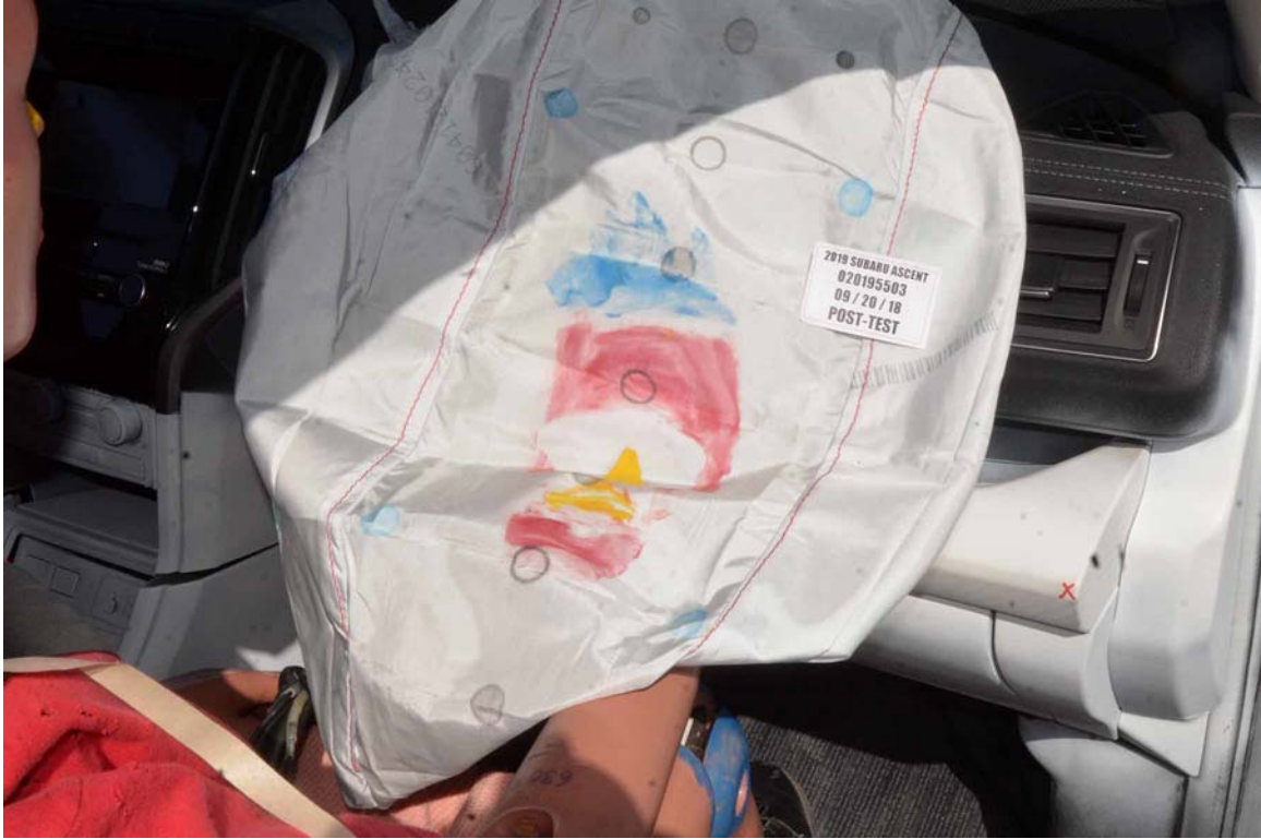
FIGURE 68. Post-Test Passenger Dummy Contact with Airbag
