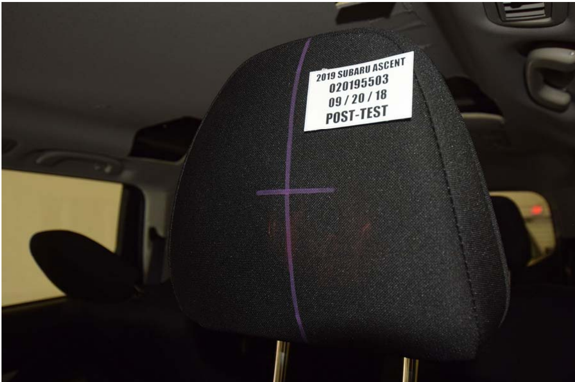
FIGURE 48. Post-Test Driver Dummy Contact with Headrest
