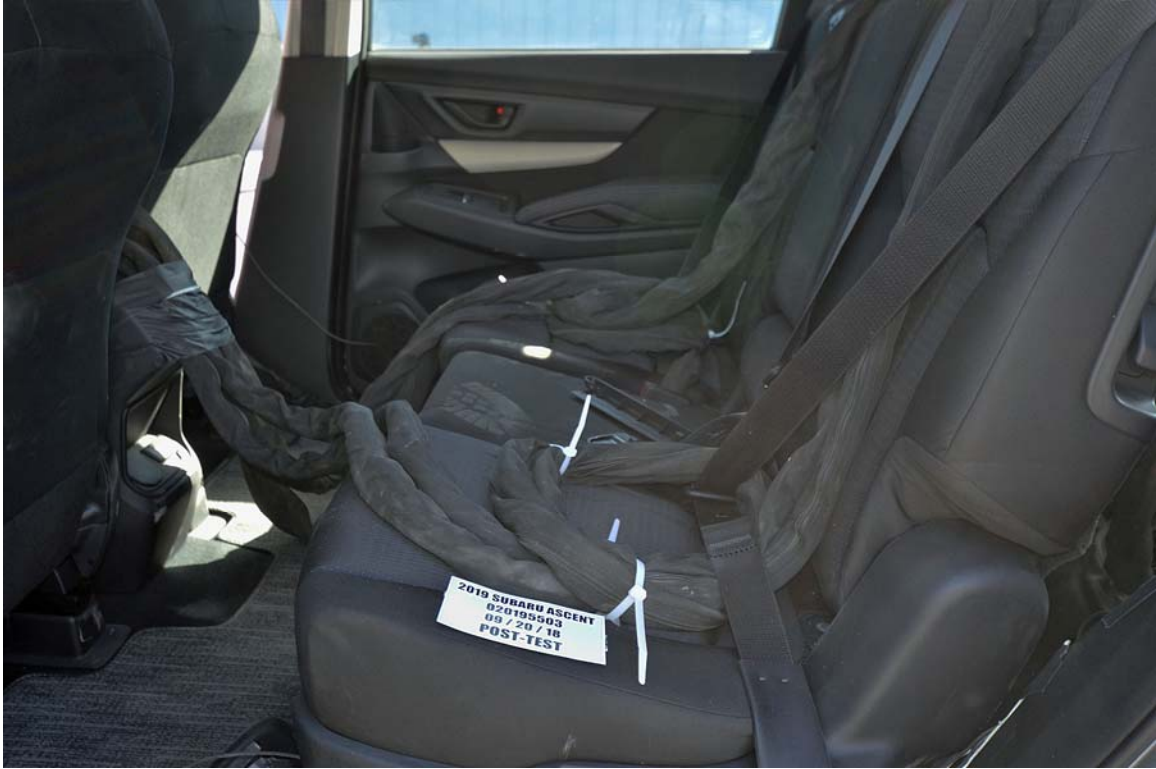
FIGURE 29. Post-Test Dummy Cable Routing
