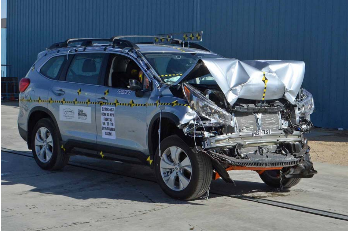
FIGURE 15. Post-Test Right Front \frac{3}{4} View
