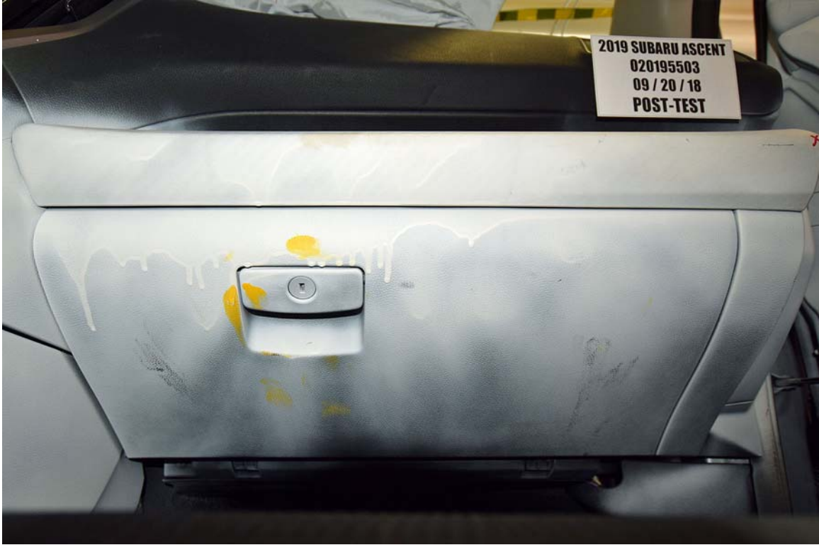
FIGURE 64. Post-Test Passenger's Side Knee Bolster
