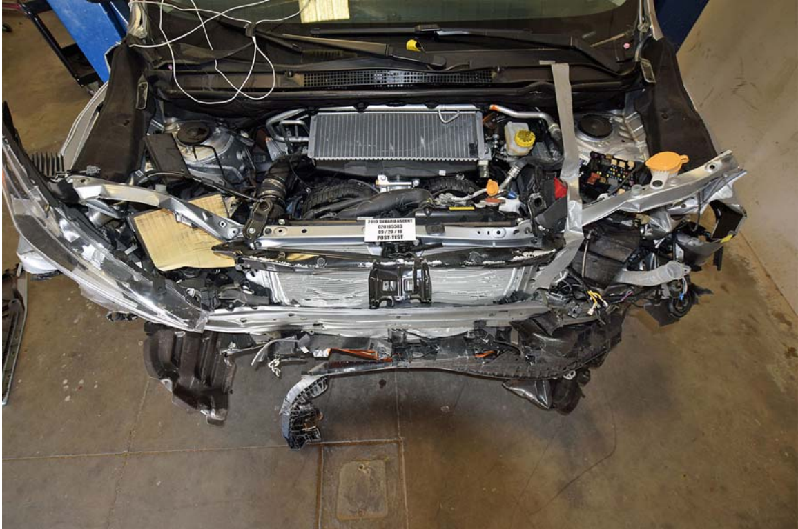
FIGURE 21. Post-Test Engine Compartment View
