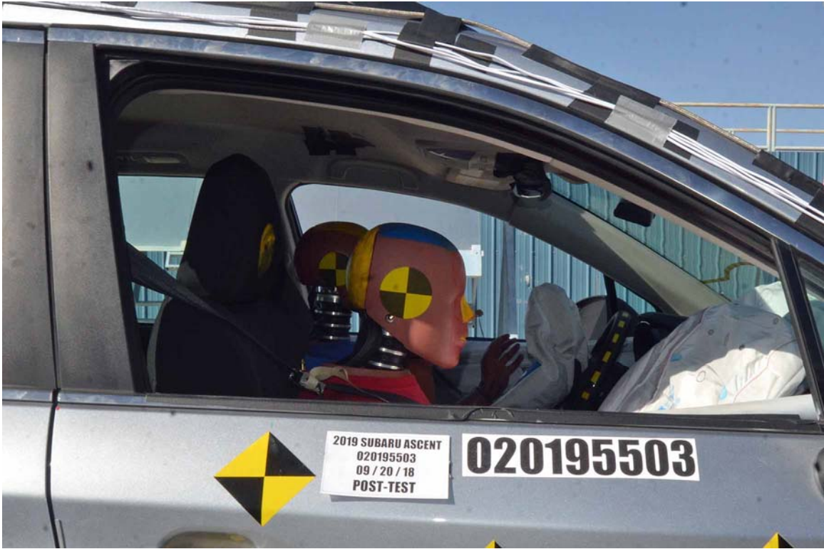
FIGURE 54. Post-Test Passenger Dummy Window View
