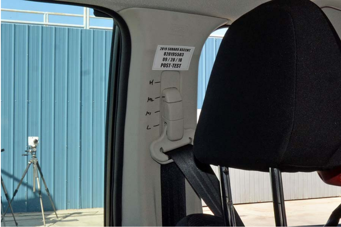
FIGURE 39. Post-Test View of Belt Anchorage for Driver Dummy
