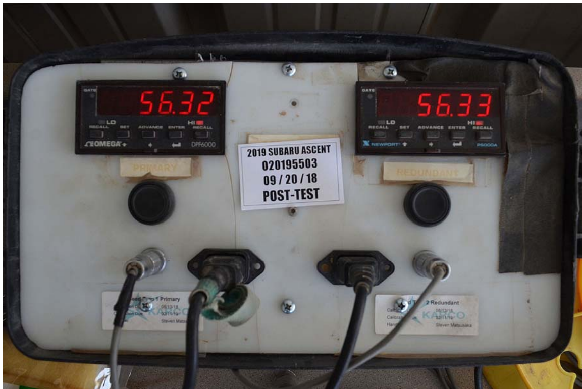
FIGURE 72. Post-Test Speed Trap Read-Out
