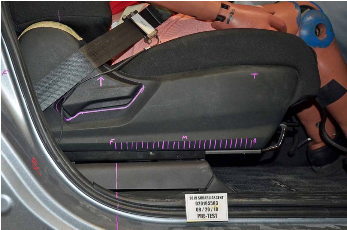
FIGURE 57. Pre-Test Passenger's Seat Fore-Aft Markings
