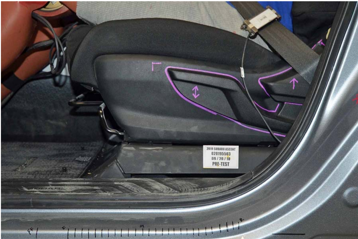
FIGURE 36. Pre-Test Driver's Seat Fore-Aft Markings
