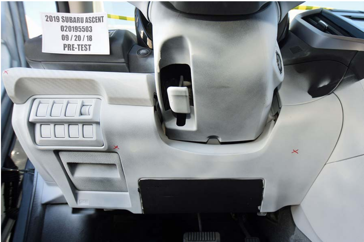
FIGURE 42. Pre-Test Driver's Side Knee Bolster
