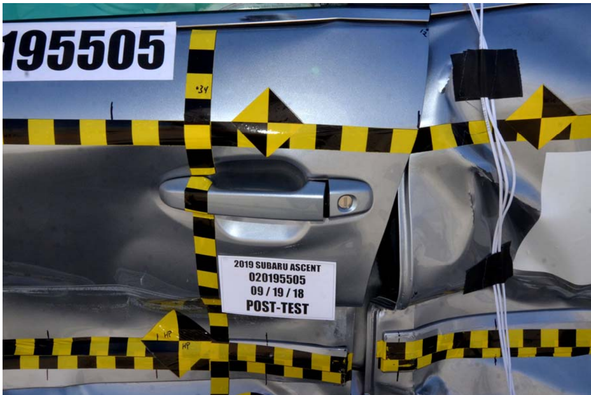
FIGURE 22. Post-Test Left Front Door Latch Close-Up
