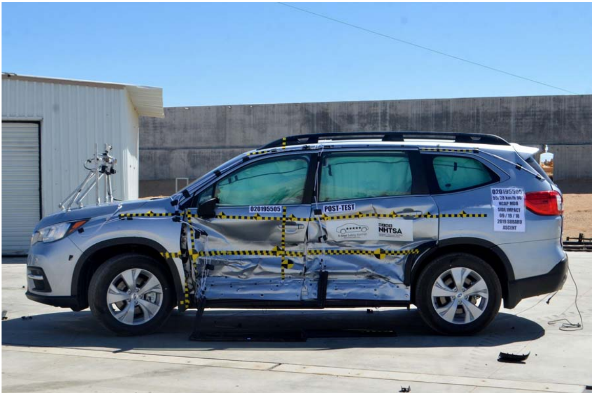
FIGURE 8. Post-Test Left Side View of Test Vehicle
