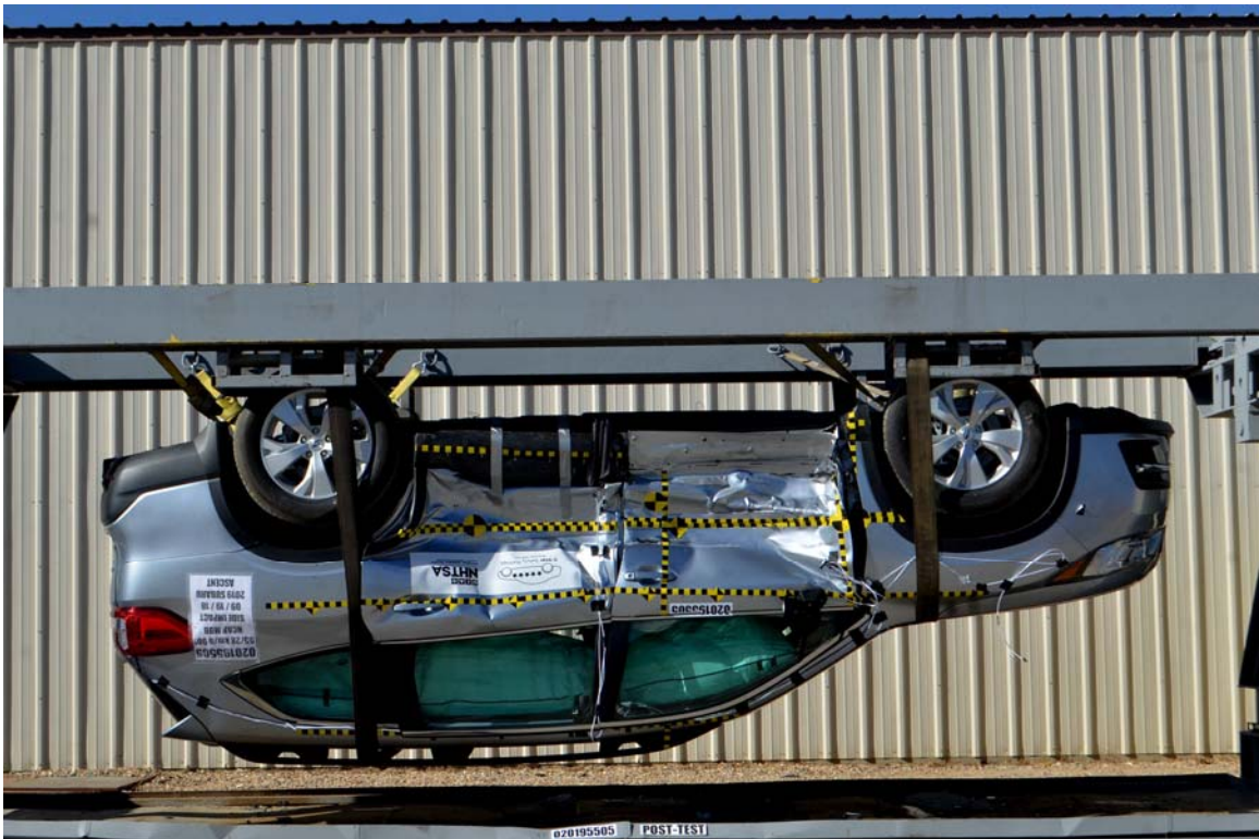
FIGURE 98. FMVSS No. 301 Static Rollover 180 Degrees
