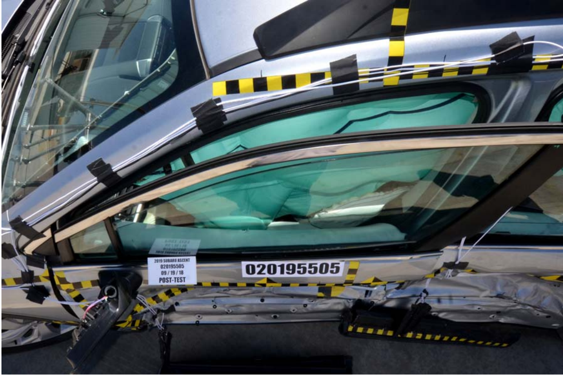
FIGURE 43. Post-Test Driver Dummy and Door Clearance View
