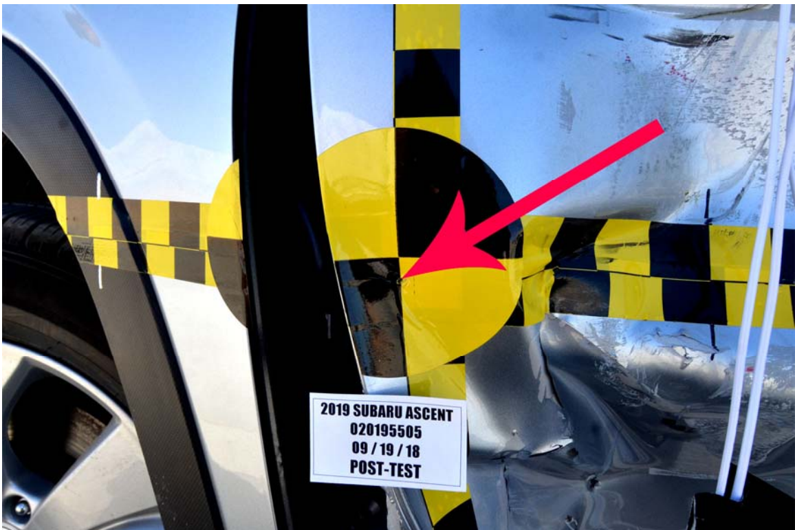
FIGURE 20. Post-Test Close-Up View of Impact Point Target
