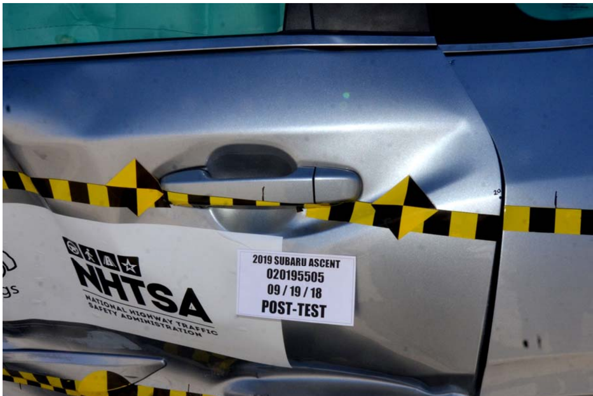
FIGURE 24. Post-Test Left Rear Door Latch Close-Up
