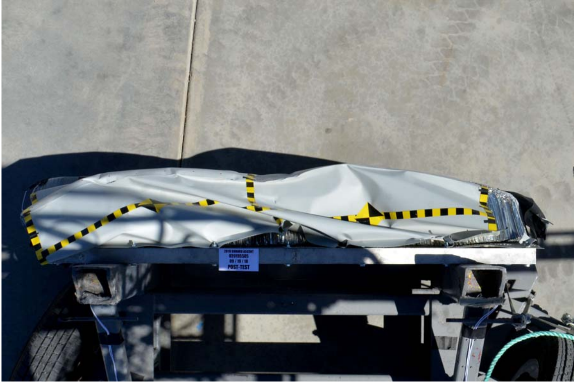
FIGURE 87. Post-Test Top View of MDB Impactor Face
