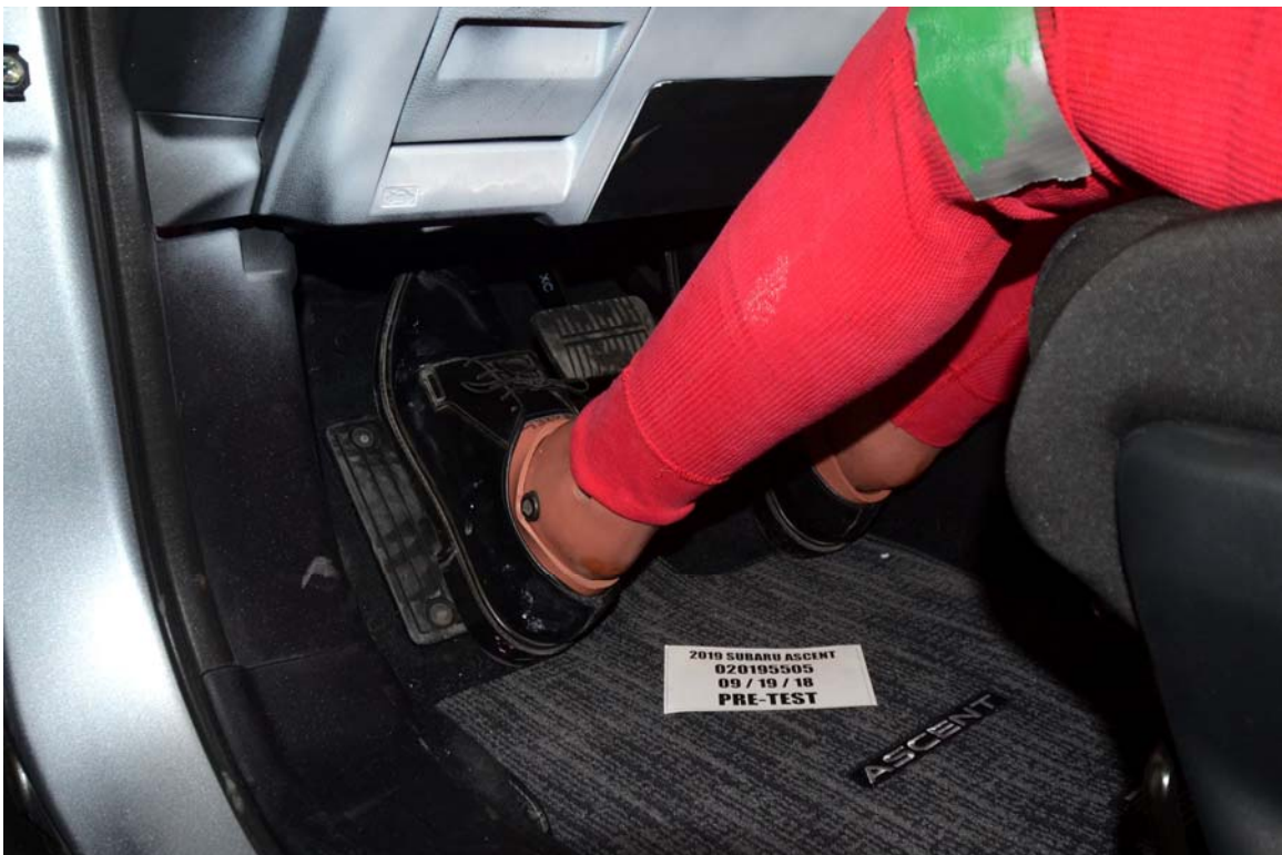
FIGURE 34. Pre-Test Placement of Driver Dummy's Feet
