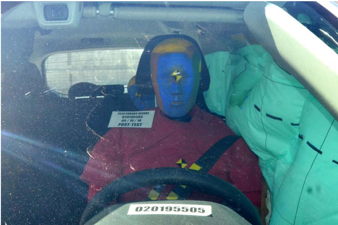
FIGURE 26. Post-Test Front Close-Up View of Driver Dummy
