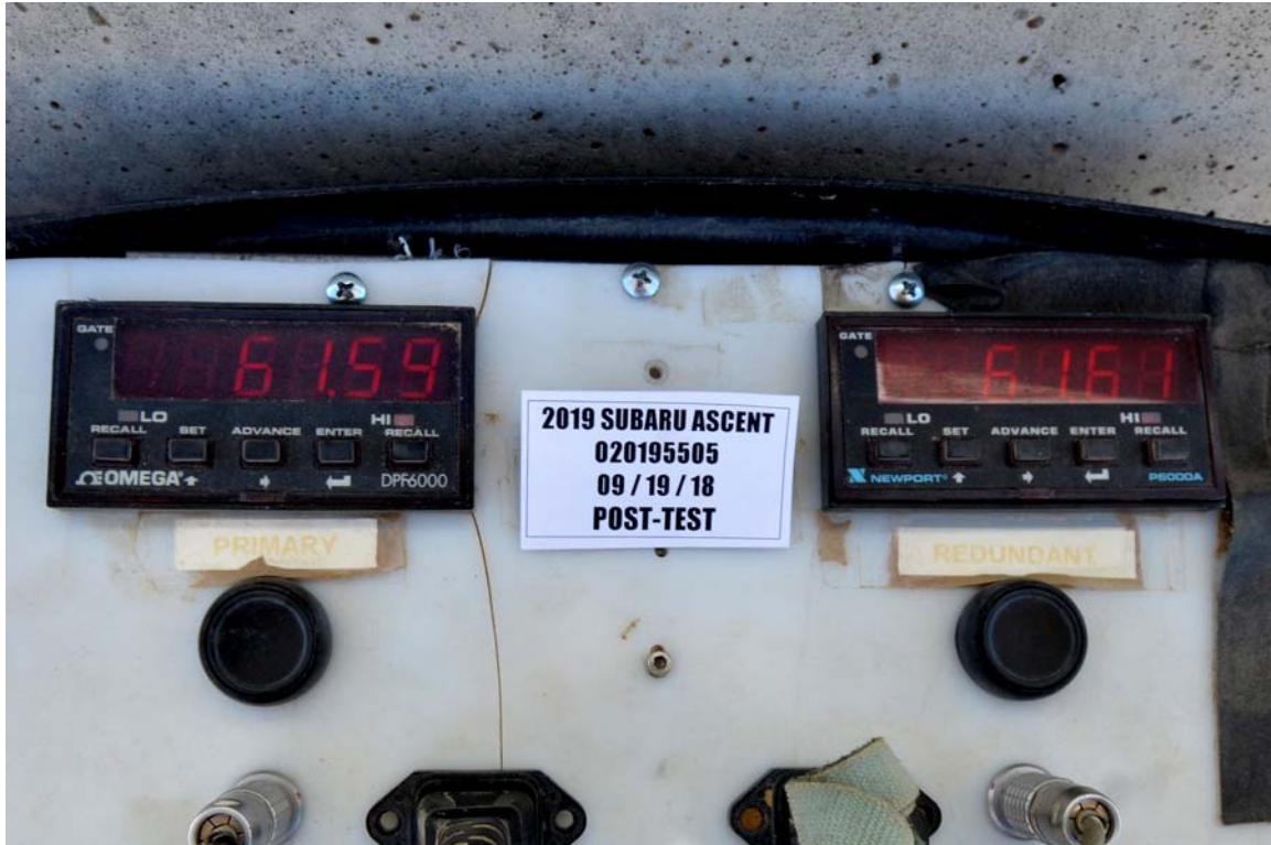
FIGURE 95. Post-Test Primary and Redundant Speed Trap Read-Out
