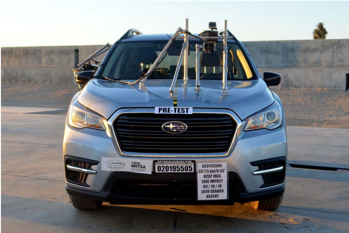
FIGURE 3. Pre-Test Frontal View of Test Vehicle
