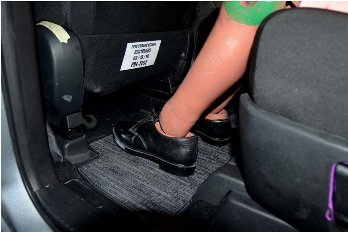
FIGURE 64. Pre-Test Placement of Rear Passenger Dummy's Feet
