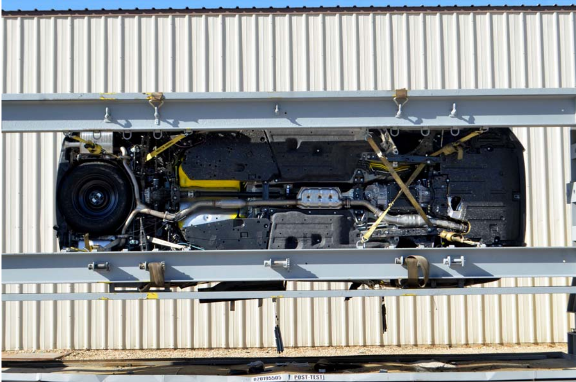
FIGURE 99. FMVSS No. 301 Static Rollover 270 Degrees
