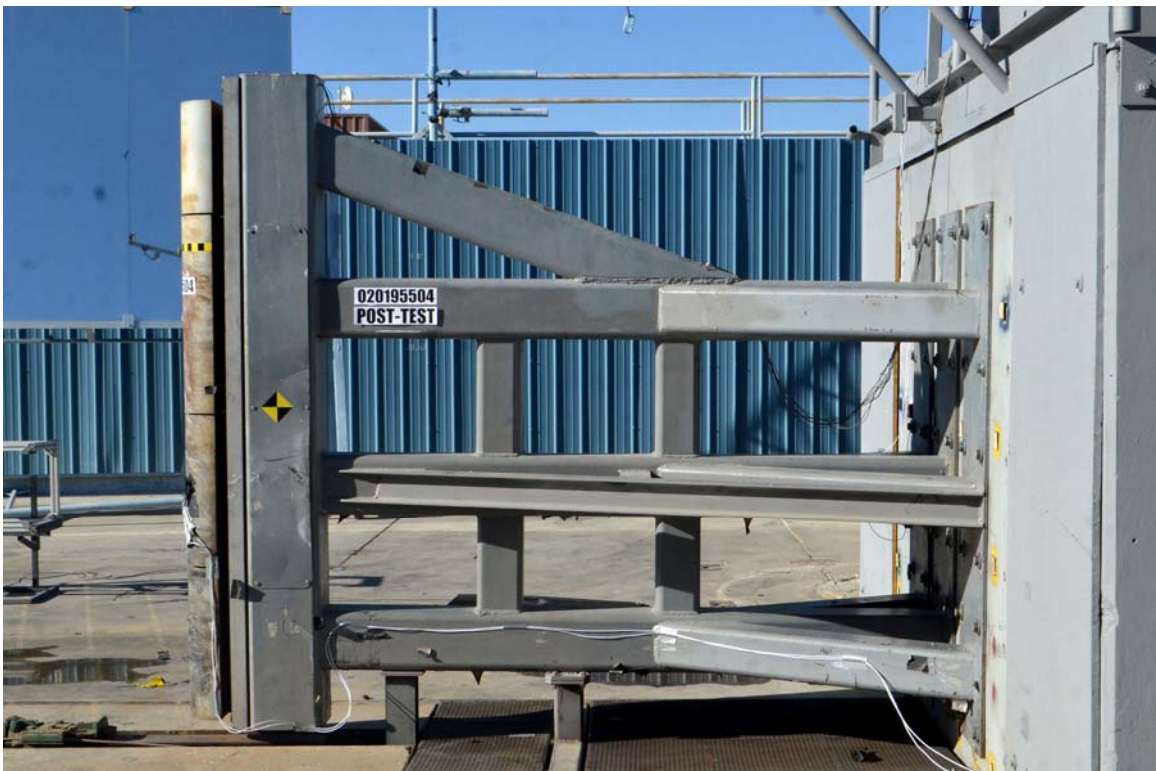
FIGURE 60. Post-Test Pole Barrier Side View
