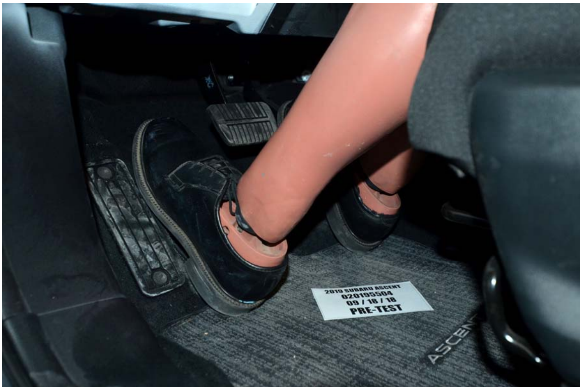
FIGURE 32. Pre-Test Placement of Dummy's Feet
