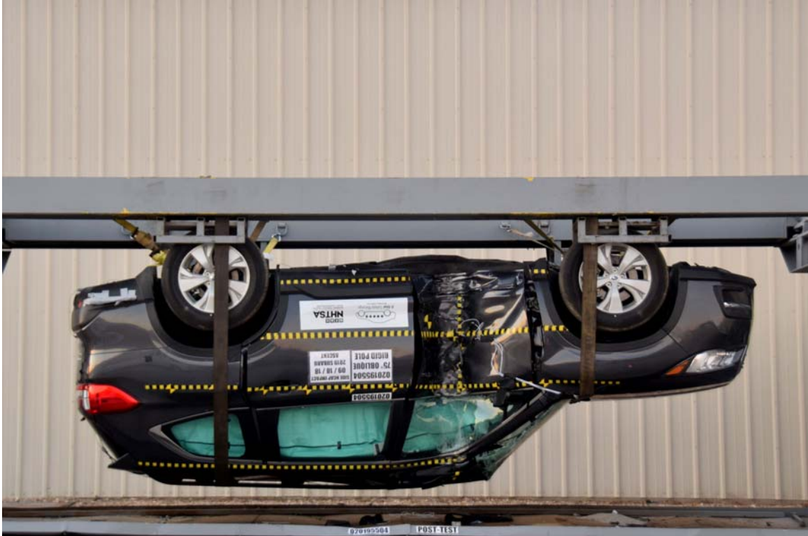
FIGURE 65. FMVSS No. 301 Static Rollover 180 Degrees
