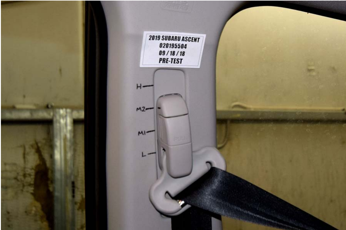
FIGURE 33. Pre-Test View of Belt Anchorage for Dummy
