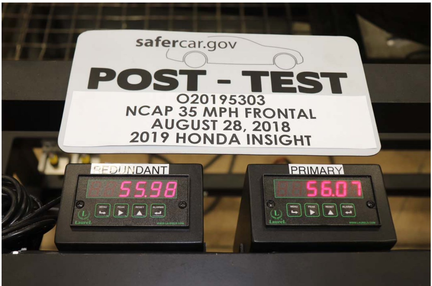
Photo No. 072 - Post-Test Speed Trap Read-Out
