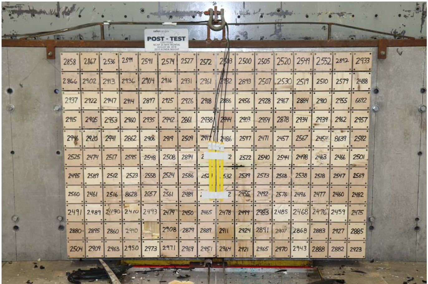
Photo No. 003 - Post-Test Load Cell Wall
