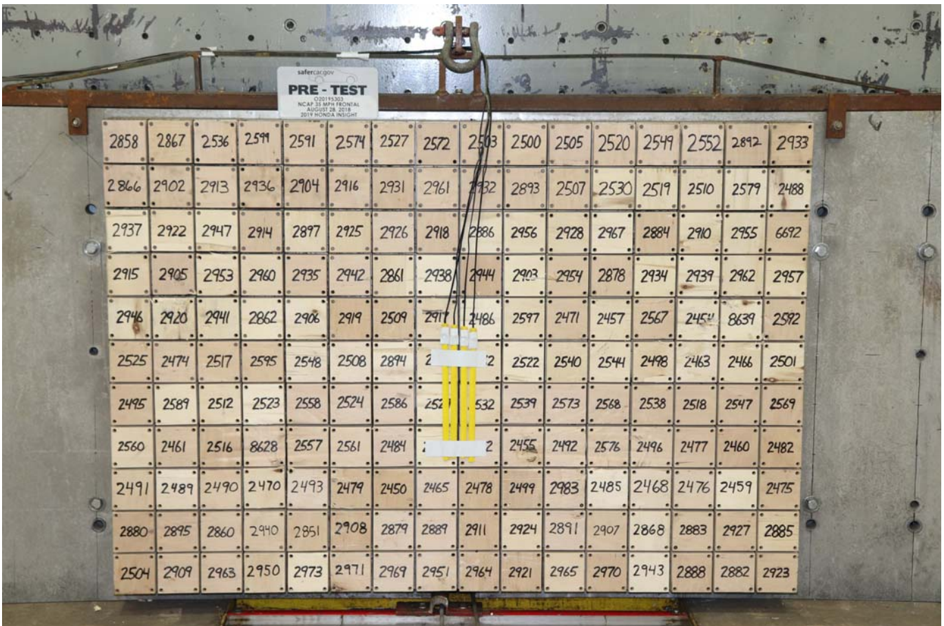
Photo No. 002 - Pre-Test Load Cell Wall
