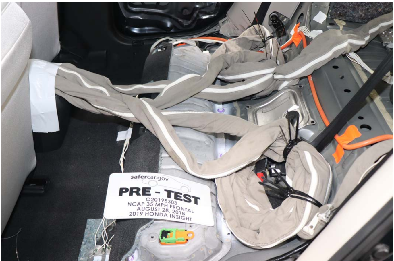
Photo No. 028 - Pre-Test Dummy Cable Routing
