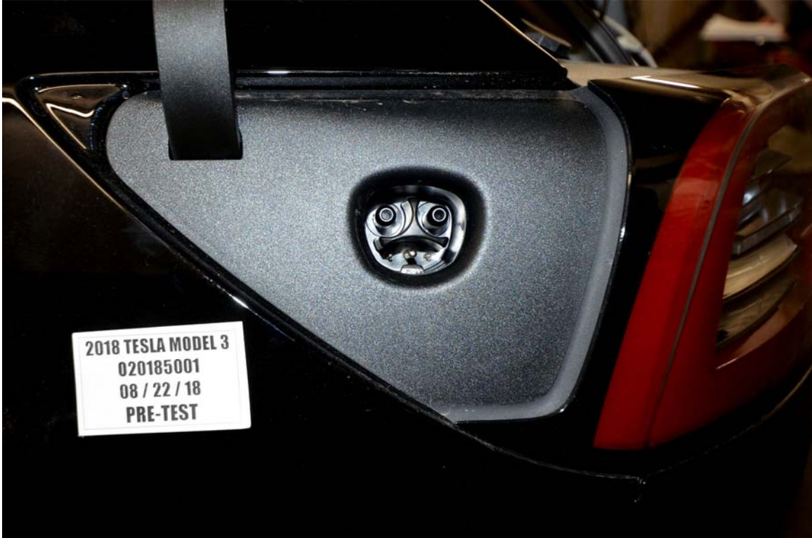
FIGURE 53. Pre-Test Fuel Filler Cap – Charge Port View
