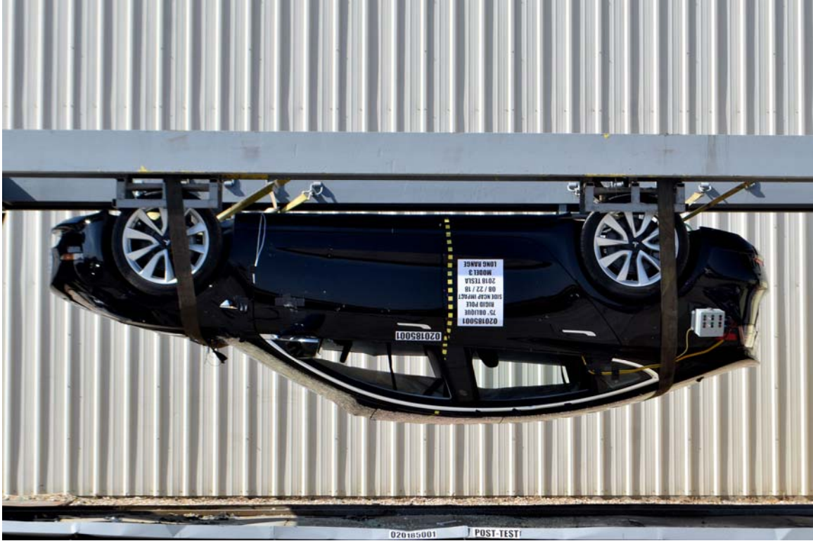
FIGURE 65. FMVSS No. 305 Static Rollover 180 Degrees
