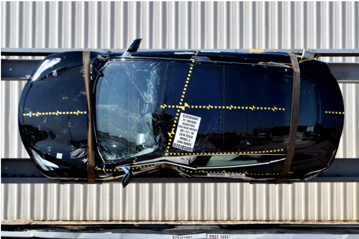
FIGURE 64. FMVSS No. 305 Static Rollover 90 Degrees
