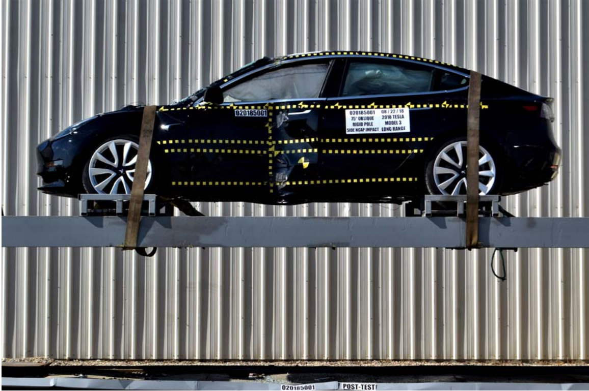
FIGURE 67. FMVSS No. 305 Static Rollover 360 Degrees
