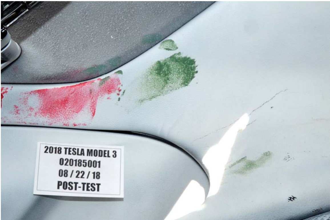
FIGURE 52. Post-Test Dummy Close-Up Knee Contact with Vehicle Interior View
