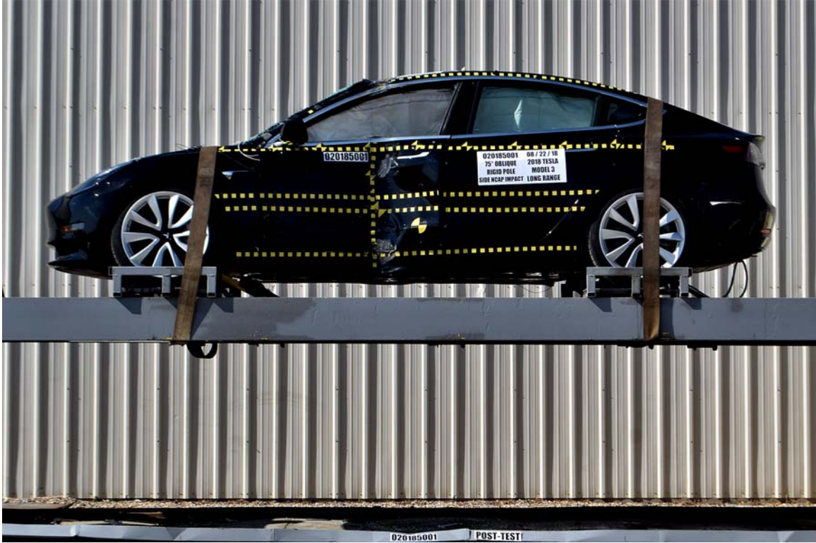
FIGURE 63. FMVSS No. 305 Static Rollover 0 Degrees
