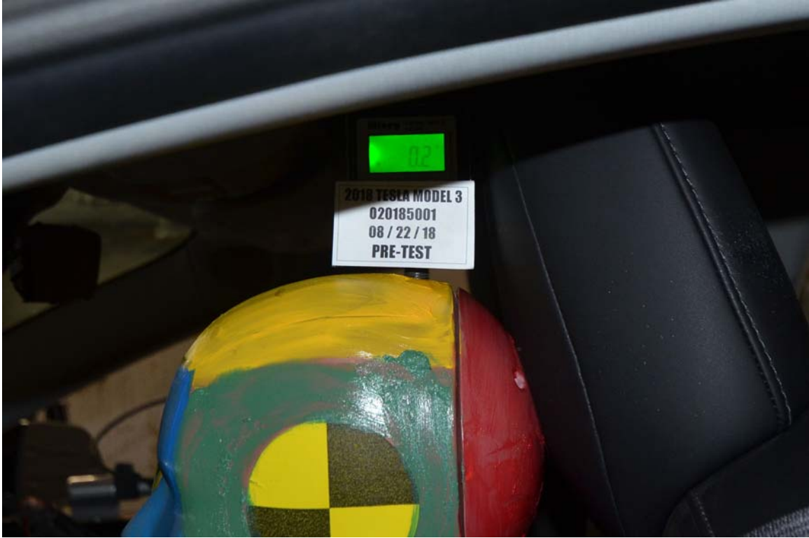
FIGURE 31. Pre-Test Left Side View of Dummy's Head Showing Dummy's Head is Level
