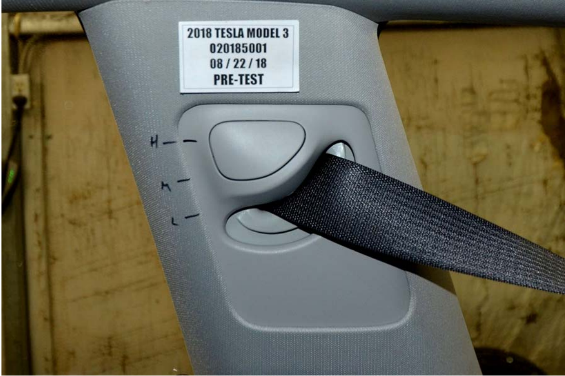
FIGURE 33. Pre-Test View of Belt Anchorage for Dummy
