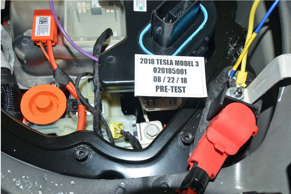
FIGURE 24. Pre-Impact Close-Up View of High Voltage Leads Attached
