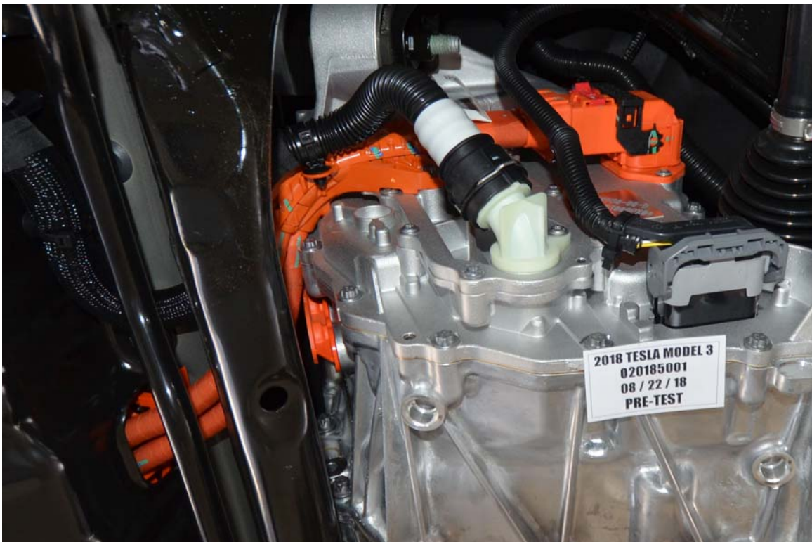
FIGURE 19a. Pre-Impact View of High Voltage Interconnect(s)
