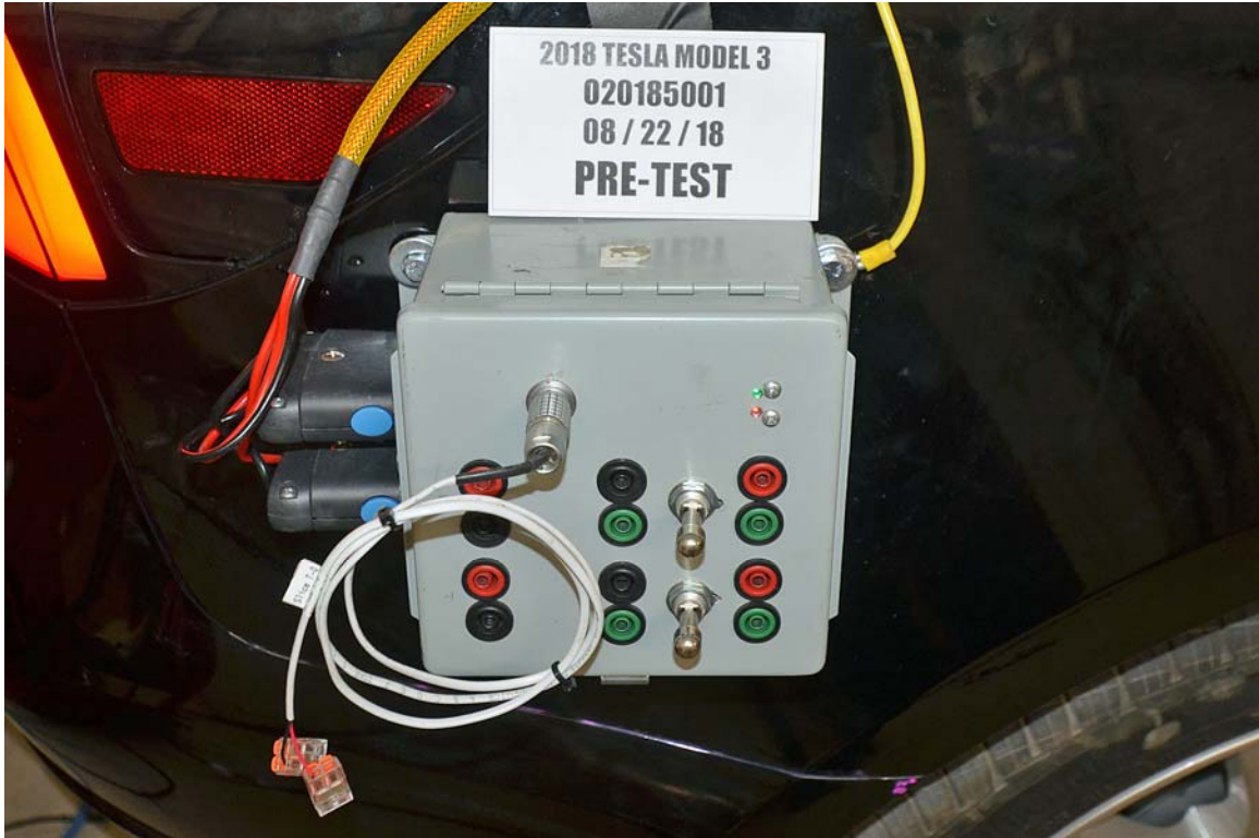
FIGURE 25. Pre-Impact View of Installed Test Interface Port
