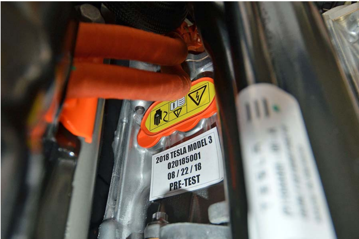
FIGURE 2b. Power Inverter Warning Label
