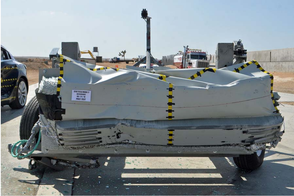
FIGURE 85. Post-Test Front View of MDB Impactor Face
