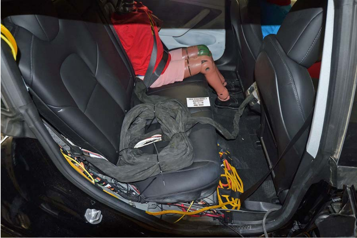
FIGURE 34. Pre-Impact View of the Vehicle Passenger Compartment Adjacent to Propulsion Battery
