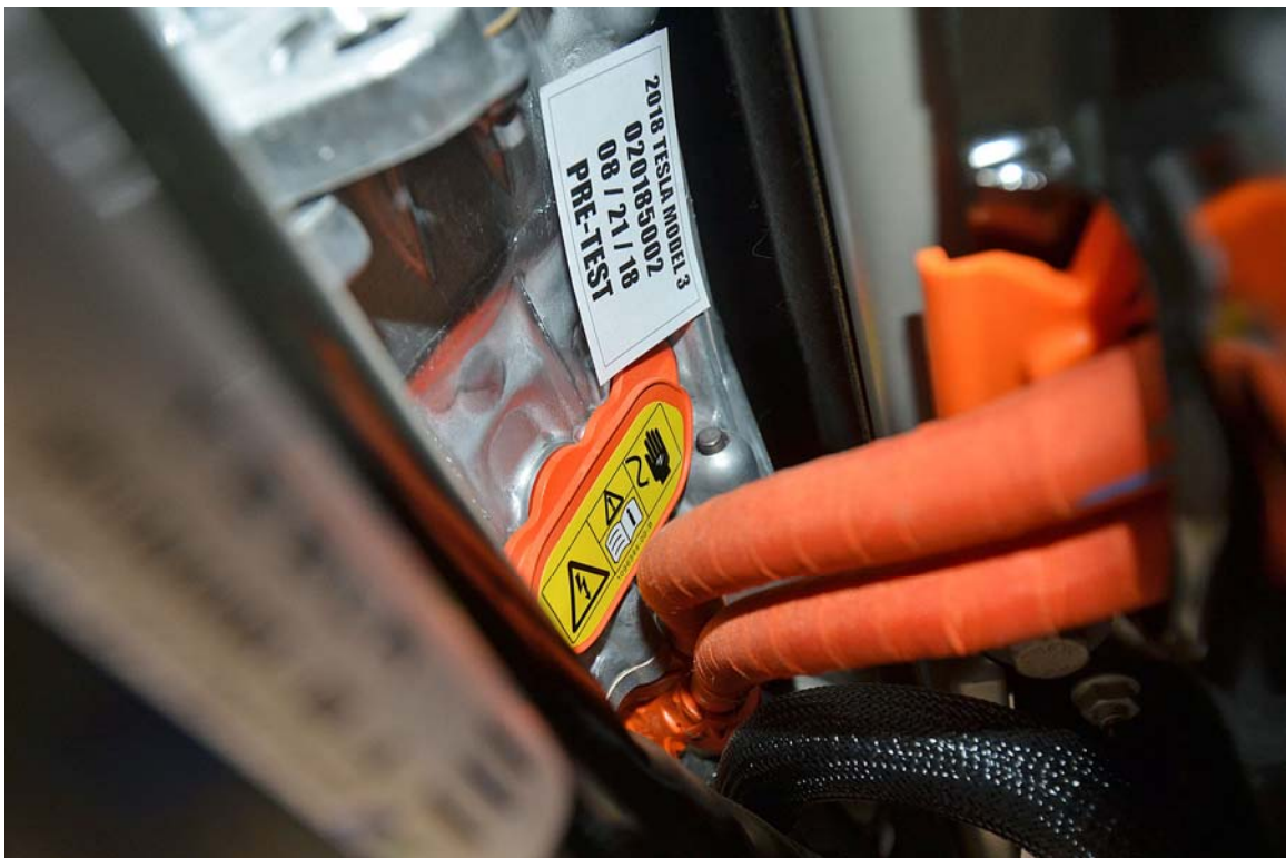
FIGURE 2b. Power Inverter Warning Label
