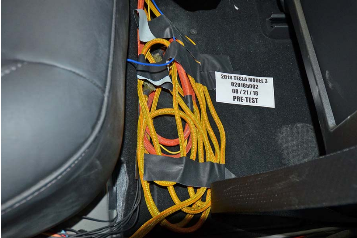
FIGURE 23. Pre-Impact View of High Voltage Leads Attached
