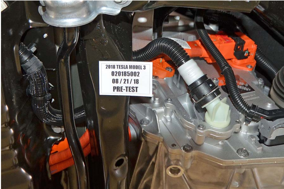
FIGURE 19b. Pre-Impact View of High Voltage Interconnect(s)
