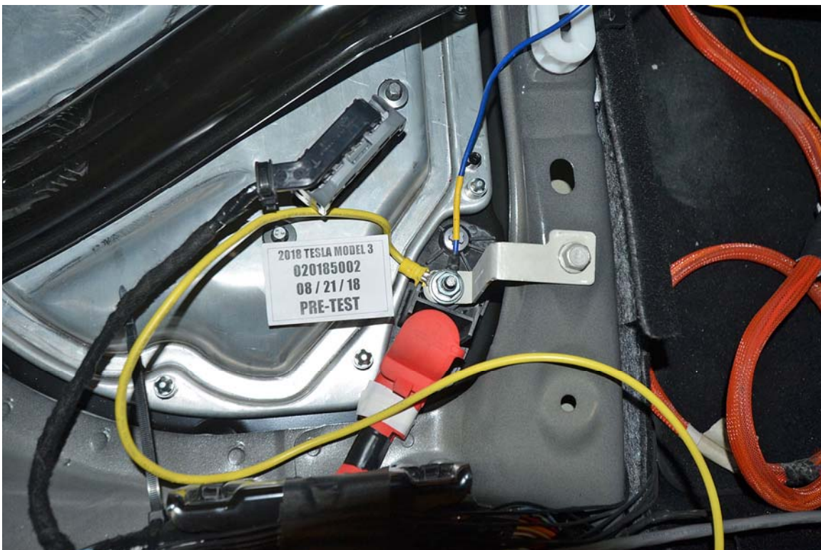
FIGURE 22. Pre-Impact View of Ground Lead Attached
