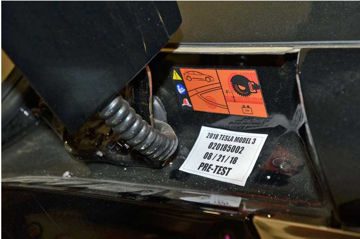
FIGURE 3. First Responder Warning Label
