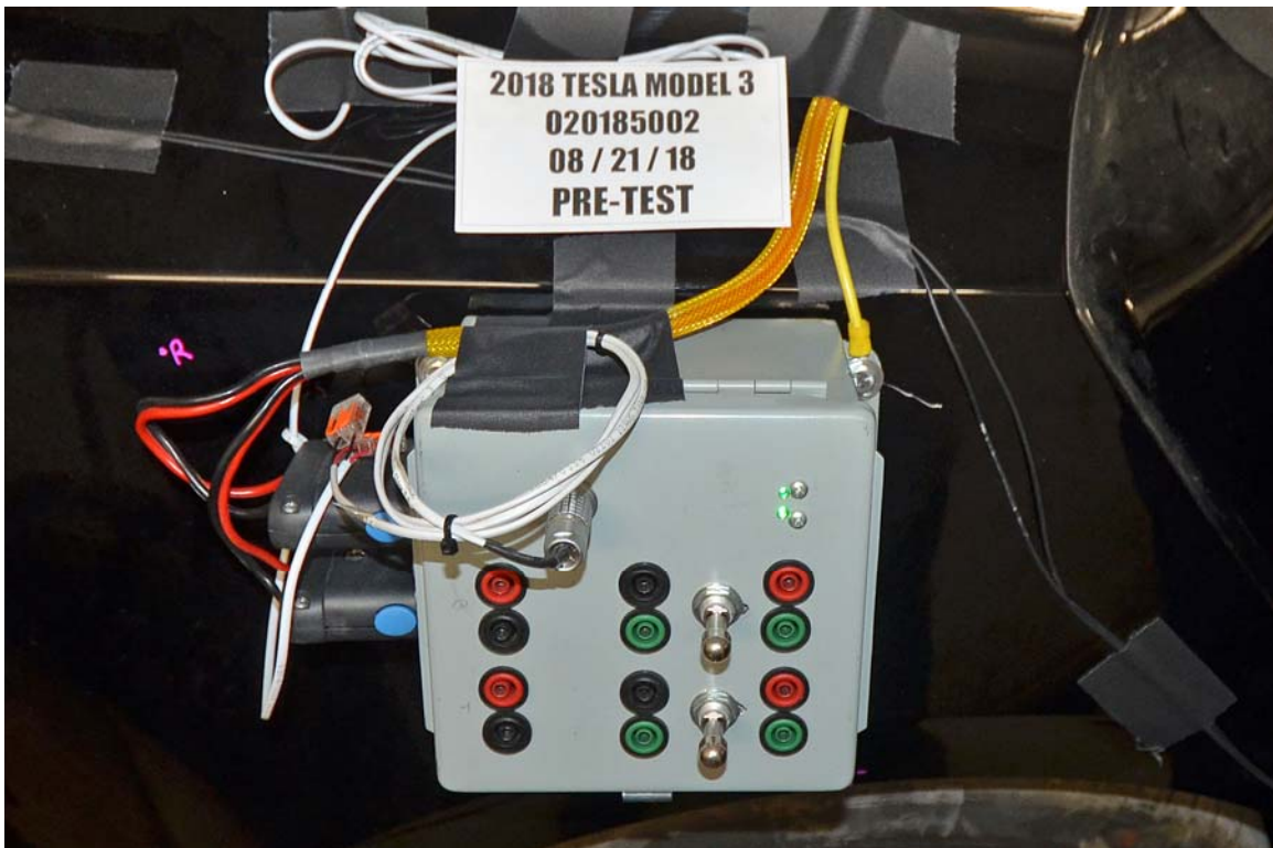
FIGURE 25. Pre-Impact View of Installed Test Interface Port
