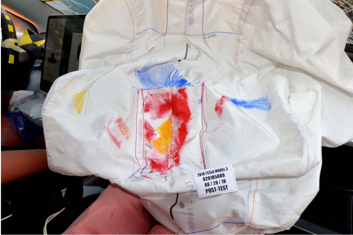
FIGURE 68. Post-Test Passenger Dummy Contact with Airbag
