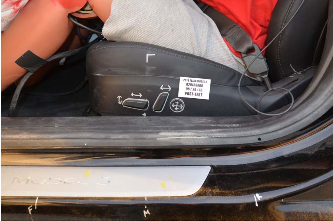
FIGURE 37. Post-Test Driver's Seat Fore-Aft Markings
