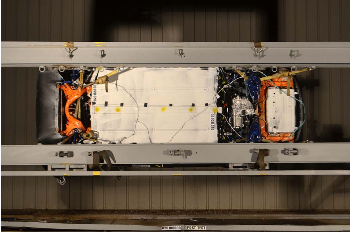
FIGURE 76. Vehicle at 270° on Static Rollover Device
