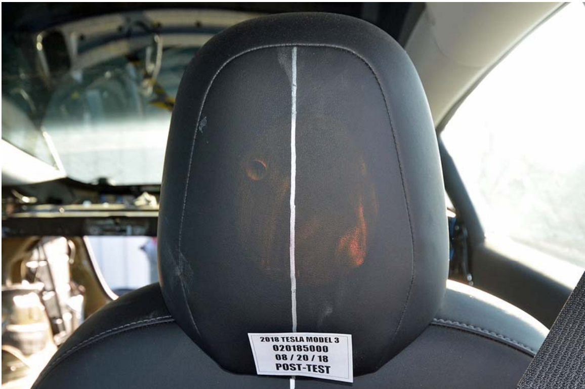
FIGURE 48. Post-Test Driver Dummy Contact with Headrest
