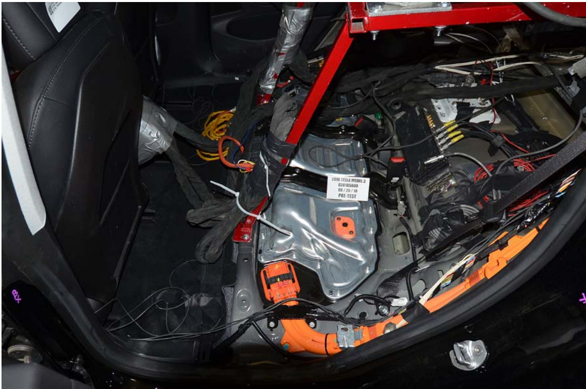
FIGURE 28. Pre-Test Dummy Cable Routing
