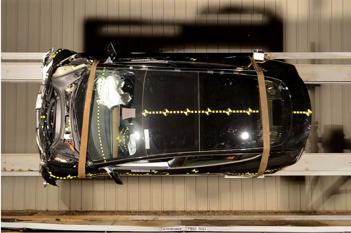
FIGURE 74. Vehicle at 90° on Static Rollover Device
