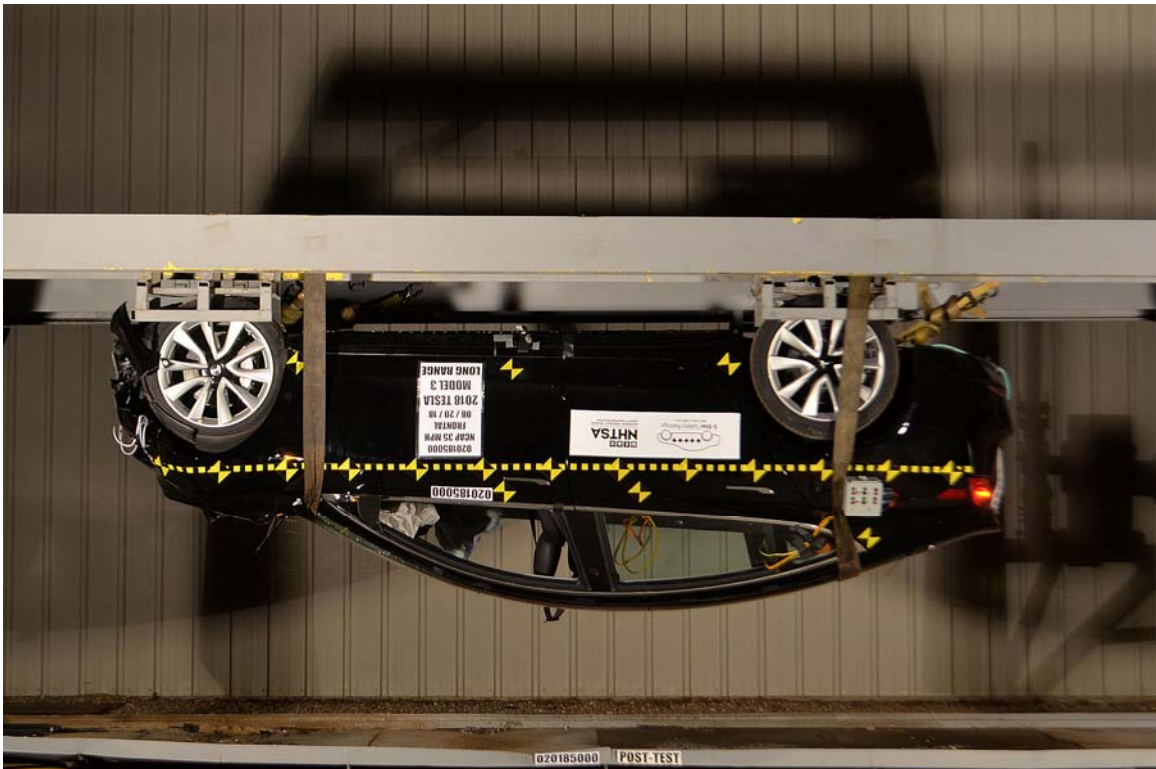
FIGURE 75. Vehicle at 180° on Static Rollover Device
