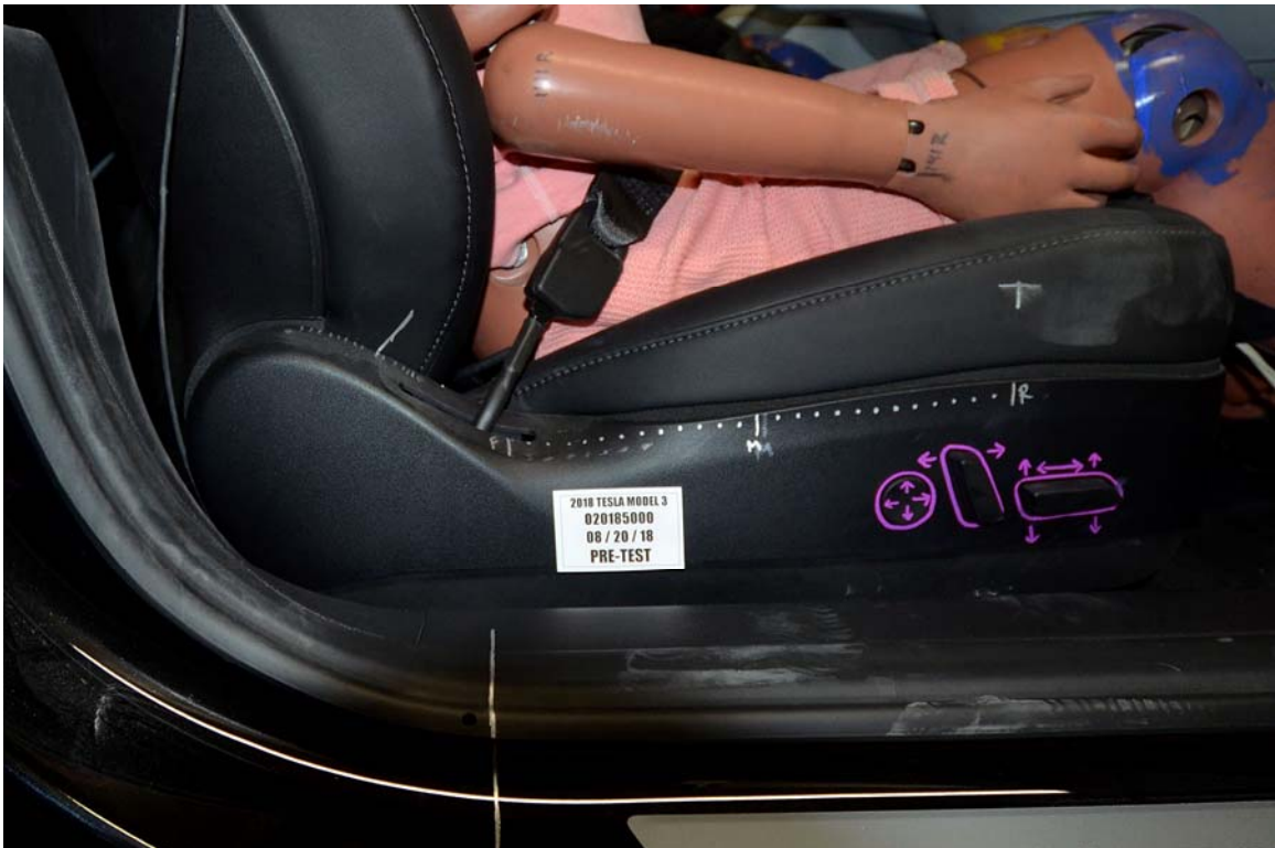
FIGURE 57. Pre-Test Passenger's Seat Fore-Aft Markings
