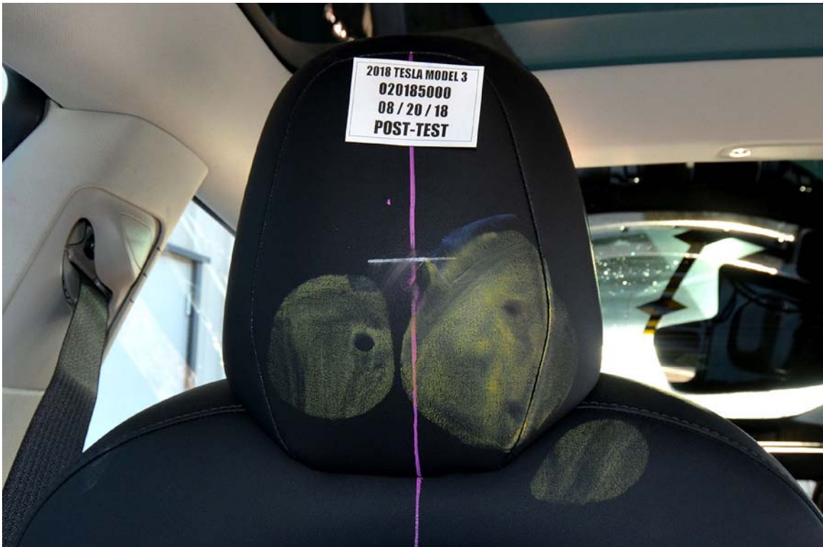
FIGURE 69. Post-Test Passenger Dummy Contact with Headrest
