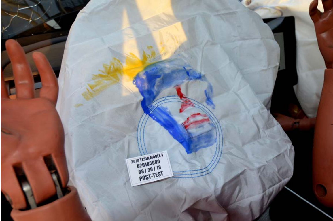
FIGURE 47. Post-Test Driver Dummy Contact with Airbag
