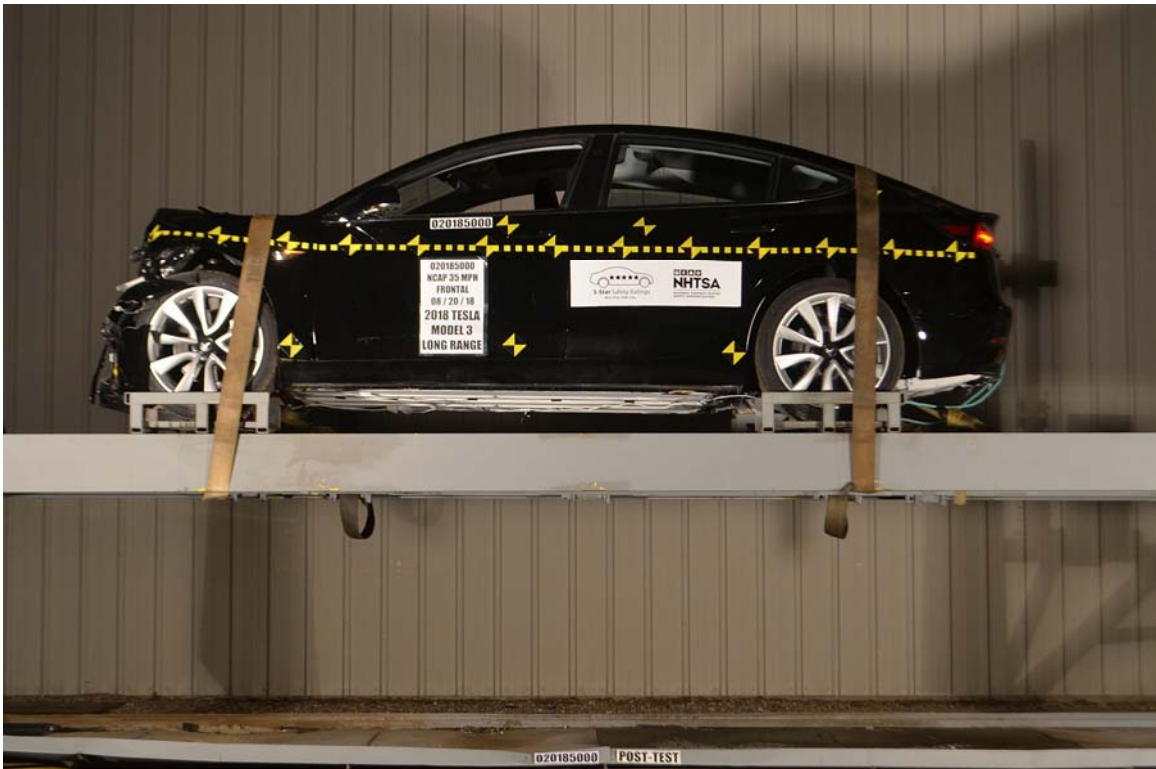
FIGURE 73. Vehicle at 0° on Static Rollover Device
