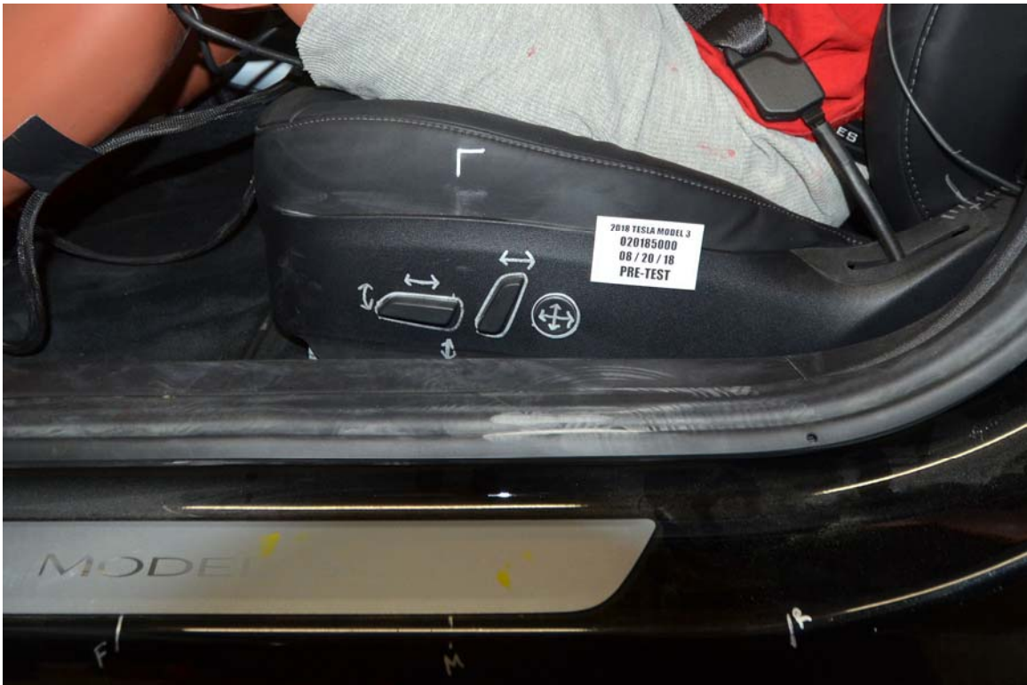
FIGURE 36. Pre-Test Driver's Seat Fore-Aft Markings
