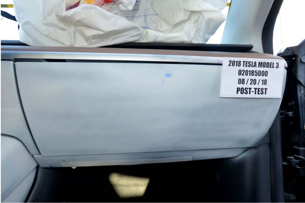
FIGURE 64. Post-Test Passenger's Side Knee Bolster
