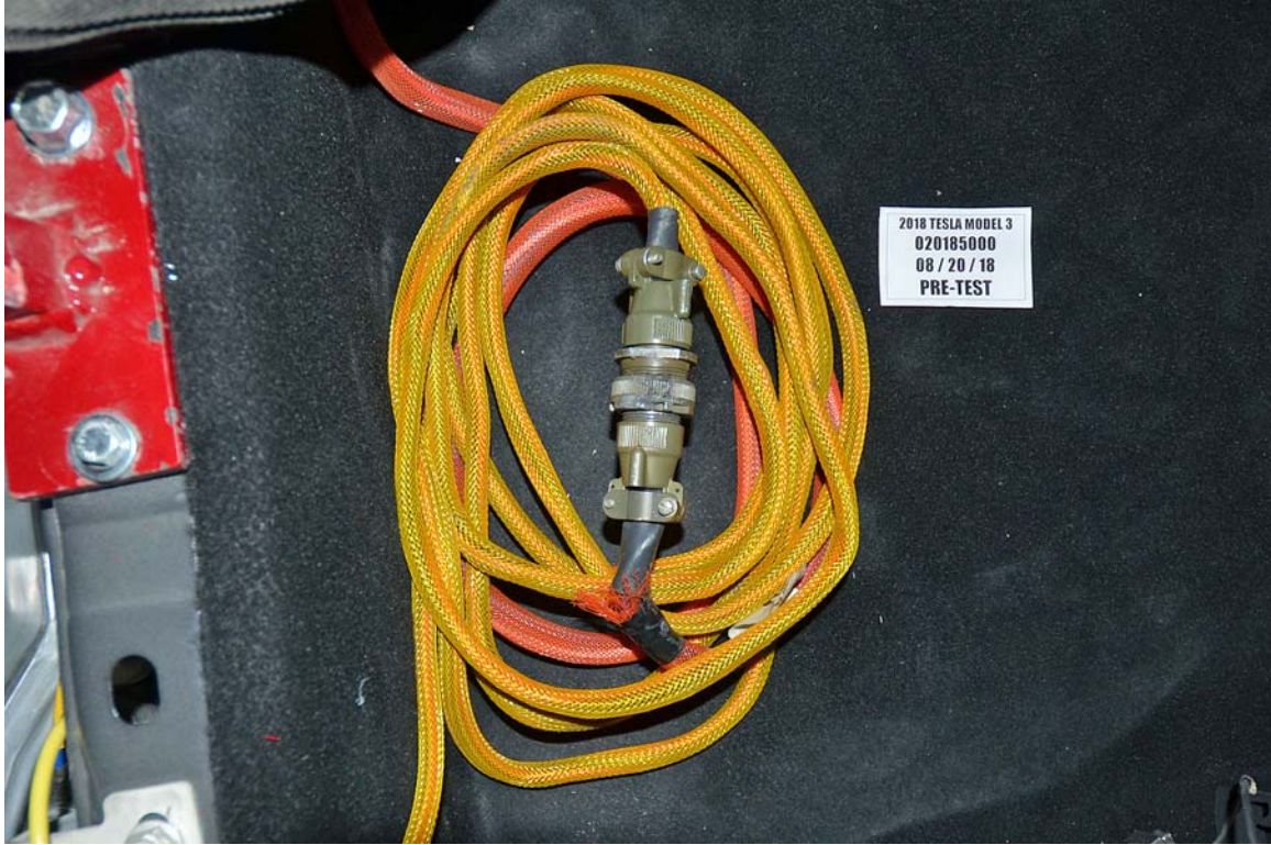
FIGURE 23. Pre-Impact View of High Voltage Leads Attached
