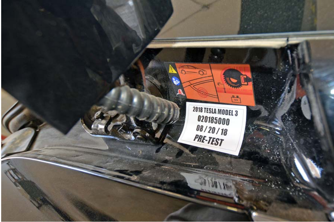
FIGURE 3. First Responder Warning Label
