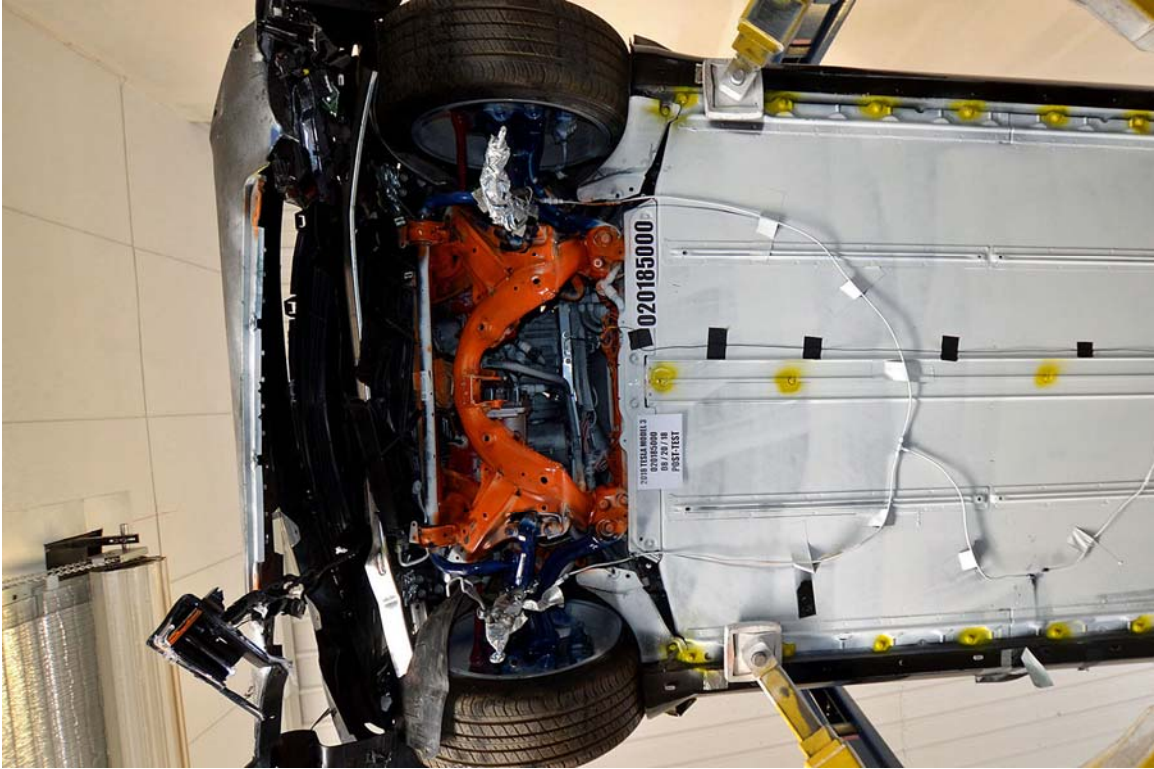
FIGURE 10. Post-Impact Front View of Propulsion Battery
