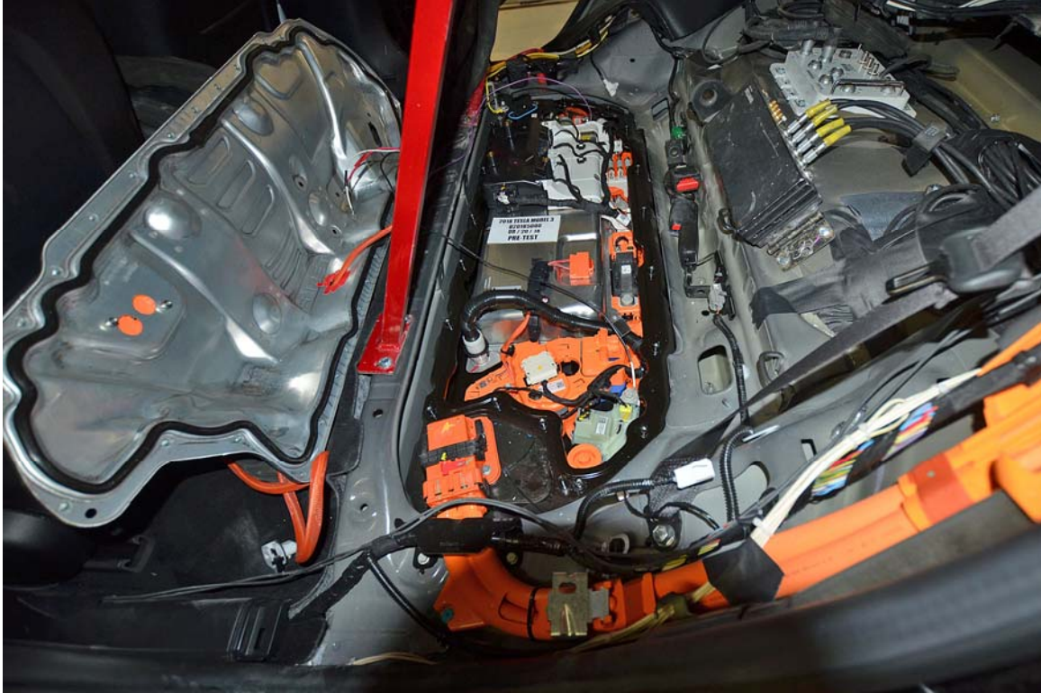
FIGURE 21. Pre-Impact View of Other Visible Electric Propulsion Components
