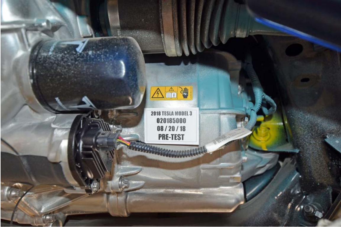
FIGURE 2a. Power Inverter Warning Label
