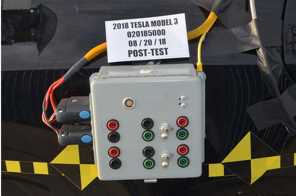
FIGURE 26. Post-Impact View of Installed Test Interface Port
