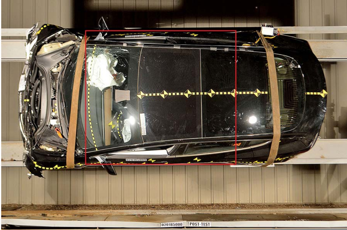
FIGURE 30. FMVSS No. 305 Static Rollover at 90°
