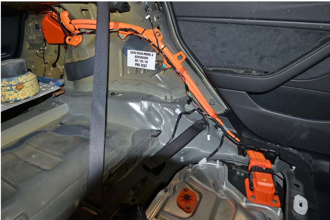
FIGURE 19. Pre-Impact View of High Voltage Interconnect(s)
