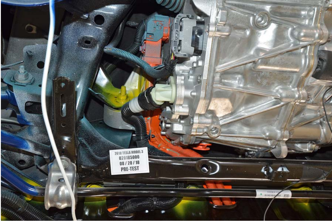
FIGURE 19c. Pre-Impact View of High Voltage Interconnect(s)
