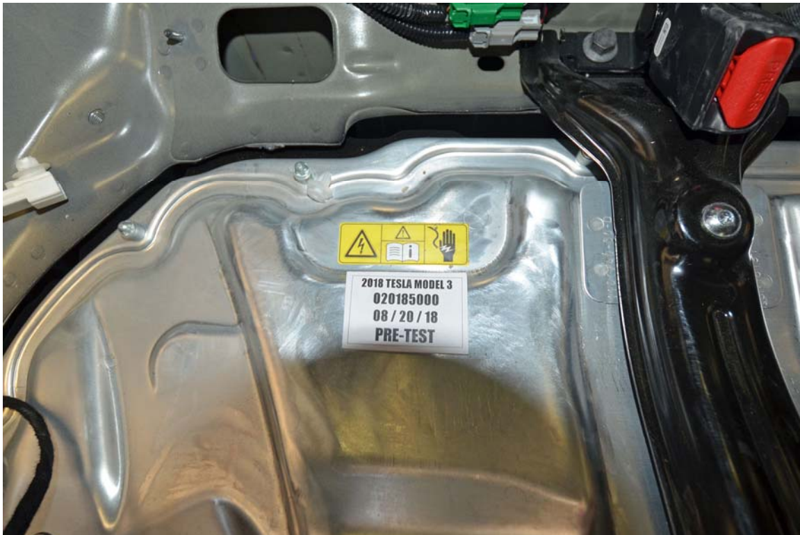
FIGURE 2. Power Inverter Warning Label
