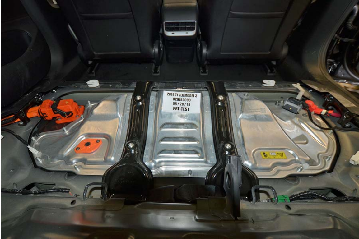
FIGURE 8. Pre-Impact View of Propulsion Battery
