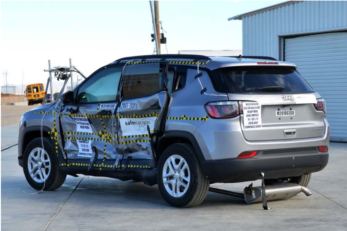
FIGURE 5. Post-Test Left Rear ¾ View of NCAP Side MDB Impact Test
