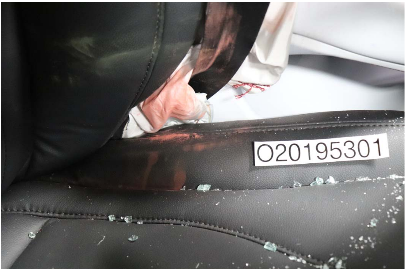
Photo No. 050 - Post-Test Dummy Close-Up Pelvis Contact with Vehicle Interior View
