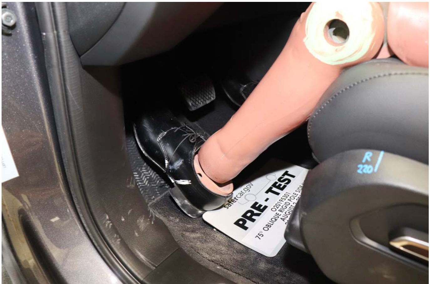
Photo No. 032 - Pre-Test Placement of Dummy Feet
