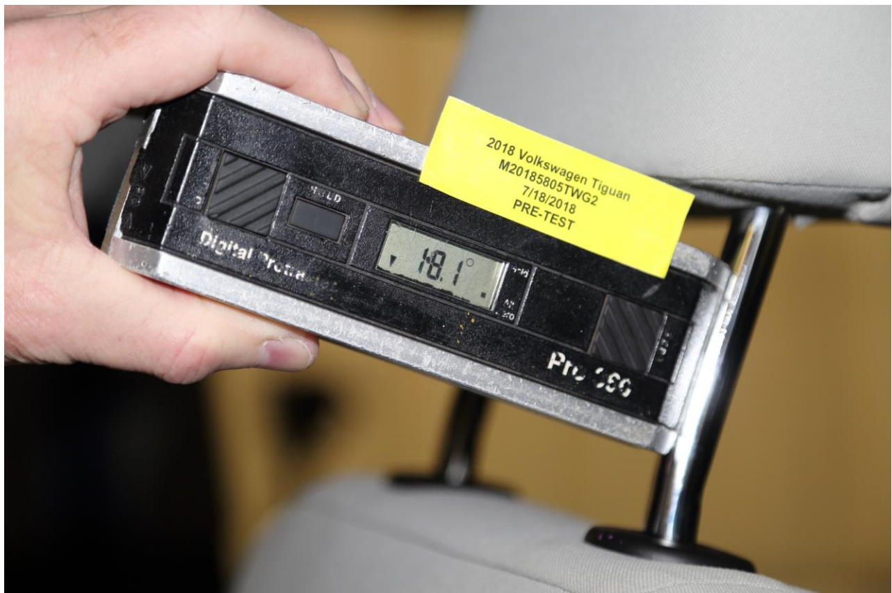
Figure A-8 Pre-Test Vehicle Seat Back Angle
