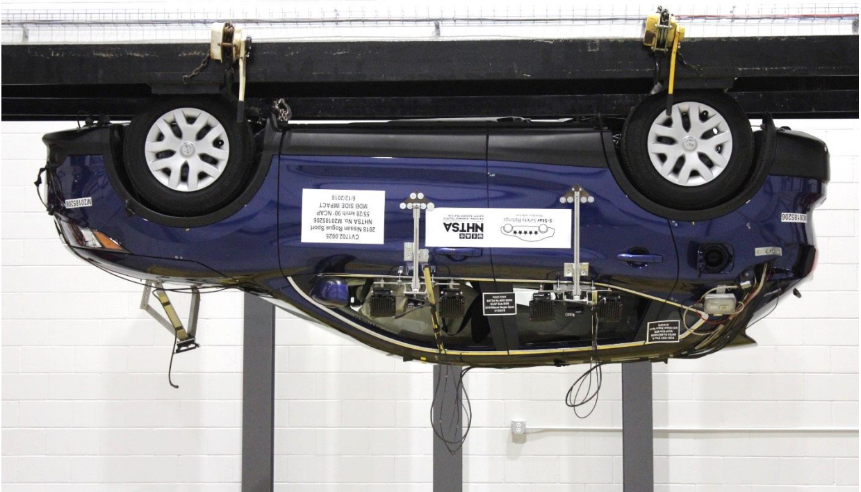
Figure A-98: FMVSS No. 301 Static Rollover 180 Degrees
