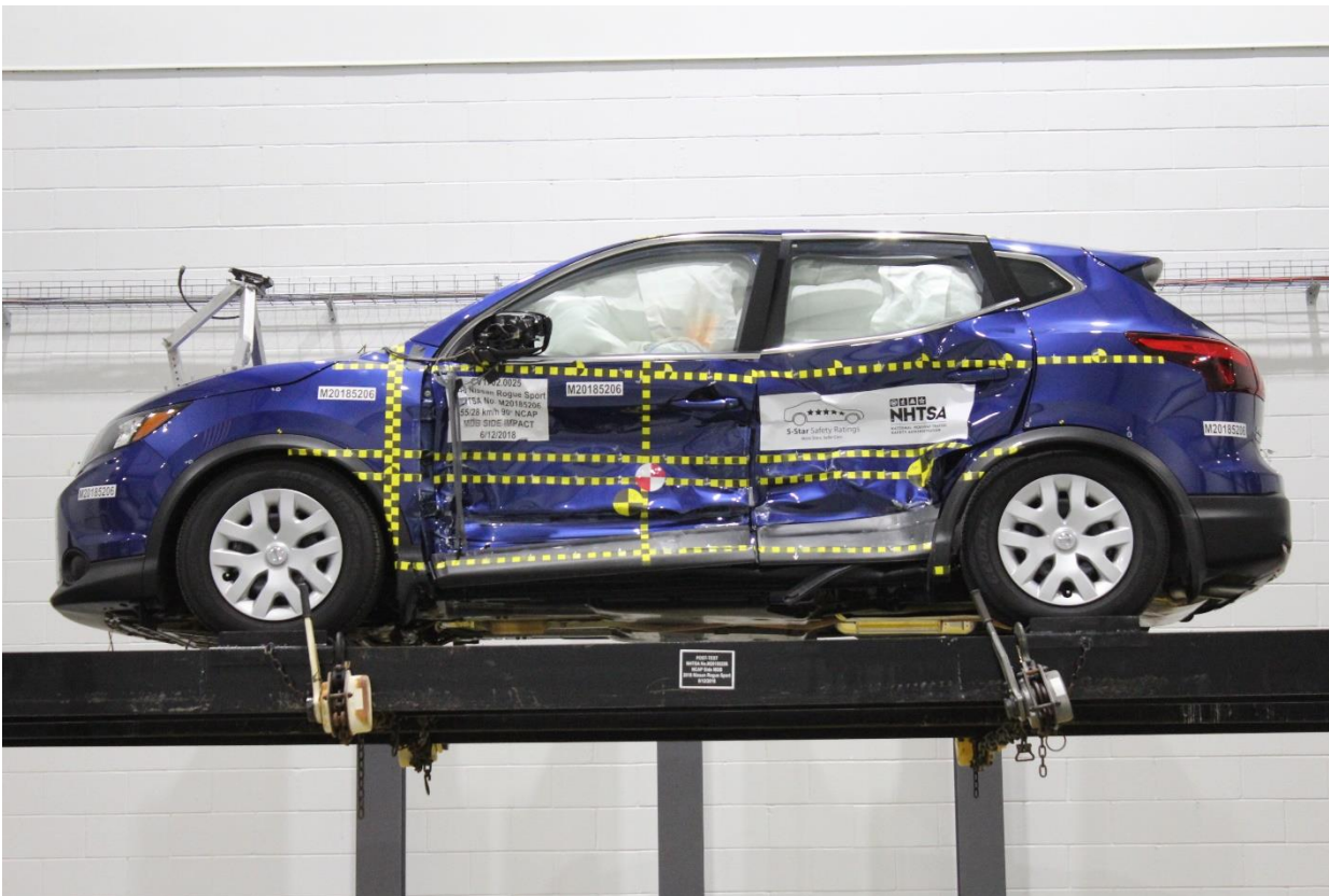
Figure A-96: FMVSS No. 301 Static Rollover 0 Degrees
