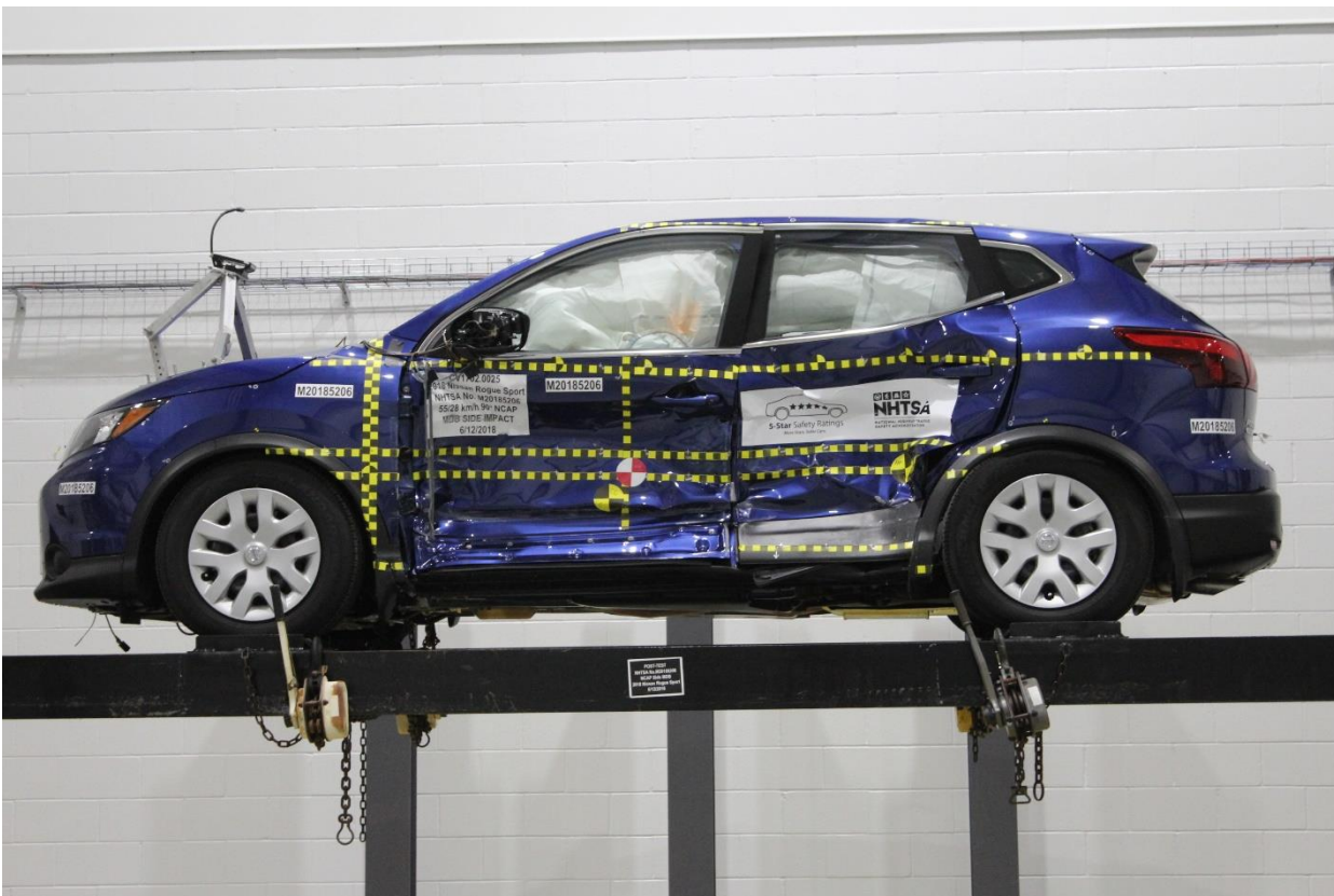
Figure A-100: FMVSS No. 301 Static Rollover 360 Degrees
