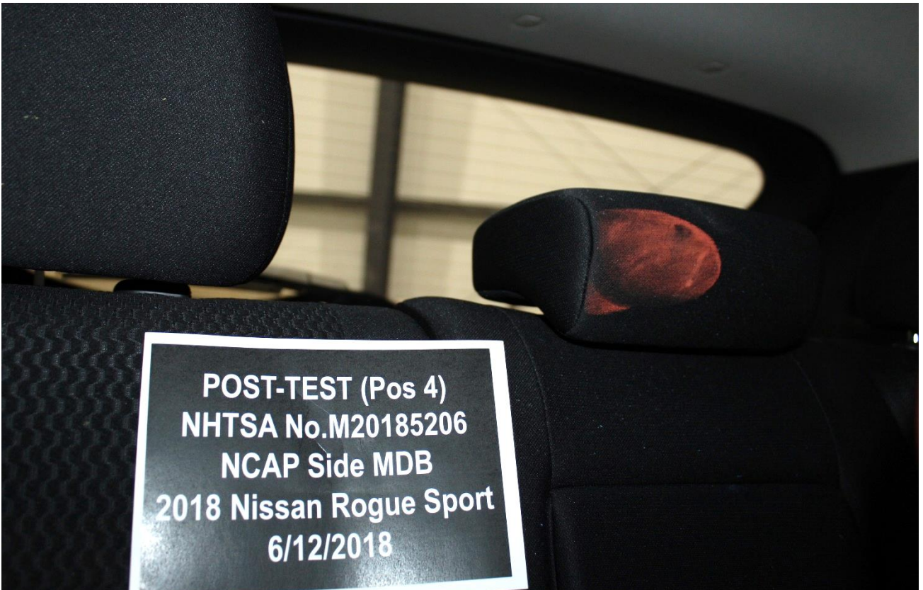
Figure A-75: Post-Test Rear Passenger Dummy Close-Up Head Contact with Vehicle View
