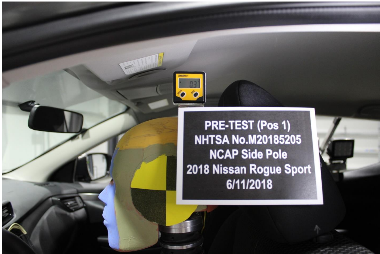
Figure A-31: Pre-Test Left Side View of Dummy's Head Showing Dummy's Head is Level
