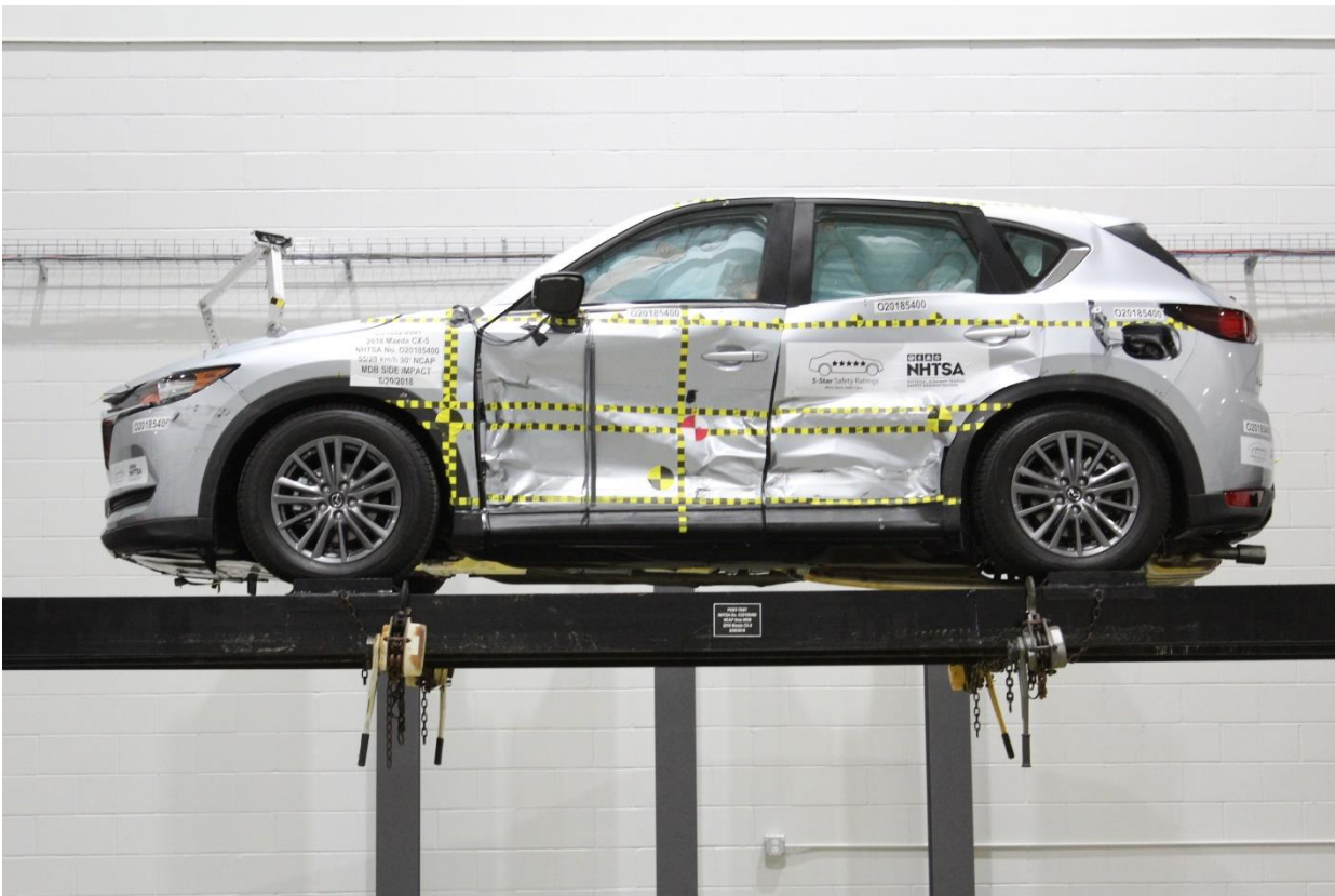
Figure A-96: FMVSS No. 301 Static Rollover 0 Degrees
