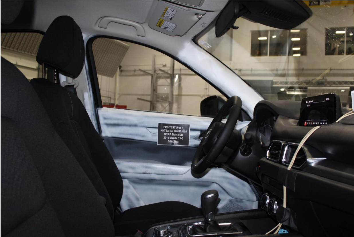
Figure A-46: Pre-Test Driver Inner Door Panel View
