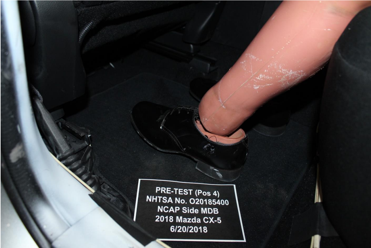
Figure A-64: Pre-Test Placement of Rear Passenger Dummy's Feet
