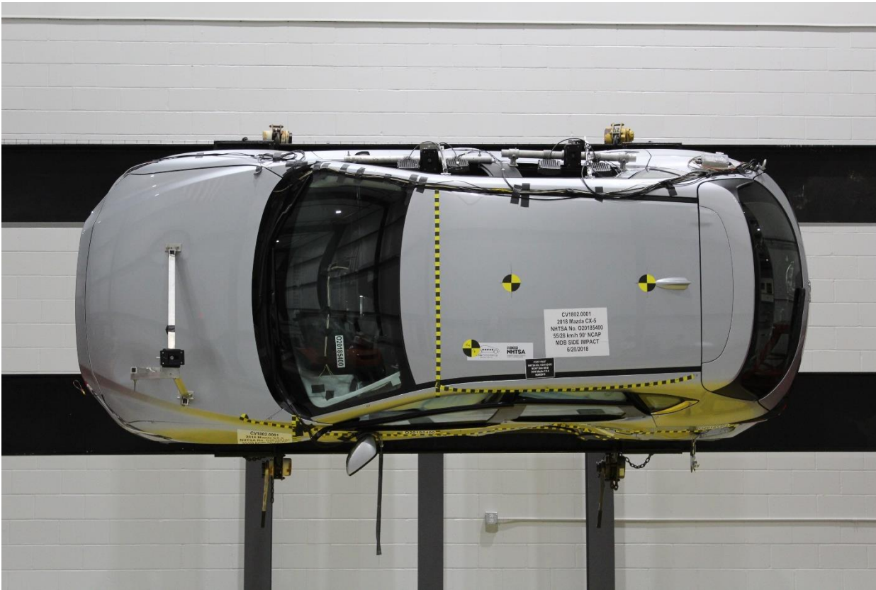
Figure A-97: FMVSS No. 301 Static Rollover 90 Degrees
