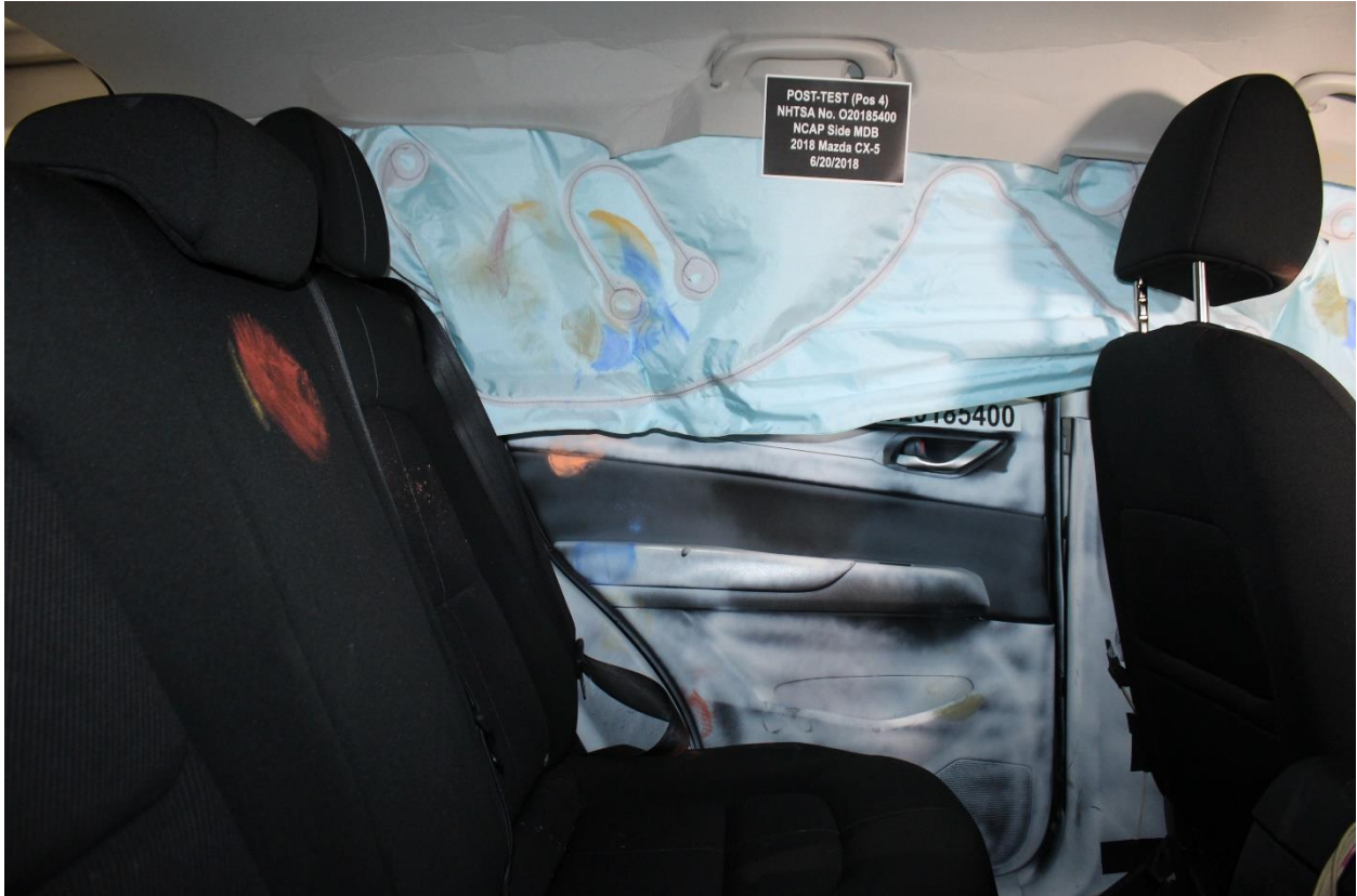
Figure A-74: Post-Test Rear Passenger Inner Door Panel View Showing Rear Passenger Contact Locations
