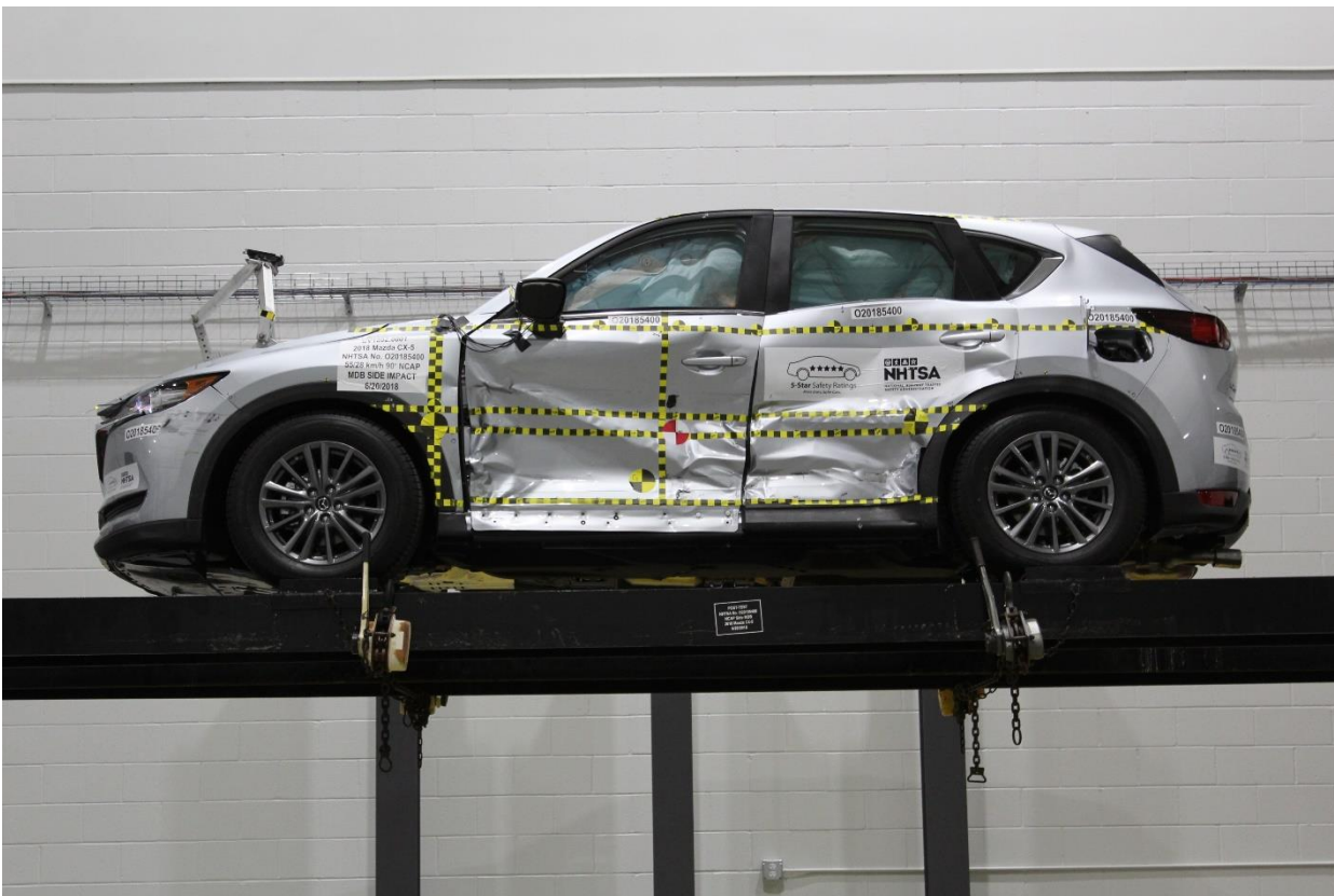
Figure A-100: FMVSS No. 301 Static Rollover 360 Degrees
