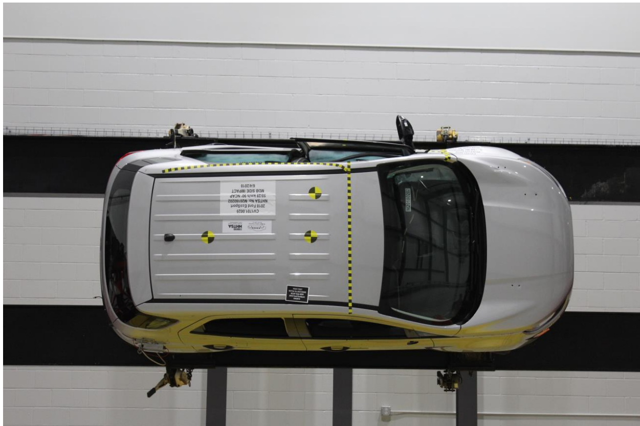
Figure A-99: FMVSS No. 301 Static Rollover 270 Degrees
