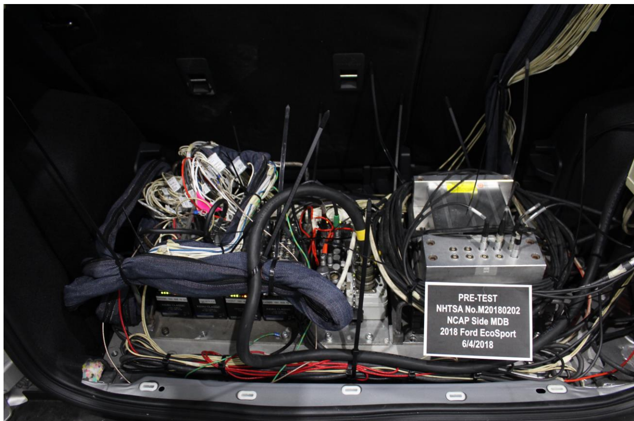
Figure A-94: Pre-Test Ballast View
