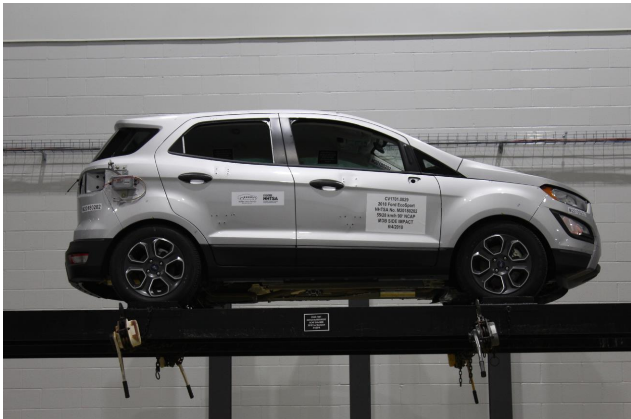
Figure A-96: FMVSS No. 301 Static Rollover 0 Degrees
