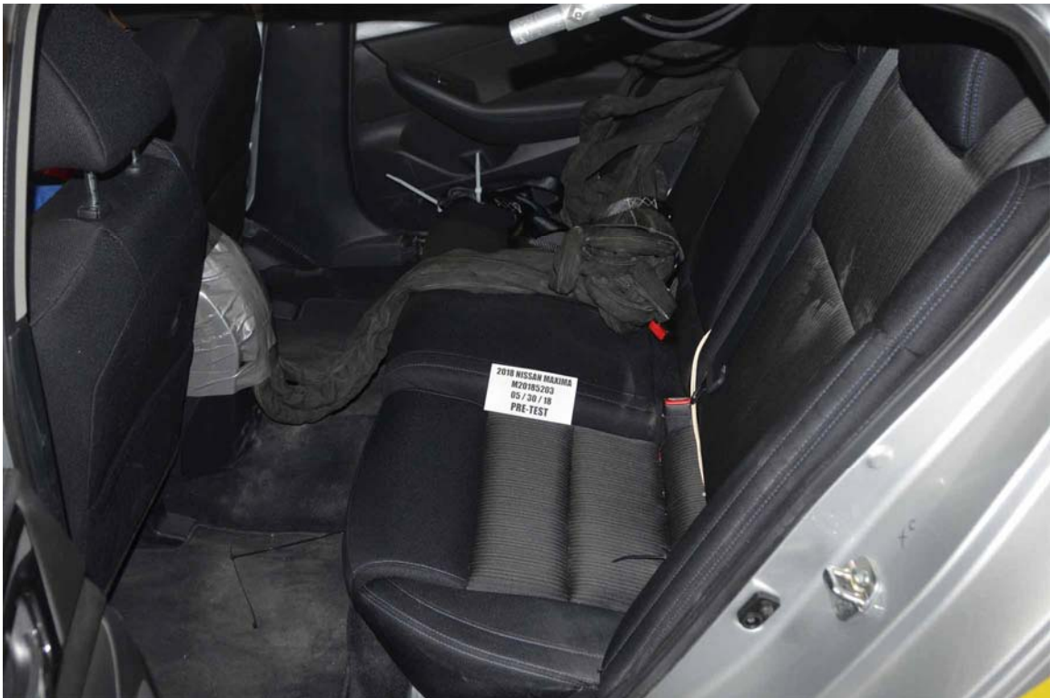
FIGURE 28. Pre-Test Dummy Cable Routing
