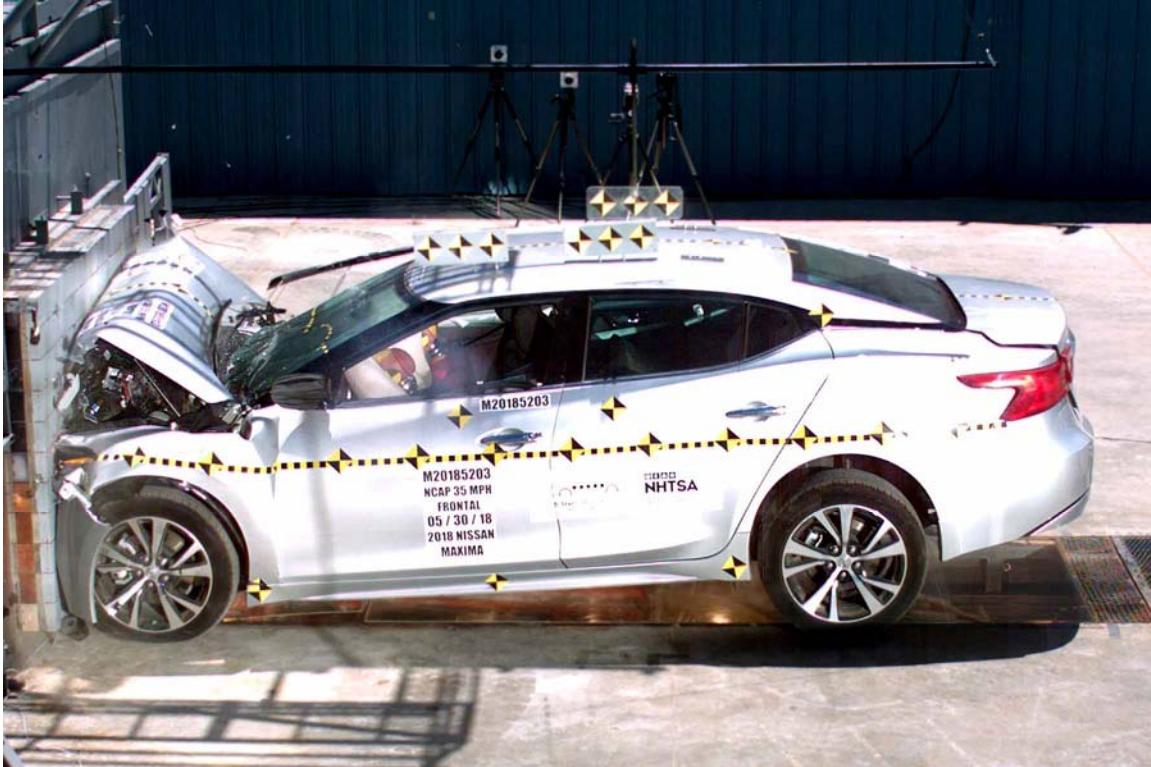
FIGURE 78. 2018 Nissan Maxima Frontal Impact Event
