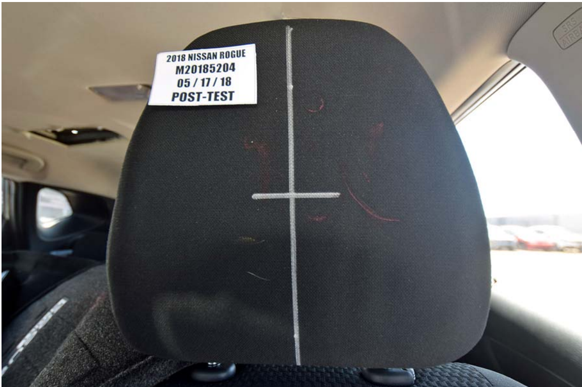
FIGURE 48. Post-Test Driver Dummy Contact with Headrest
