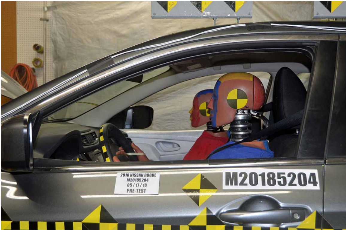
FIGURE 32. Pre-Test Driver Dummy Window View
