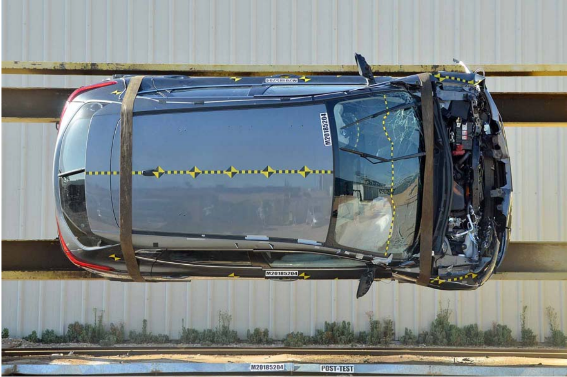
FIGURE 74. Vehicle at 90° on Static Rollover Device
