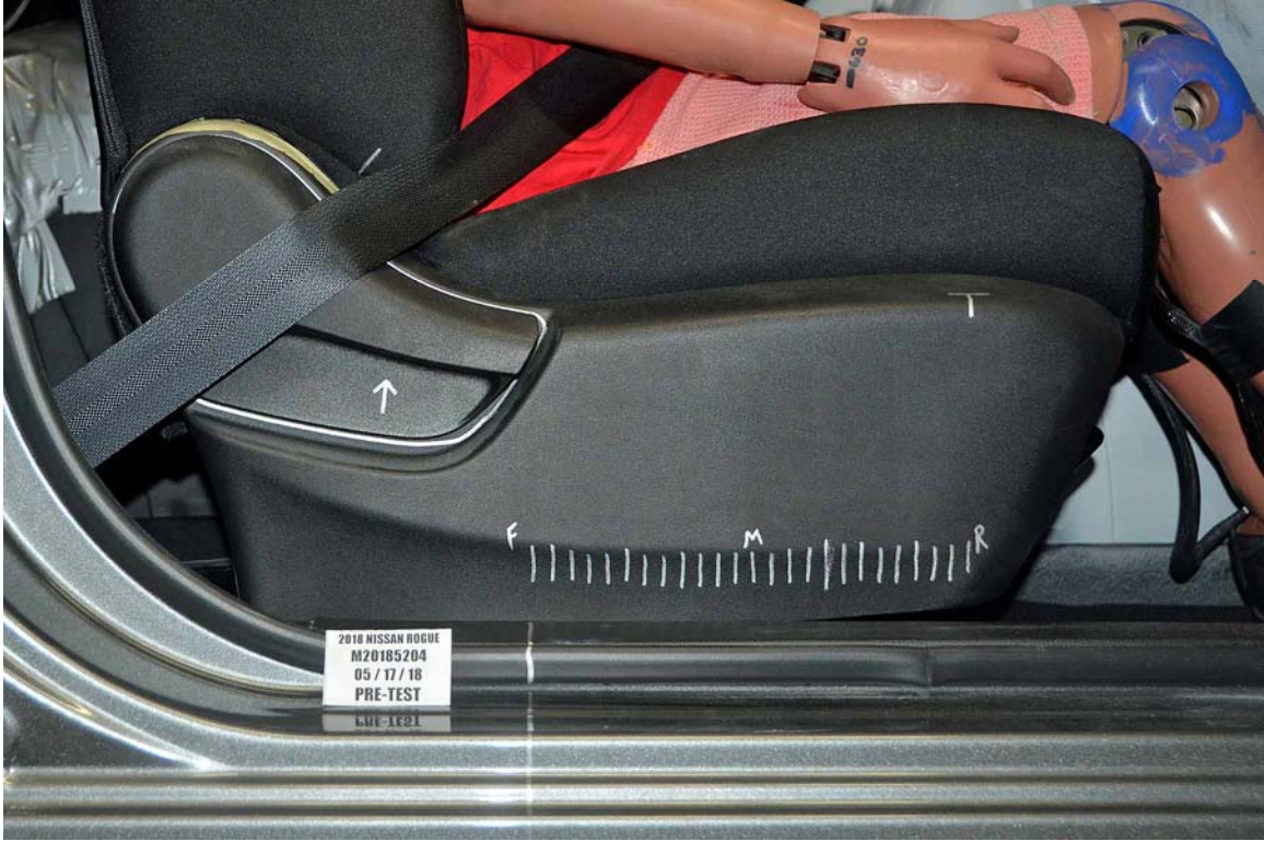
FIGURE 57. Pre-Test Passenger's Seat Fore-Aft Markings
