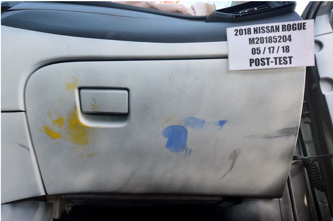
FIGURE 64. Post-Test Passenger's Side Knee Bolster
