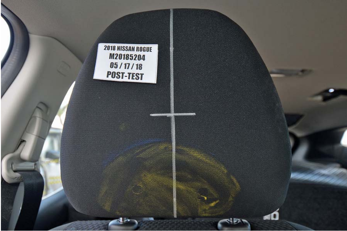
FIGURE 69. Post-Test Passenger Dummy Contact with Headrest
