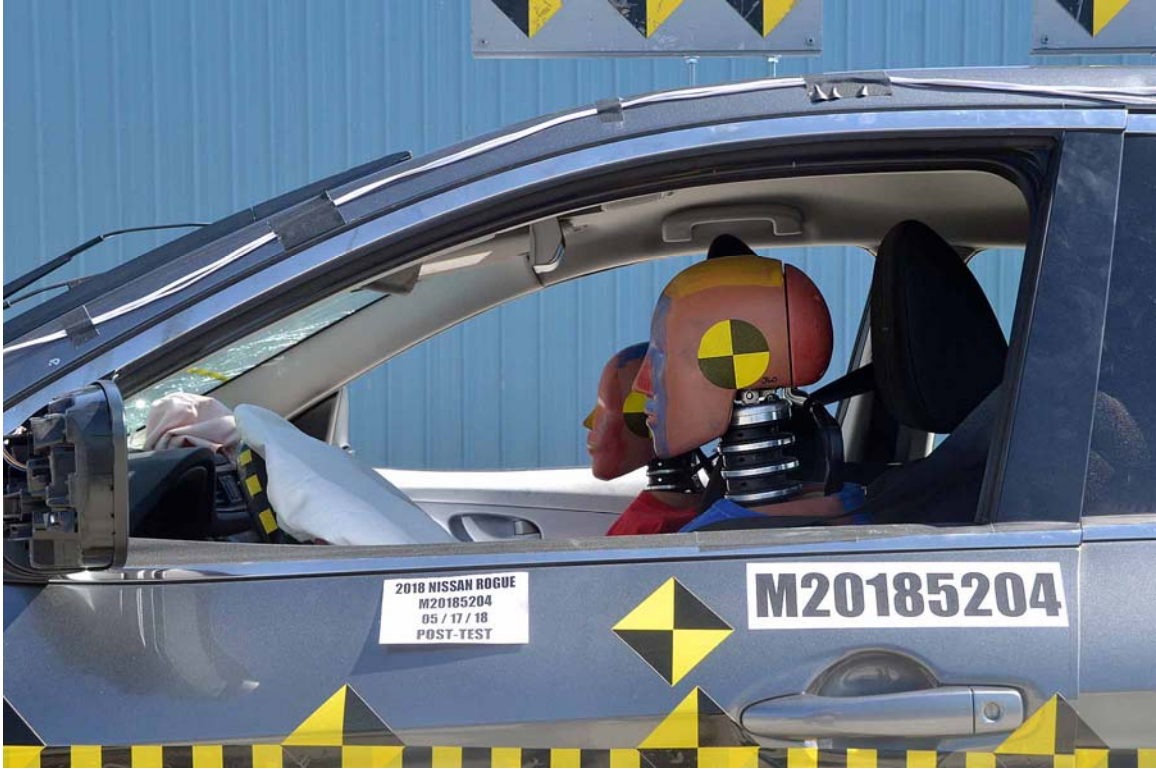
FIGURE 33. Post-Test Driver Dummy Window View
