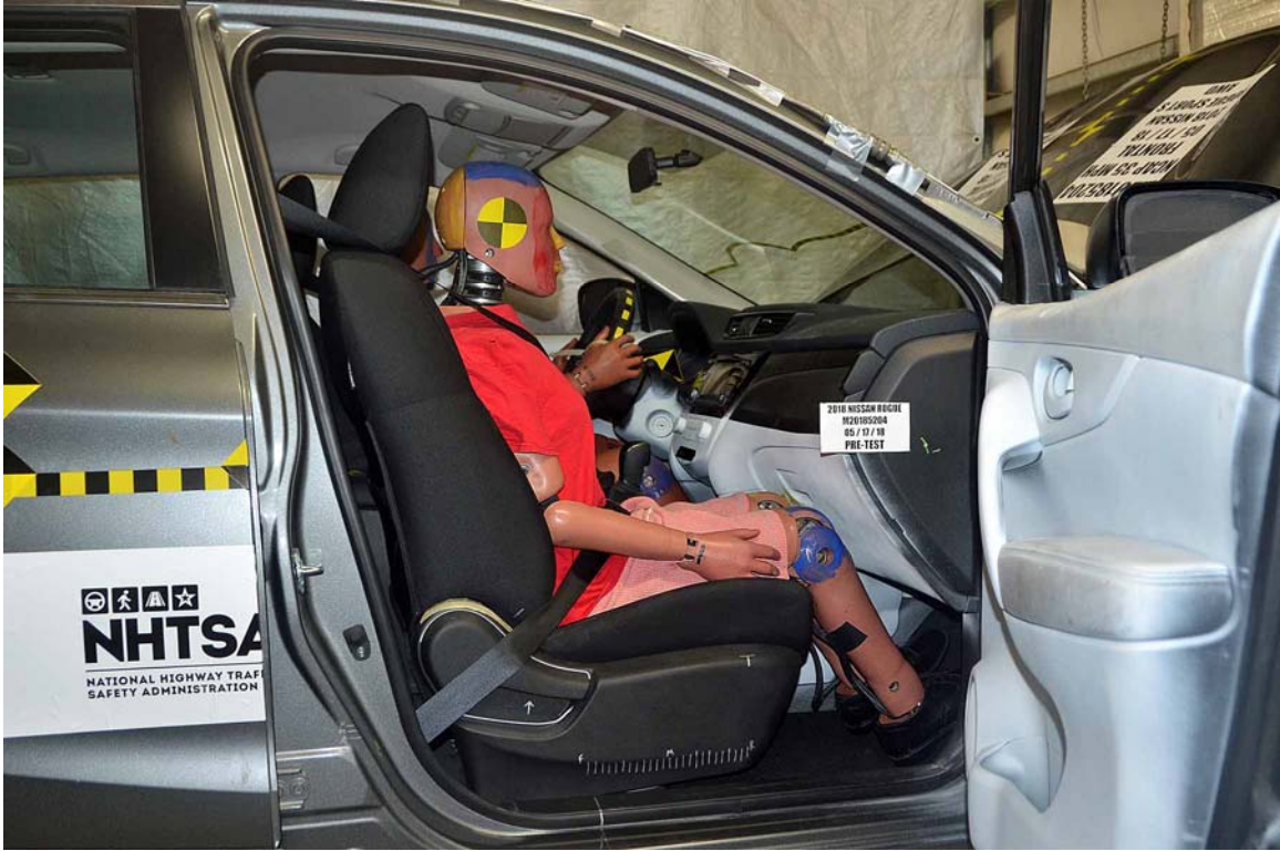
FIGURE 55. Pre-Test Passenger Dummy and Vehicle Interior View
