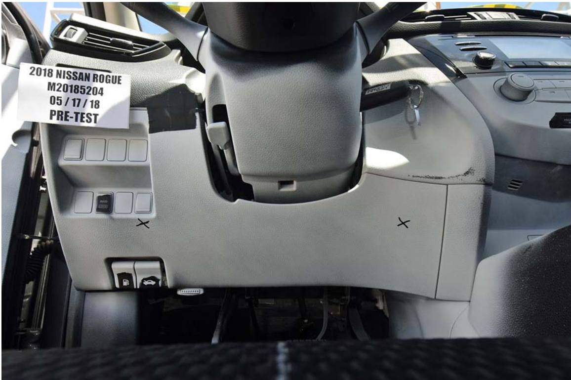
FIGURE 42. Pre-Test Driver's Side Knee Bolster
