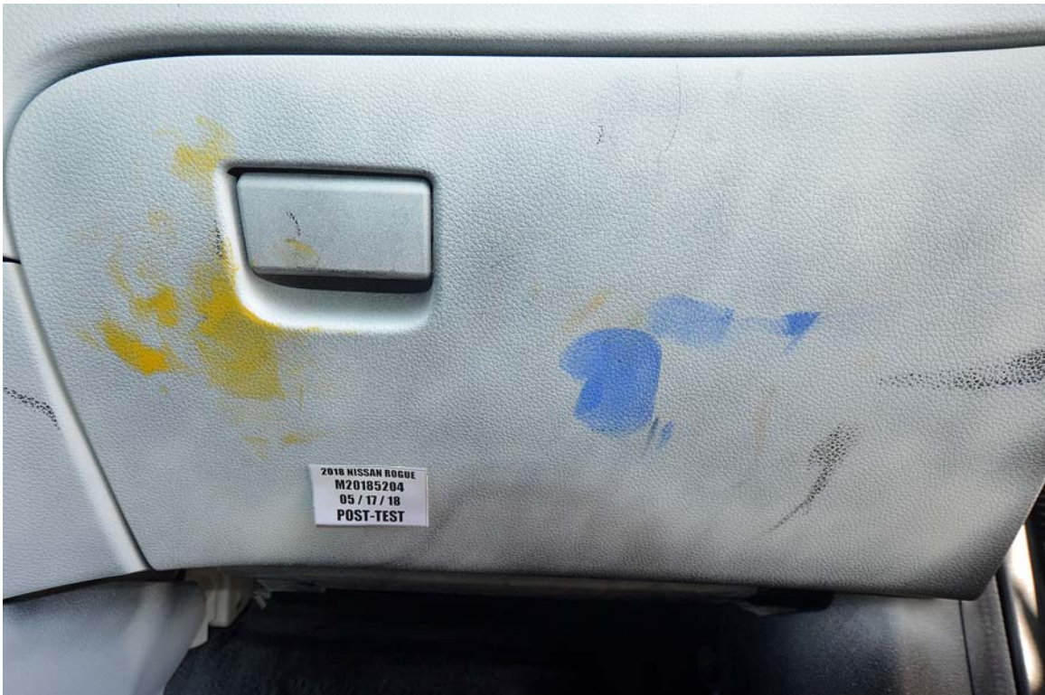
FIGURE 69a. Post-Test Passenger Dummy Contact with Knee Bolster
