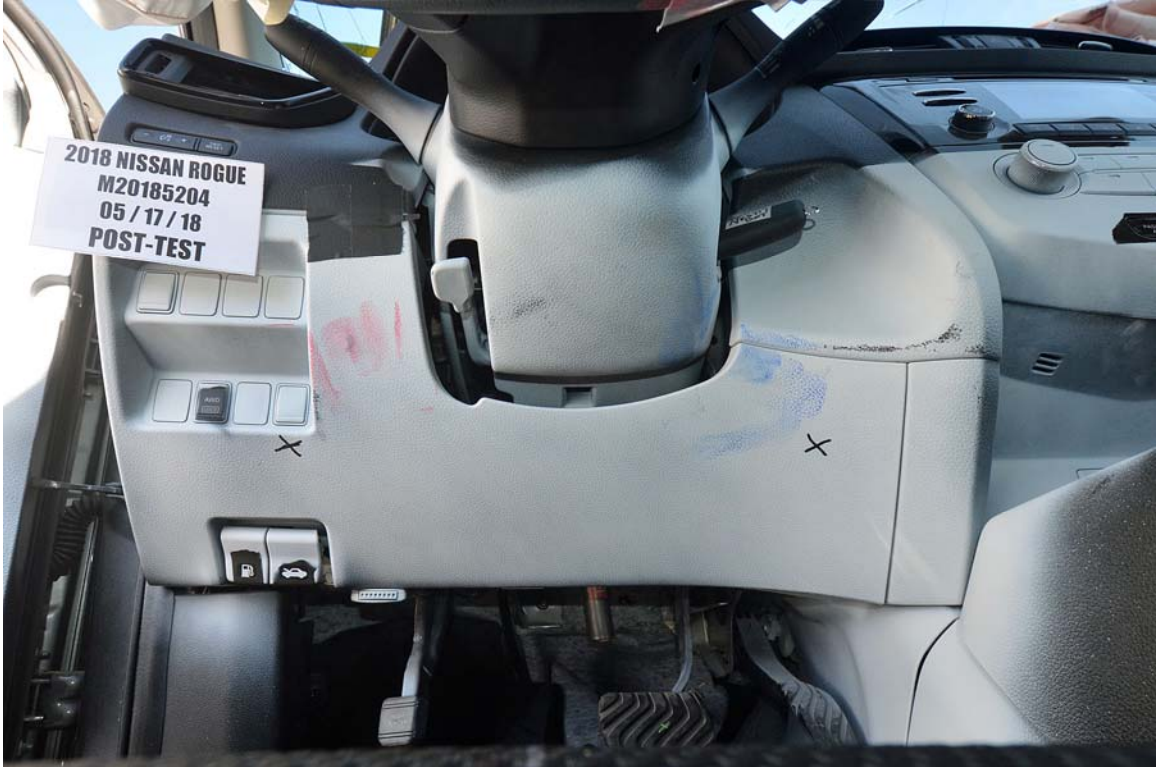
FIGURE 43. Post-Test Driver's Side Knee Bolster
