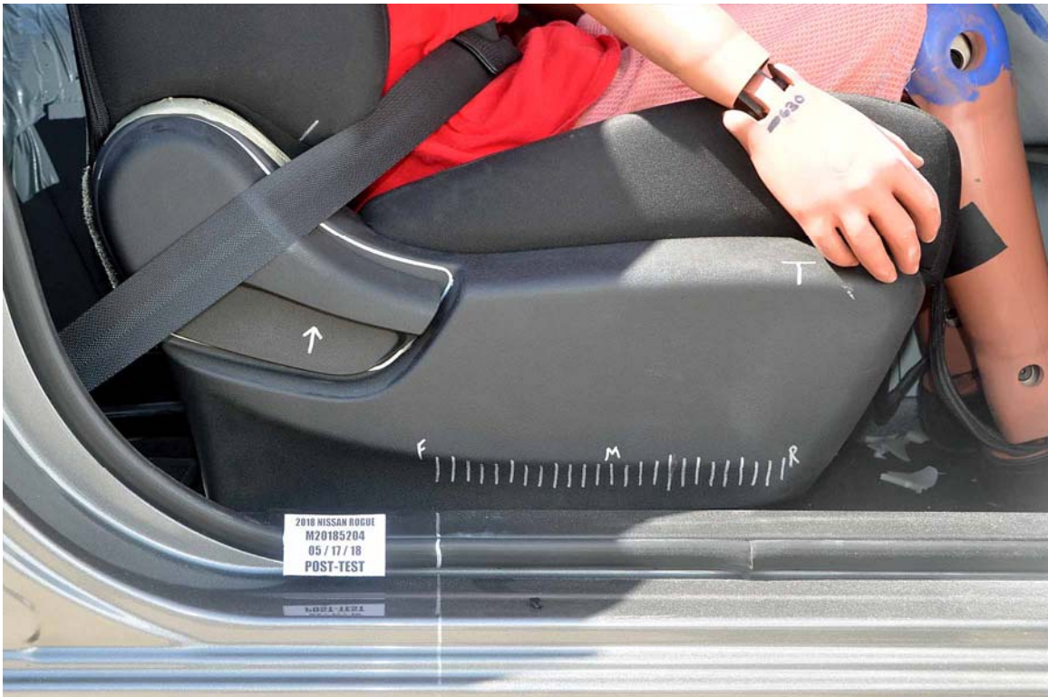
FIGURE 58. Post-Test Passenger's Seat Fore-Aft Markings
