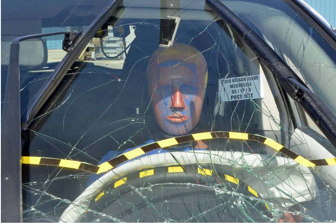
FIGURE 31. Post-Test Driver Dummy Front View
