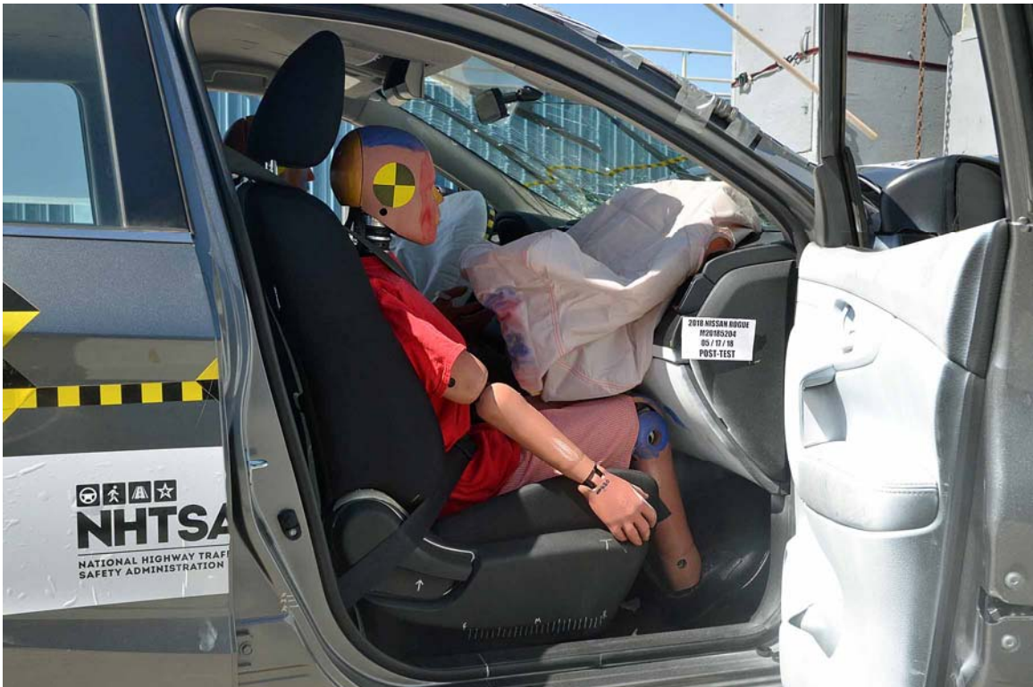
FIGURE 56. Post-Test Passenger Dummy and Vehicle Interior View
