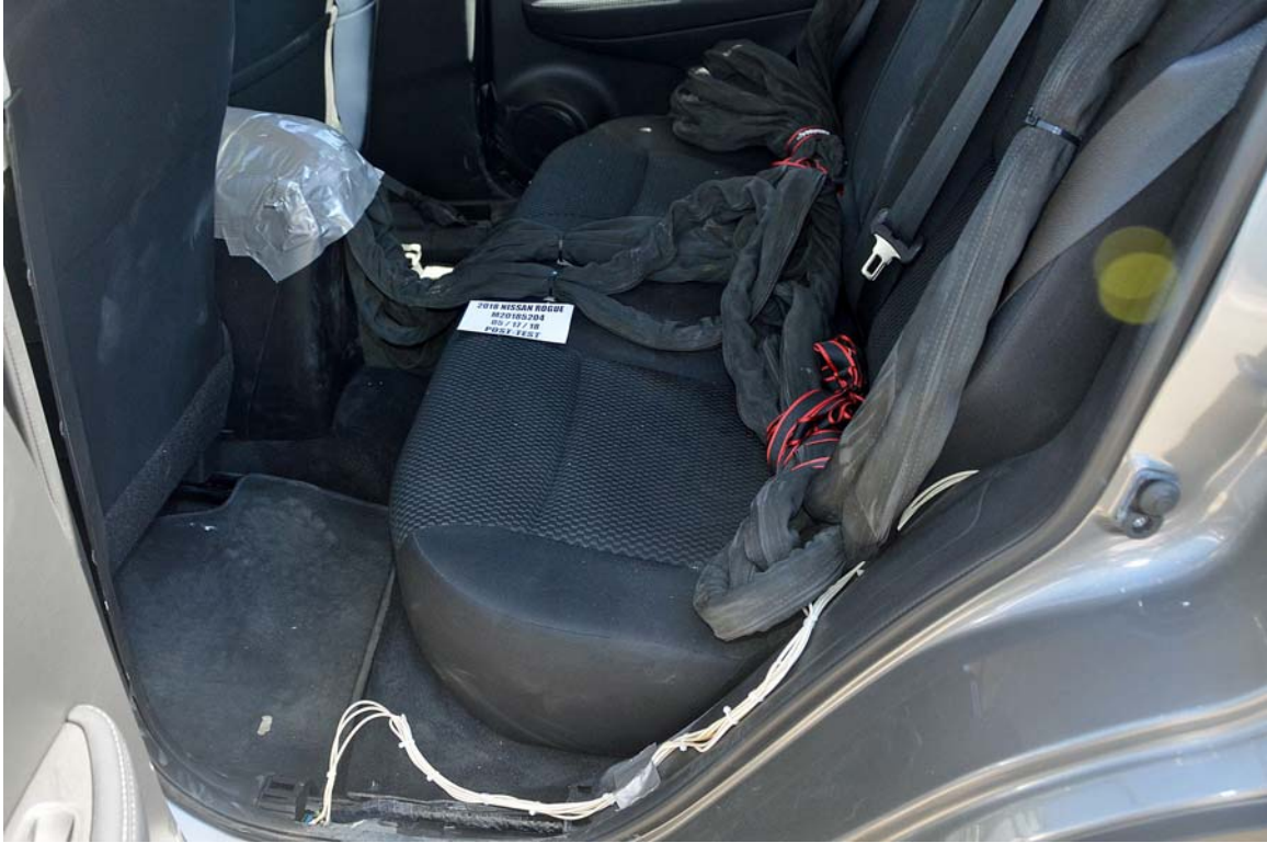
FIGURE 29. Post-Test Dummy Cable Routing
