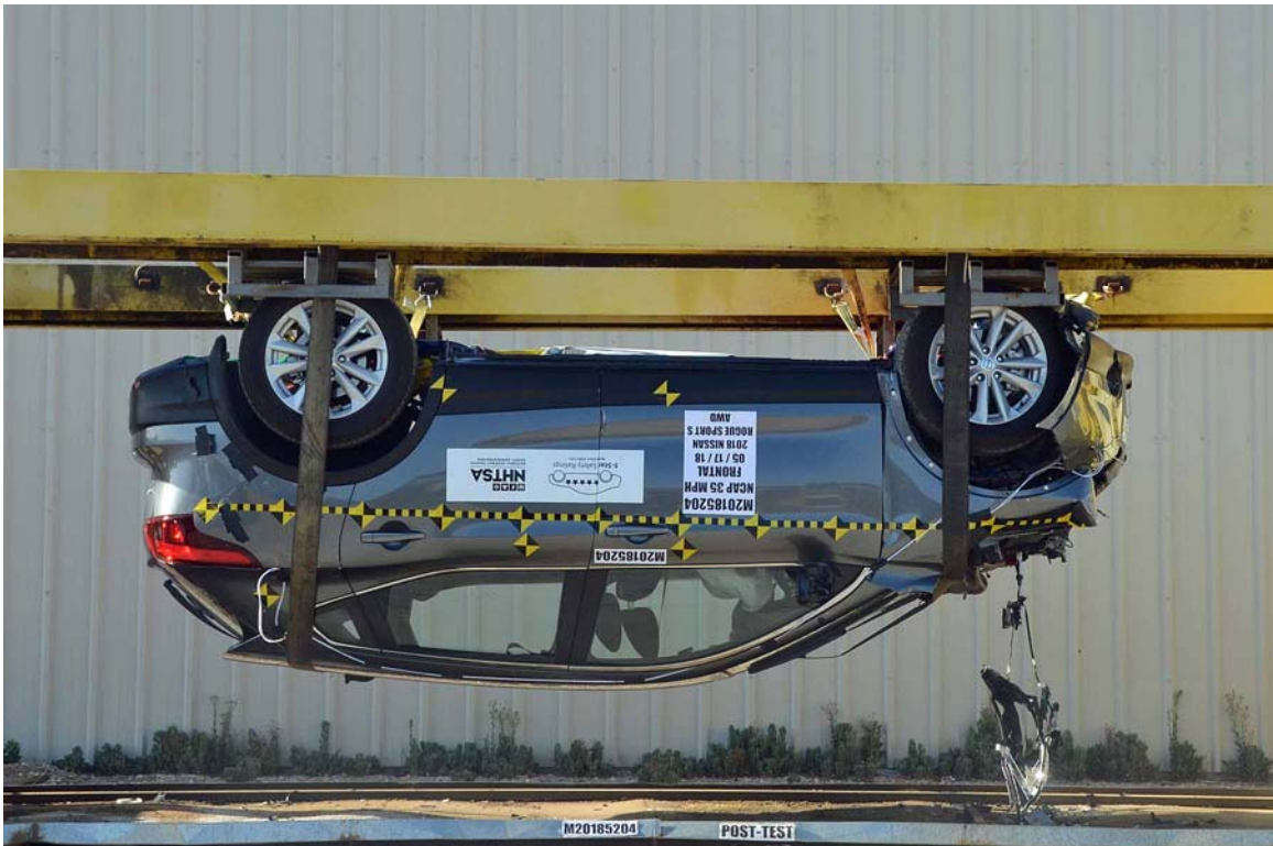
FIGURE 75. Vehicle at 180° on Static Rollover Device
