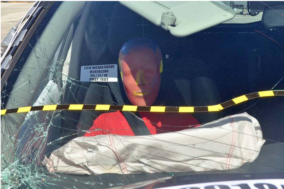
FIGURE 52. Post-Test Passenger Dummy Front View
