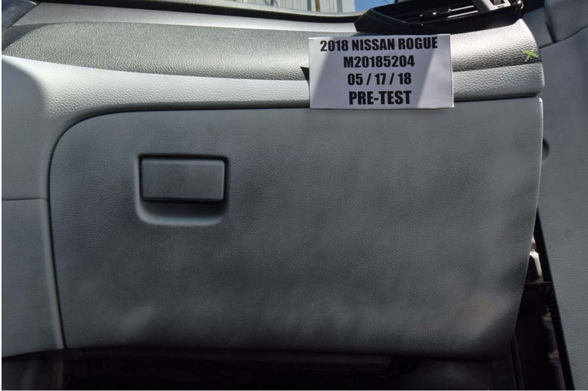
FIGURE 63. Pre-Test Passenger's Side Knee Bolster
