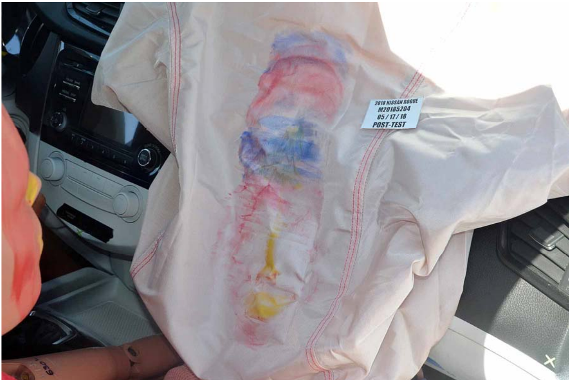
FIGURE 68. Post-Test Passenger Dummy Contact with Airbag
