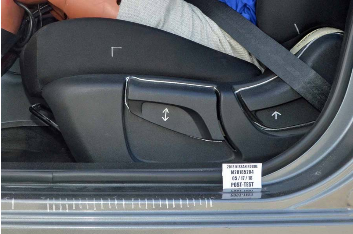
FIGURE 37. Post-Test Driver's Seat Fore-Aft Markings
