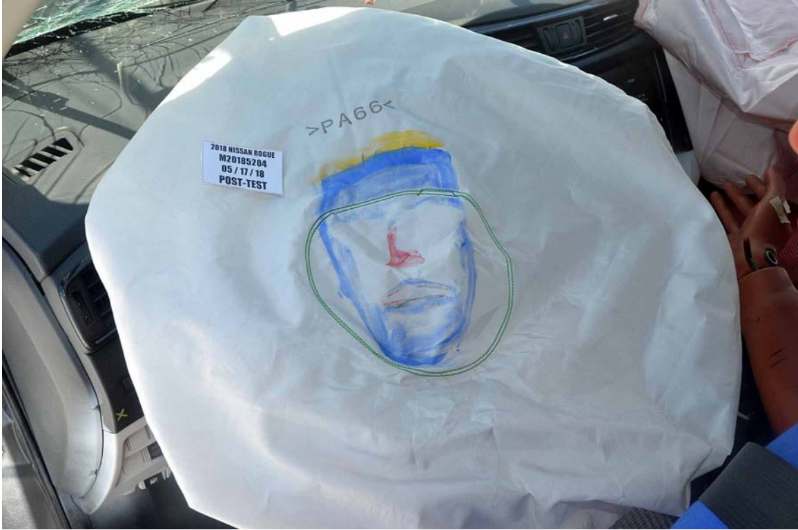
FIGURE 47. Post-Test Driver Dummy Contact with Airbag
