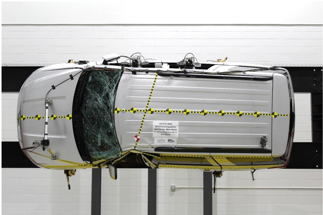
Figure A-64: FMVSS No. 301 Static Rollover 90 Degrees
