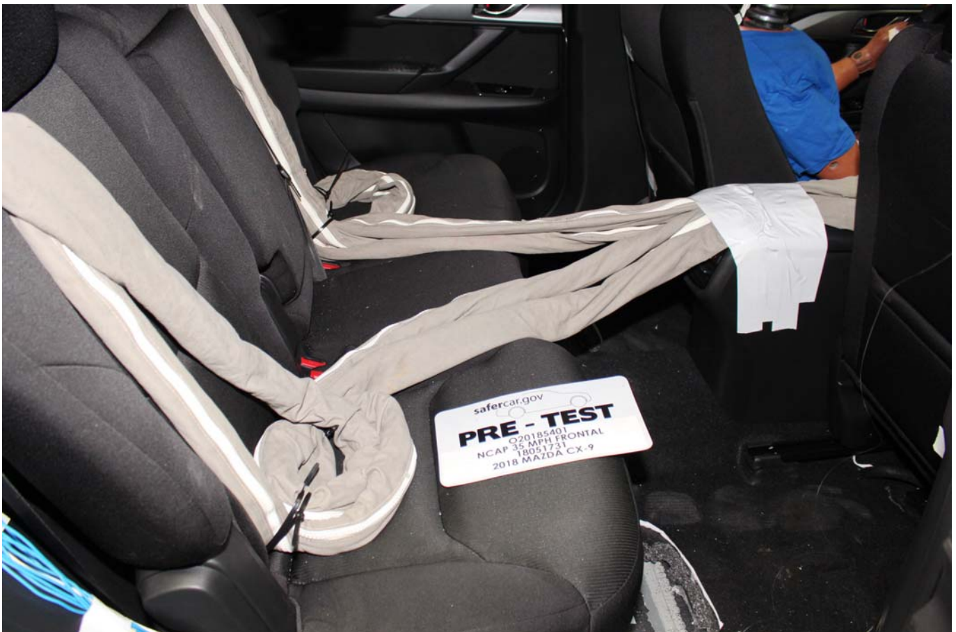
Photo No. 028 - Pre-Test Dummy Cable Routing
