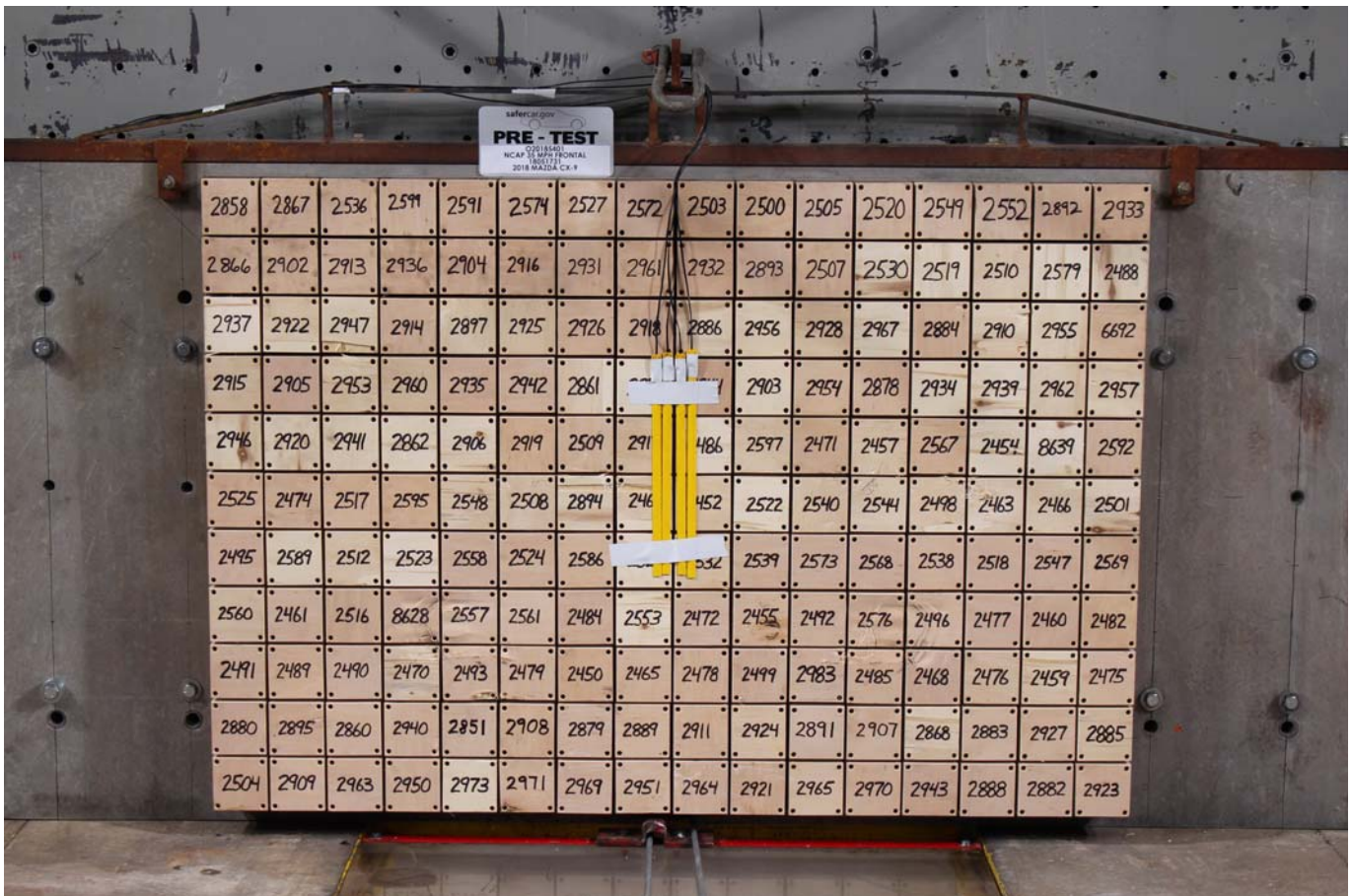
Photo No. 002 - Pre-Test Load Cell Wall
