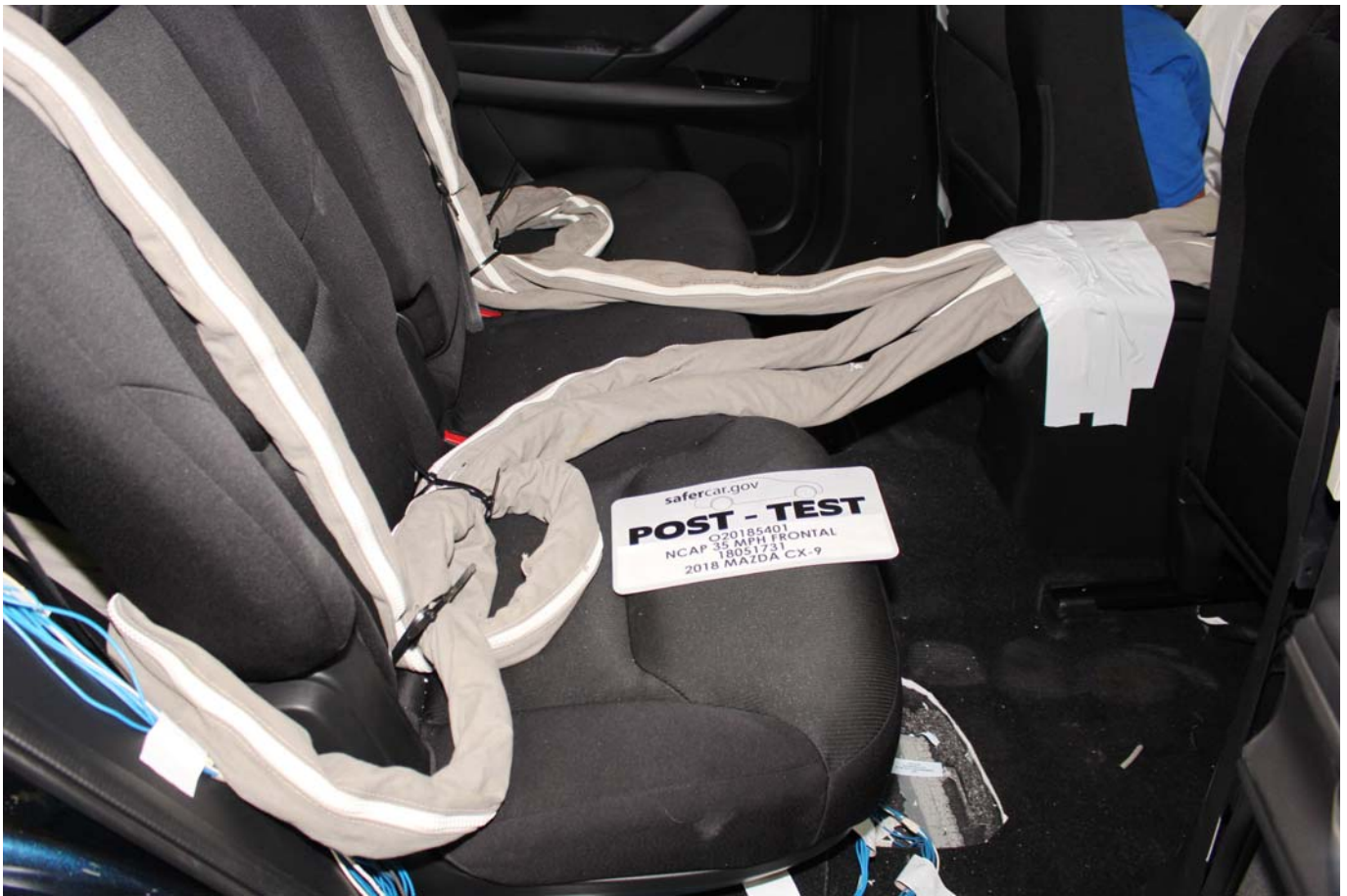
Photo No. 029 - Post-Test Dummy Cable Routing
