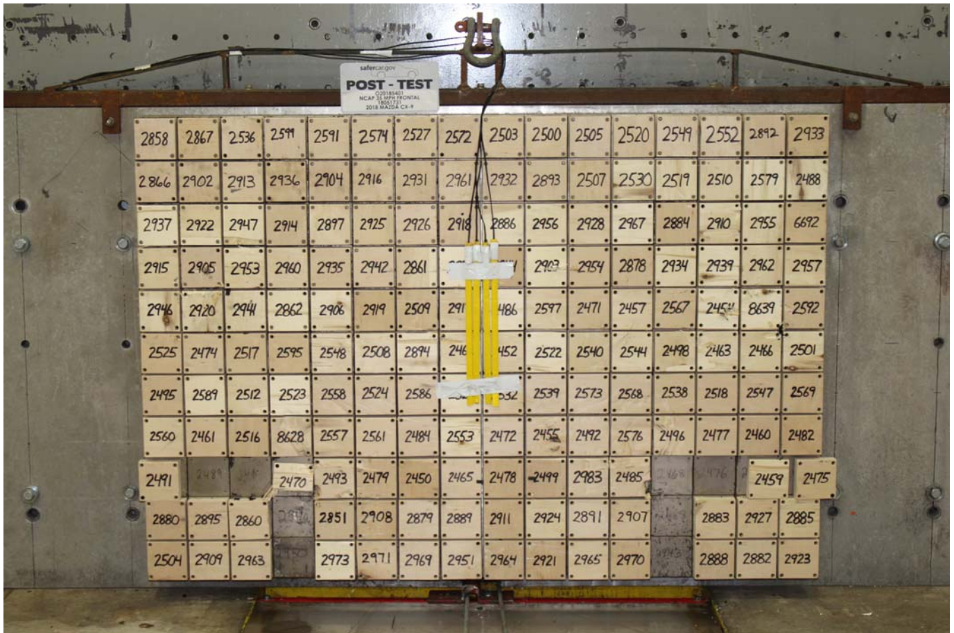
Photo No. 003 - Post-Test Load Cell Wall
