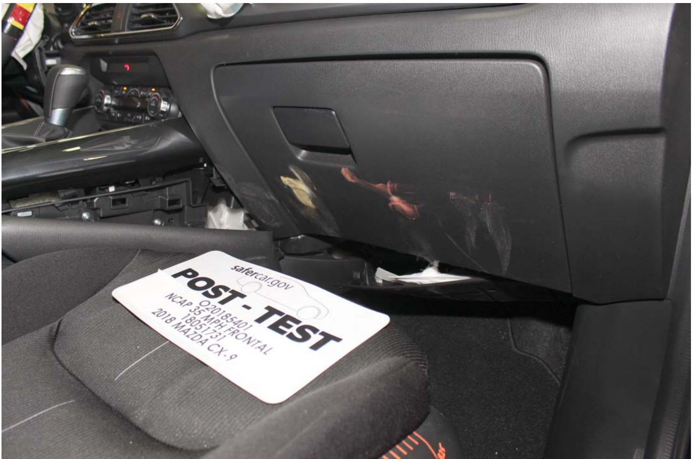
Photo No. 064 - Post-Test Passenger Side Knee Bolster (without dummy)
