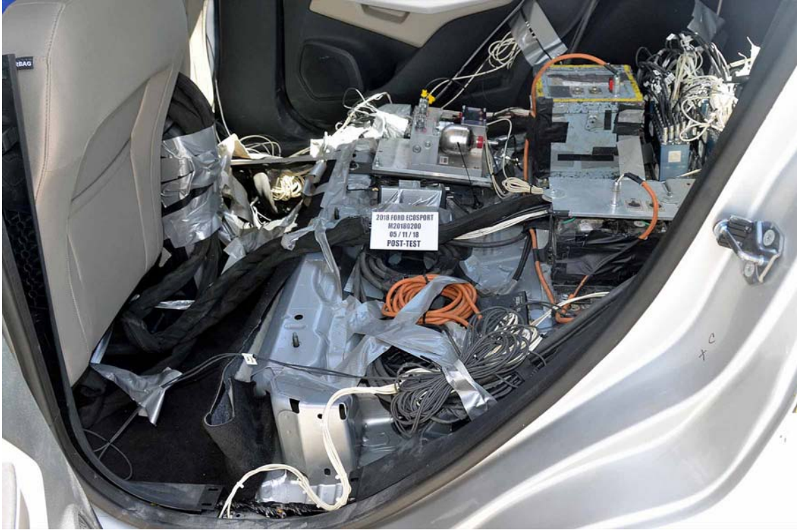
FIGURE 29. Post-Test Dummy Cable Routing
