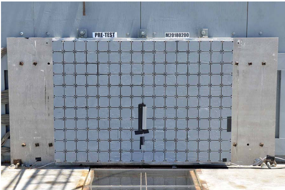
FIGURE 2. Pre-Test Load Cell Wall
