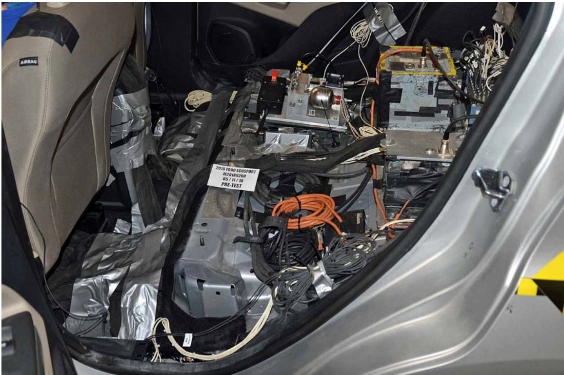
FIGURE 28. Pre-Test Dummy Cable Routing
