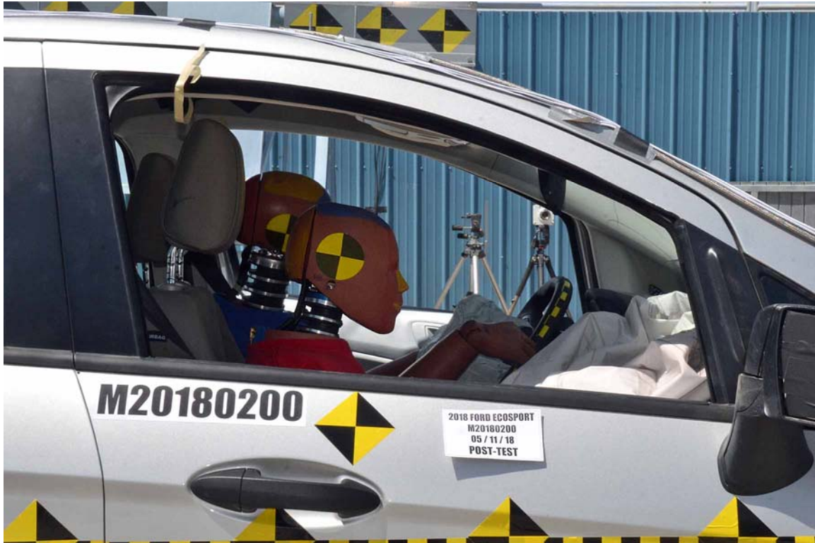
FIGURE 54. Post-Test Passenger Dummy Window View
