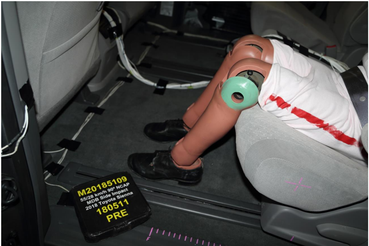
064 Pre-Test Placement of Rear Passenger Dummy's Feet
