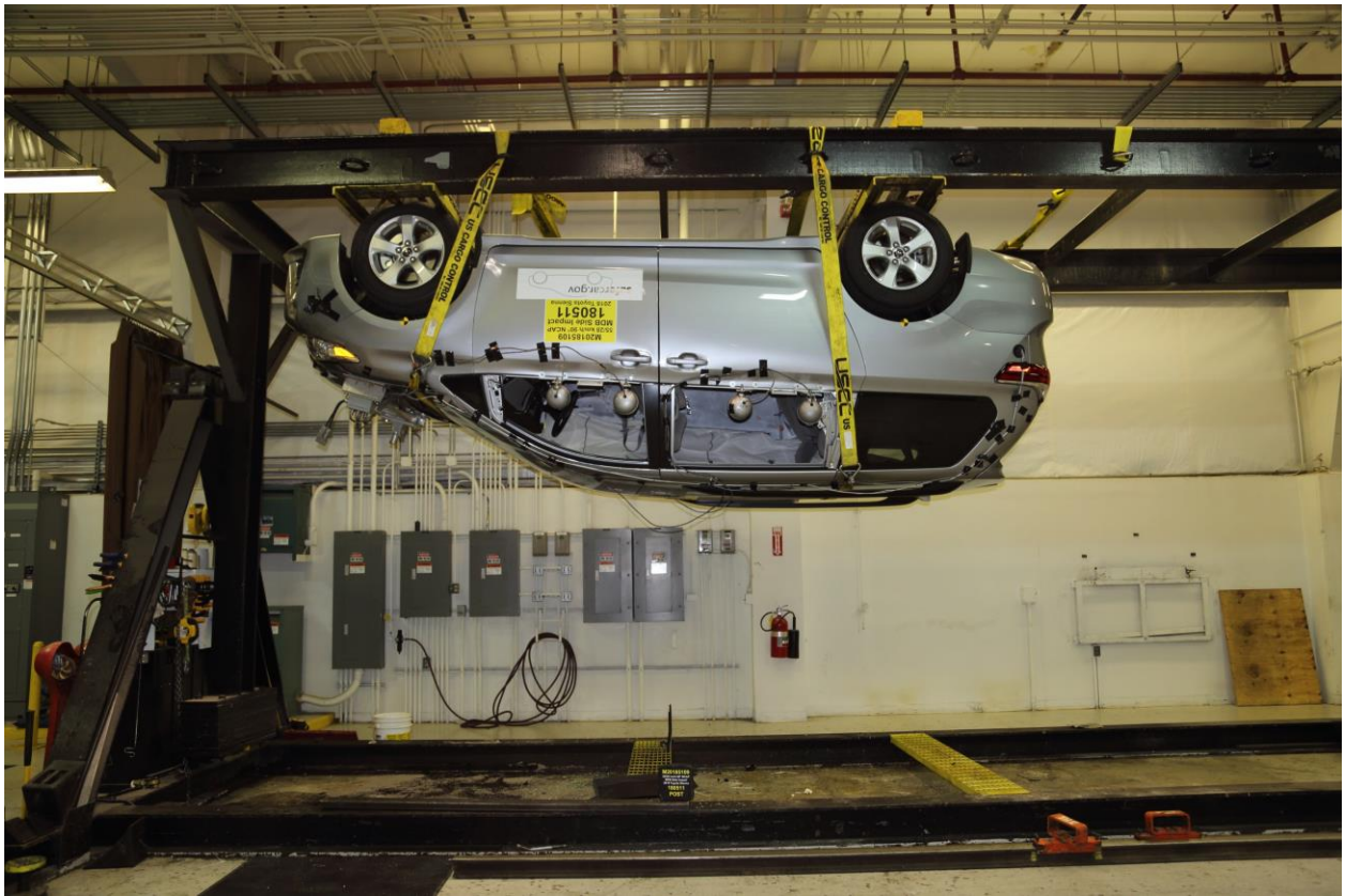
098 FMVSS No. 301 Static Rollover 180 Degrees
