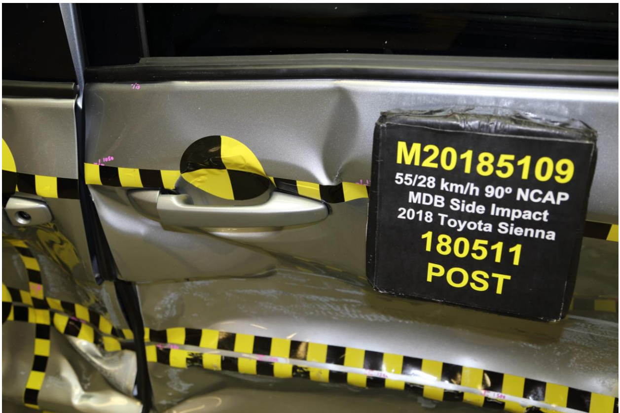
024 Post-Test Left Rear Door Latch Close-Up
