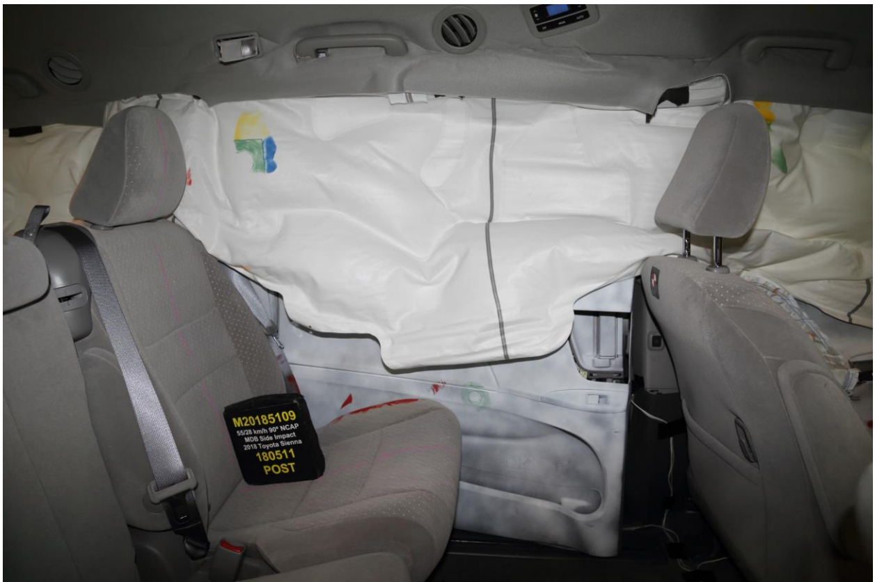
074 Post-Test Rear Passenger Inner Door Panel View
