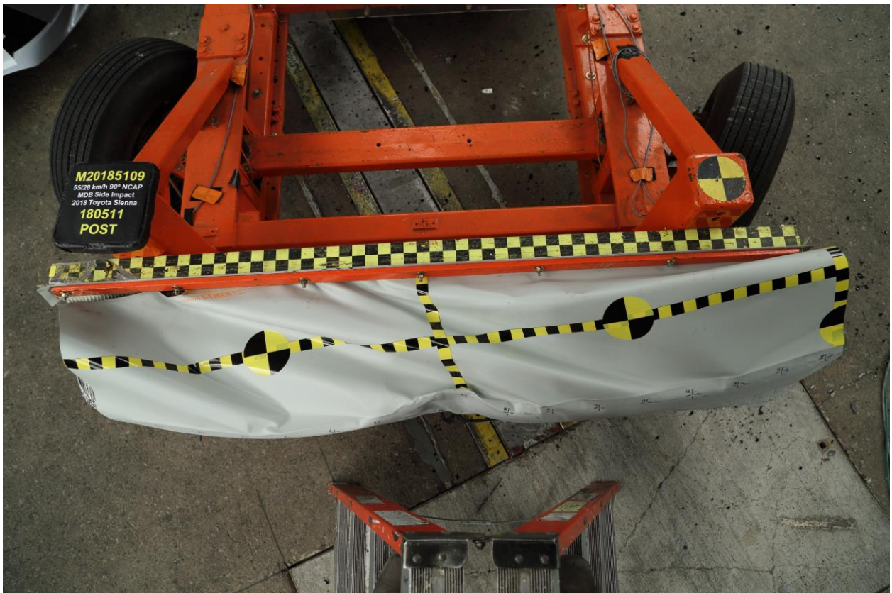
087 Post-Test Top View of MDB Impactor Face
