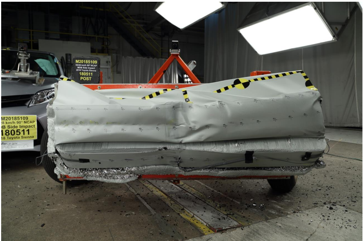
085 Post-Test Front View of MDB Impactor Face
