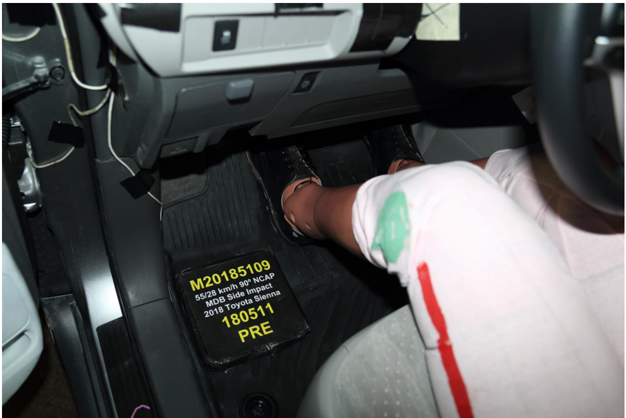
034 Pre-Test Placement of Driver's Dummy Feet
