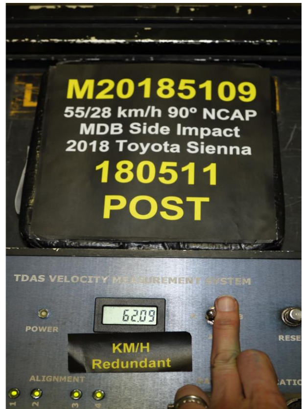
095 No. Post-Test Primary and Redundant Speed Trap Read-Out
