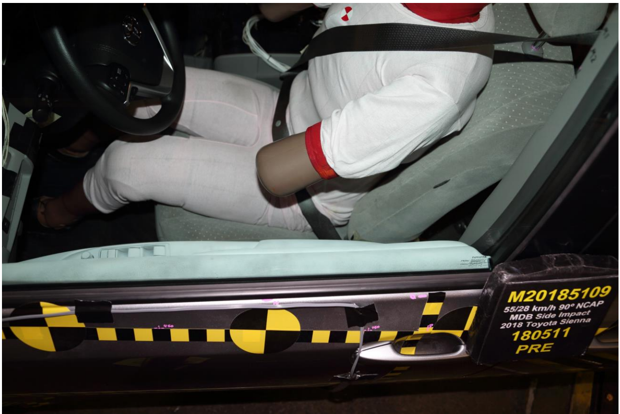
042 Pre-Test Driver Dummy and Door Clearance View
