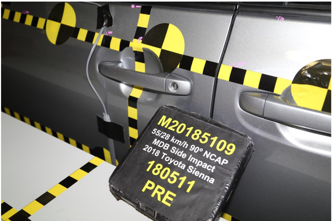
021 Pre-Test Left Front Door Latch Close-Up
