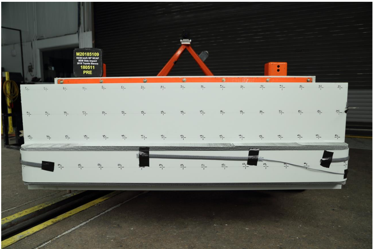
084 Pre-Test Front View of MDB Impactor Face
