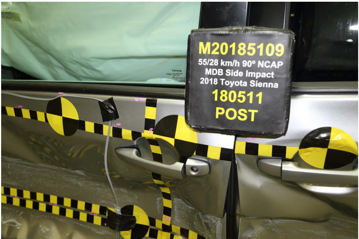
022 Post-Test Left Front Door Latch Close-Up
