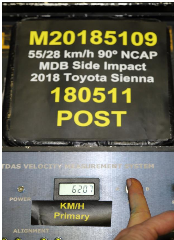
095 No. Post-Test Primary and Redundant Speed Trap Read-Out
