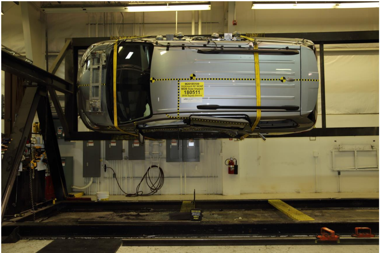
097 FMVSS No. 301 Static Rollover 90 Degrees
