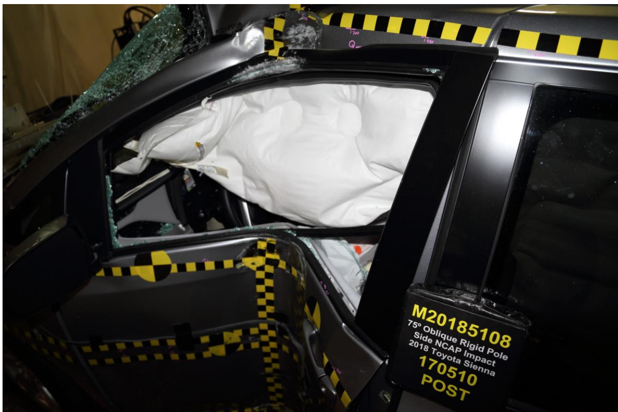
No. 041 Post-Test Dummy and Door Clearance View
