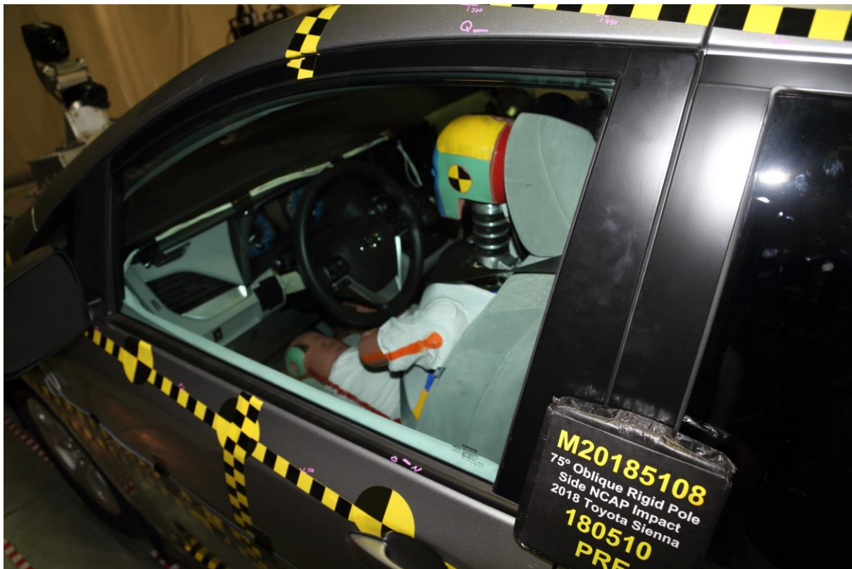
No. 040 Pre-Test Dummy and Door Clearance View
