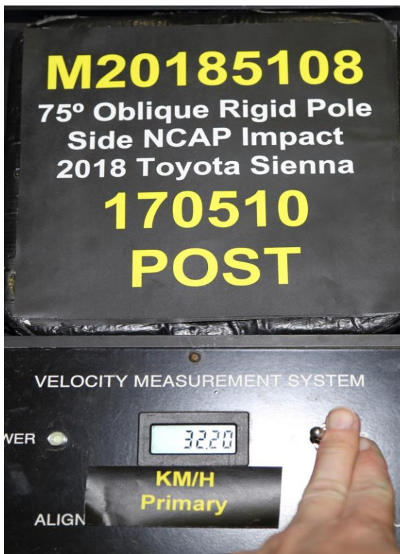
No. 062 Post-Test Primary and Redundant Speed Trap Read Out
