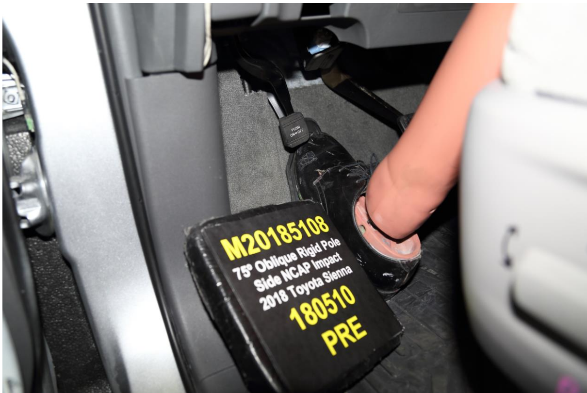
No. 032 Pre-Test Placement of Dummy Feet
