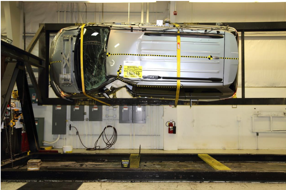
No. 064 FMVSS No. 301 Static Rollover 90 Degrees
