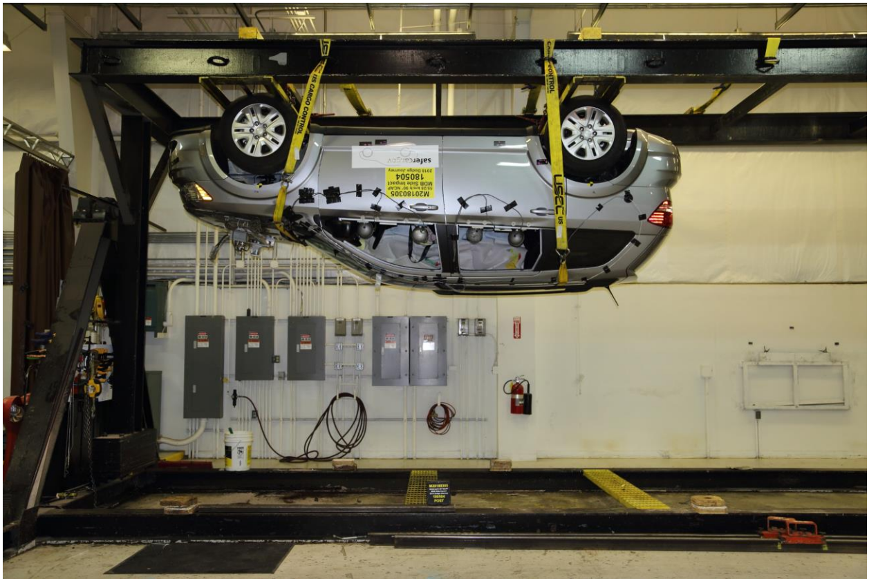
098 FMVSS No. 301 Static Rollover 180 Degrees
