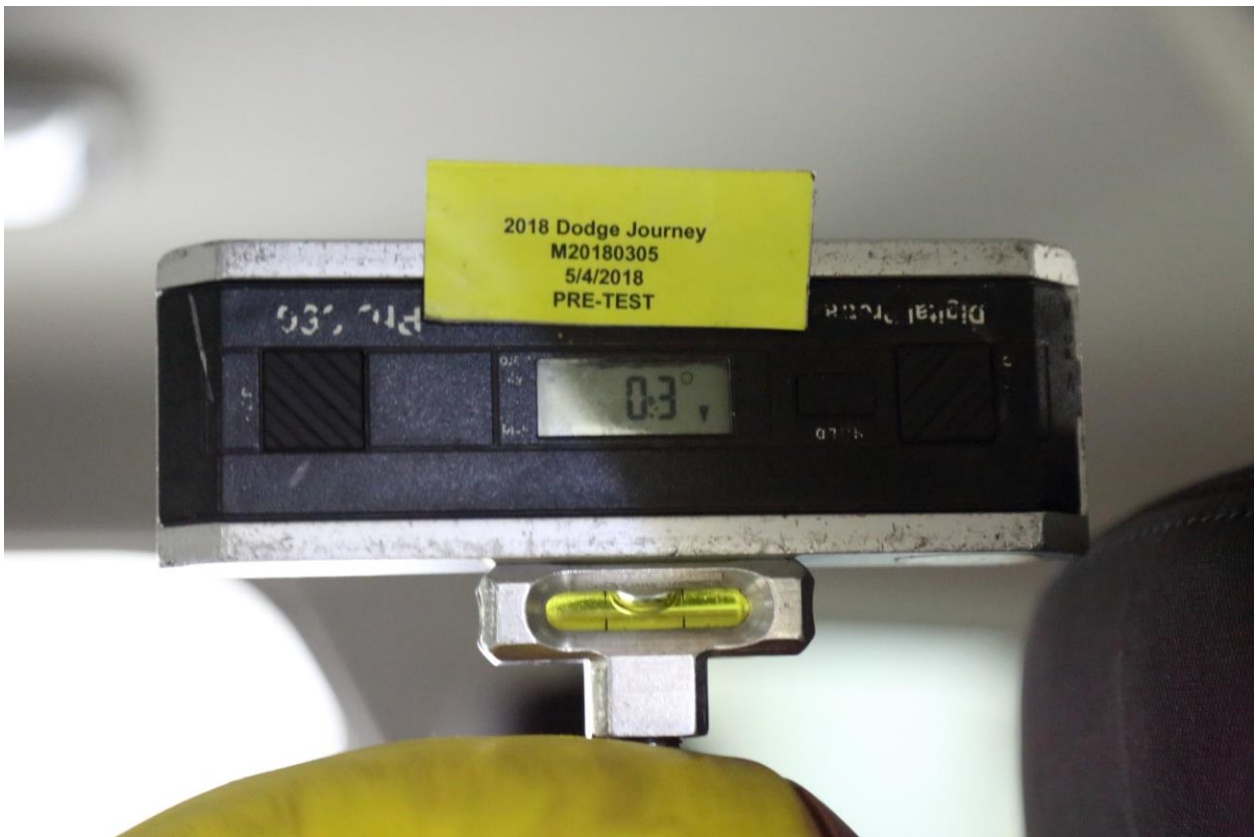
063 Pre-Test View of Rear Passenger Dummy's Head Showing Dummy Head is Level
