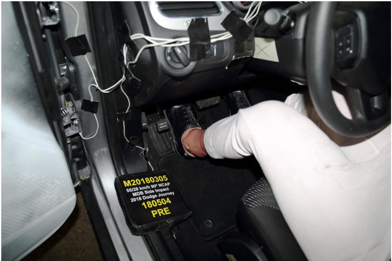
034 Pre-Test Placement of Driver's Dummy Feet
