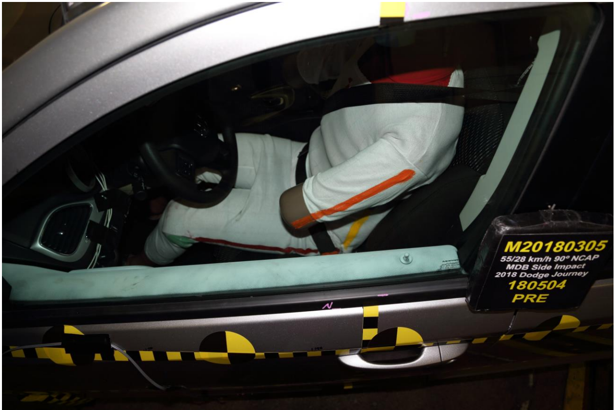
042 Pre-Test Driver Dummy and Door Clearance View
