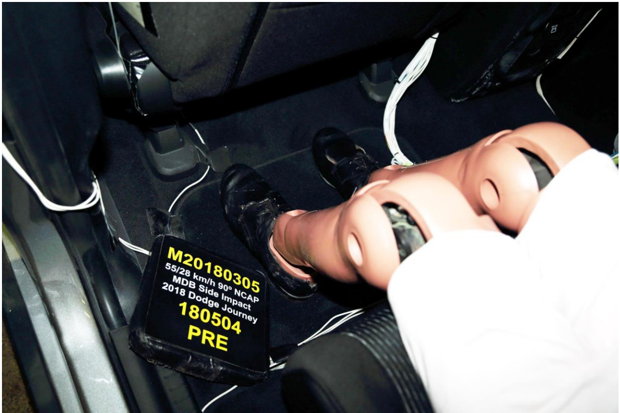
064 Pre-Test Placement of Rear Passenger Dummy's Feet
