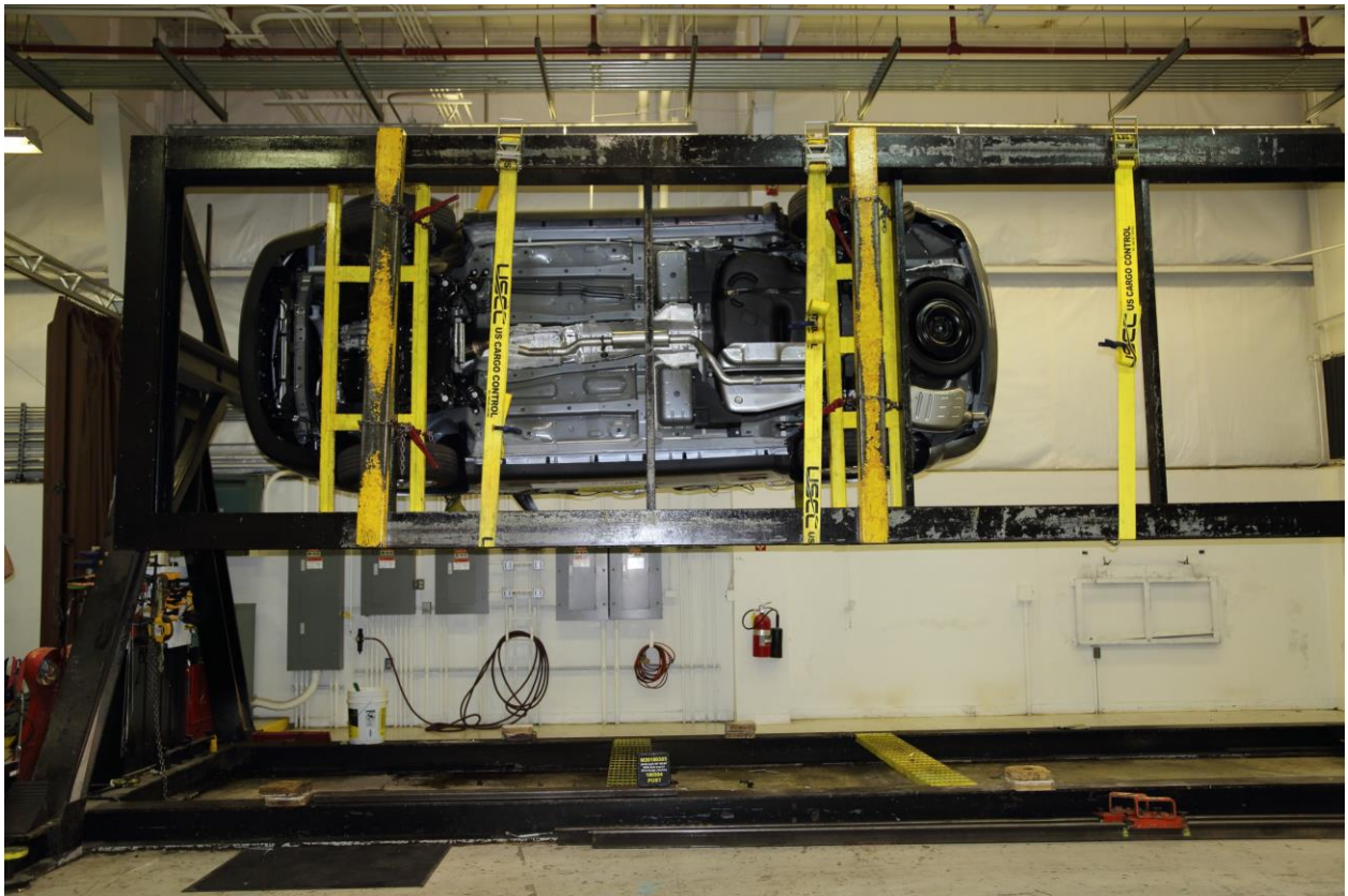
099 FMVSS No. 301 Static Rollover 270 Degrees
