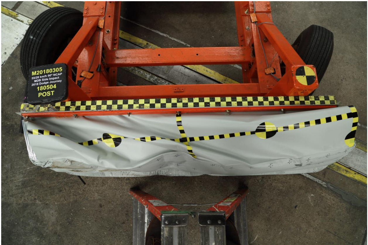
087 Post-Test Top View of MDB Impactor Face
