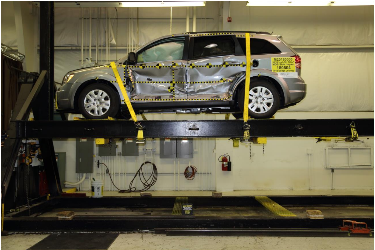
096 FMVSS No. 301 Static Rollover 0 Degrees
