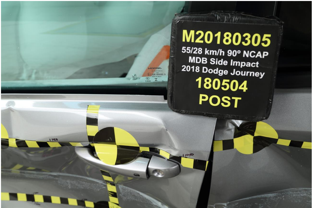
022 Post-Test Left Front Door Latch Close-Up
