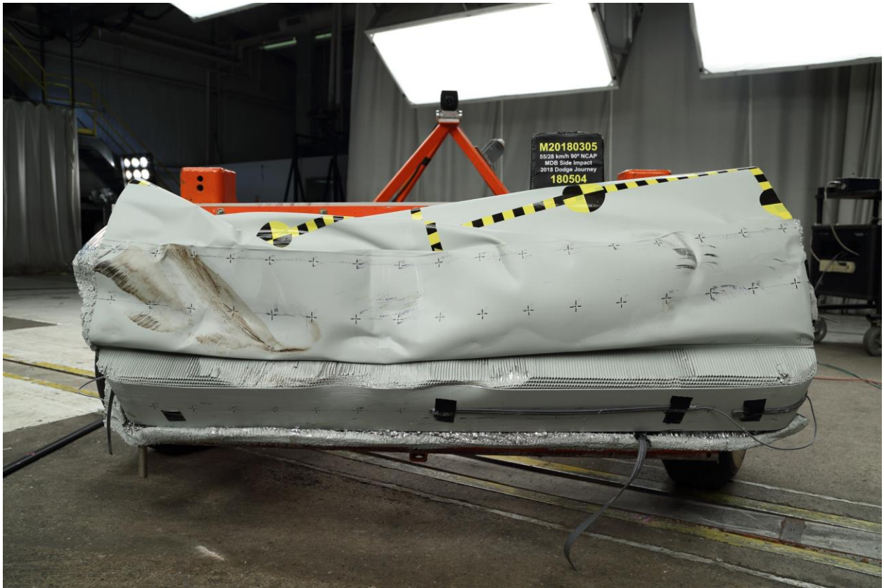
085 Post-Test Front View of MDB Impactor Face
