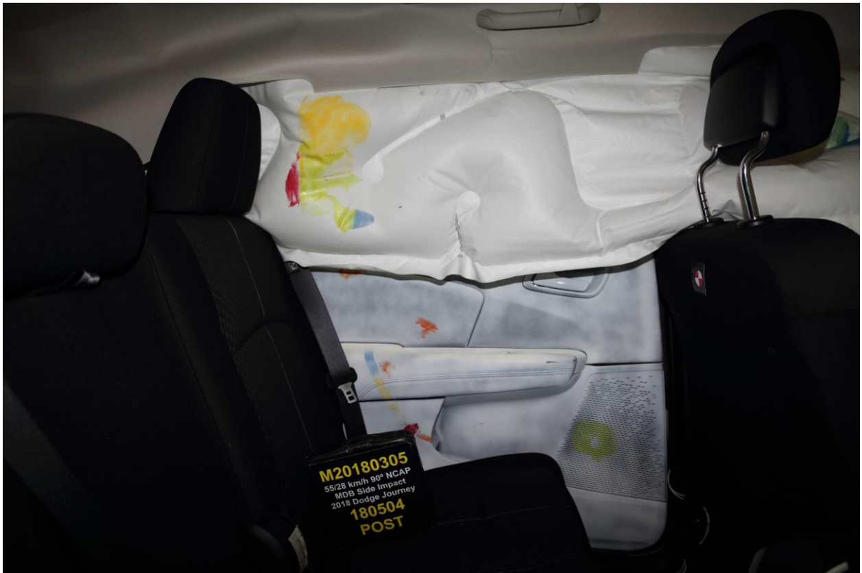
074 Post-Test Rear Passenger Inner Door Panel View
