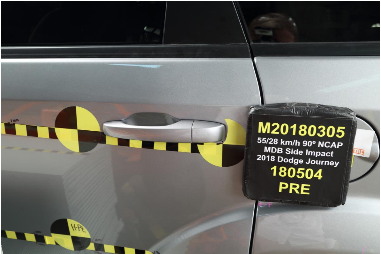
023 Pre-Test Left Rear Door Latch Close-Up
